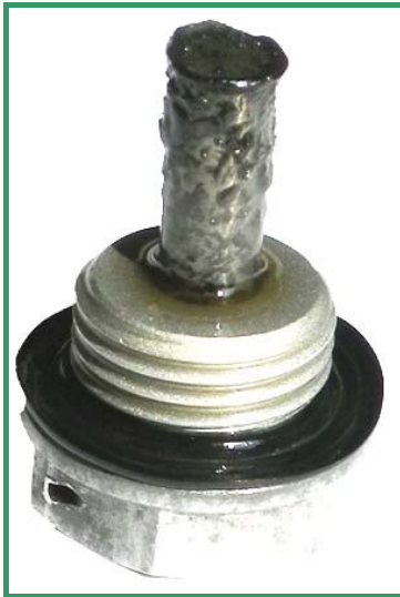
Fig. 85 - 11 Accumulation of allowable debris
