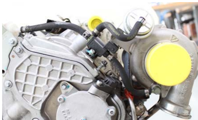
Fig. 81 - 3 Previous BPA installation version
