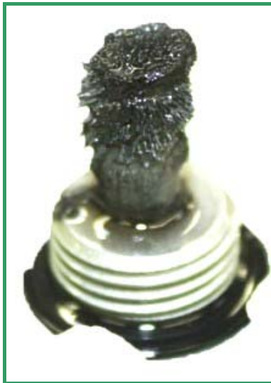
Fig. 85 - 10 Acceptable quantity for first 100 h inspection
