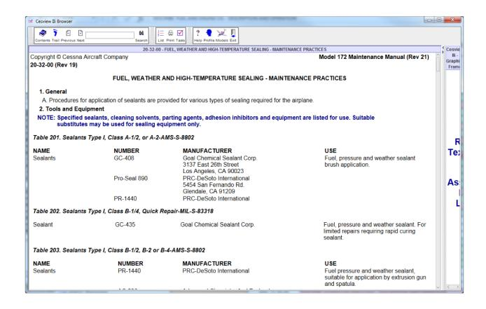
Section 20-32-00 of the maintenance manual provides procedures for application of sealants for various types of sealing required for the airplane.
