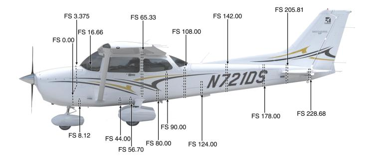
The airplane is laid out according to fuselage stations (FS) and wing stations (WS). These stations provide fixed reference points for all components located on or within the airplane. Fuselage Stations begin at the firewall (FS 0.00) and extend to the tail cone area (FS 230.18). Wing Stations begin at the root (WS 23.62) and extend to the tip (WS 208.00). Both Fuselage Stations and Wing Stations are measured in inches. For example, FS 185.50 is 185.50 inches aft of the firewall (FS 0.00).
