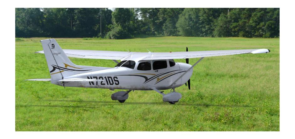
Wash the airplane frequently in order to maintain its appearance and minimize corrosion. Polish the painted area of the airplane at periodic intervals to remove chalking paint and restore its gloss. Water/detergent cleaning is the preferred method to clean the exterior surface of the airplane.
