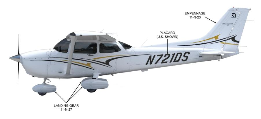
Examine the interior of the airplane. Include the aft baggage areas for the installation of all required placards, decals, and markings. For required placards, decals, and markings, refer to the Model 172S Illustrated Parts Catalog.
