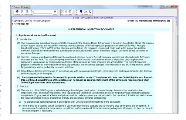
The function of the SID Program is to find damage from fatigue, overload or corrosion through the use of the Nondestructive Inspections (NDI) and visual inspections. The SID is only for primary and secondary airframe components. Engine, electrical items and primary and secondary systems are not included in this document.
