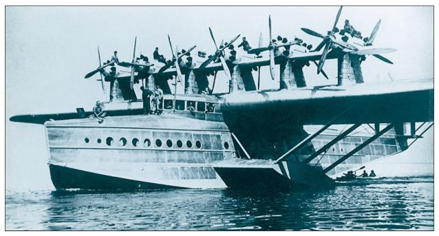
The Do X in its original form, with Jupiter radial engines. Although it flew successfully with this powerplant, it was underpowered for regular operations.
