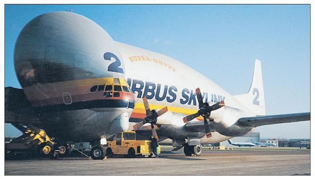
With its vast forward fuselage hinged to port, a Guppy 201 takes on a load of Airbus components.
