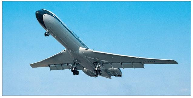
The VC10's extensive high-lift devices were particularly evident on take-off.
