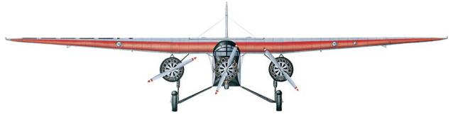
Ford Model 5-AT-B, a variant of the TriMotor, featuring three 313kW (420hp) engines and seating for 15 passengers. Forty-two were built.
