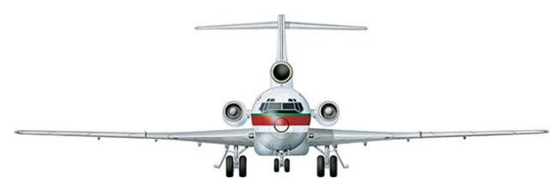
In another masterstroke Boeing used the upper fuselage of the 707, speeding design, standardizing flight decks and saving money on production tooling. The relatively wide cabin also allowed the 727 to seat passengers six abreast in
