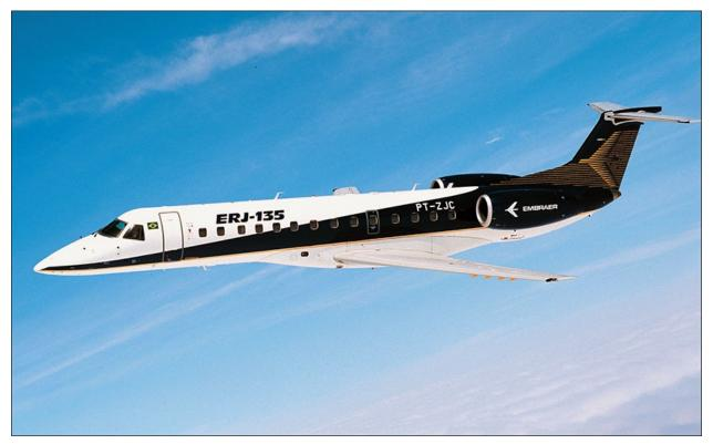
**PT-ZJC** was the second ERJ-135 prototype. The model's forward fuselage was shortened compared to that of the ERJ145.
