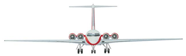
The VC10's engine nacelles were mounted in a 'spectacle' arrangement, but a short joining section separated those of the II-62.
