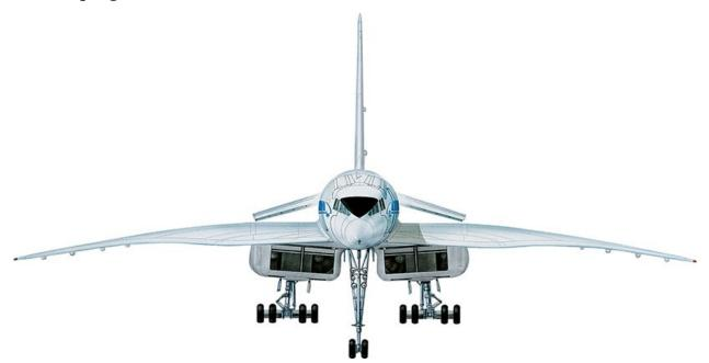
The Tu-144 prototype resembled Concorde, but was quite different in detail, while the production aircraft were far closer to the Western aircraft in design.
