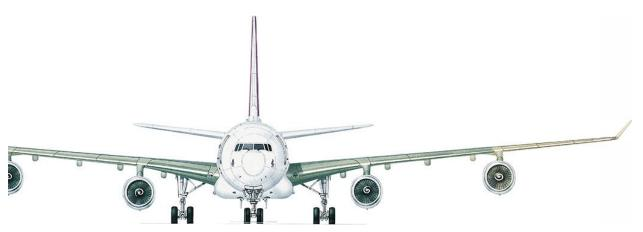
The wings of the A330 and A340 are remarkably similar, the A330 retaining the hardpoint for the outer engine's pylon.
