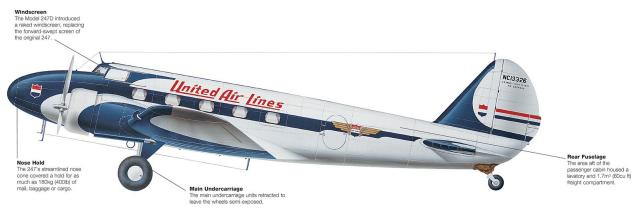
This United Air Lines Model 247D, NC13326, is shown in a typical late-1930s' United colour scheme.
