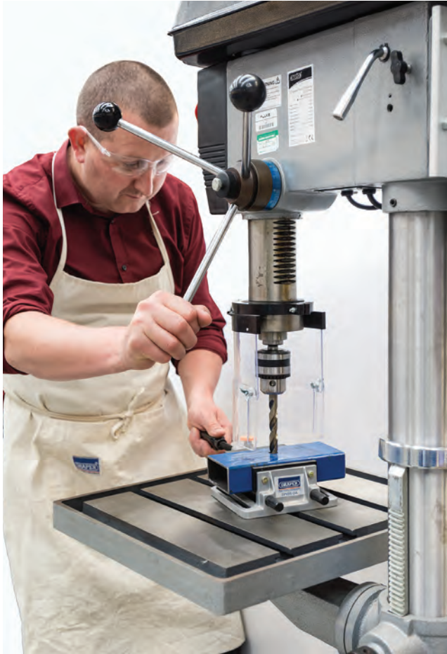
Figure 10.22 Typical pedestal drill – note the guard is adjustable and adjusted to cover the rotating drill
