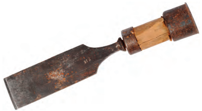
Figure 10.7 (a) Damaged wood chisel with dangerous handle.
