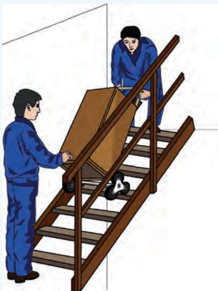
A sack truck with star truck wheels for climbing and descending stairs
