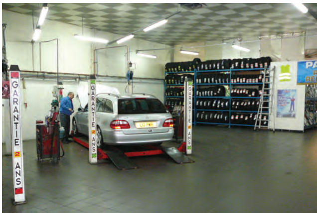
Figure 9.15 Hoist for lifting a car
