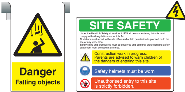
Figure 4.9 Falling object and construction site entrance signs
