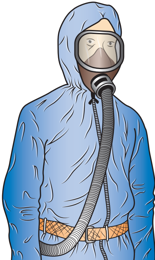
Figure 4.20 Respiratory protection and disposable overalls are needed when working in high levels of asbestos dust
