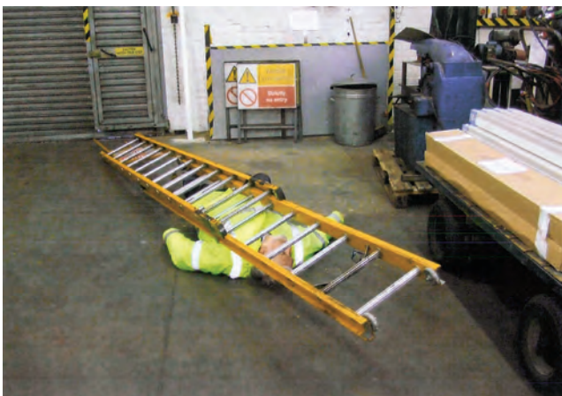
Figure 5.5 Accident at work – reconstruction of a ladder accident showing where the deceased person was found under the ladder which had toppled over while he was attempting to adjust the height of the extending ladder
