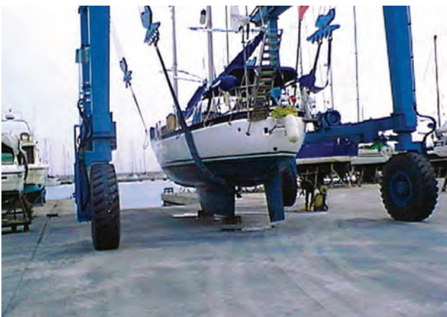
Figure 9.14 Manoeuvring a yacht using a large overhead travelling gantry and slings in a marina
