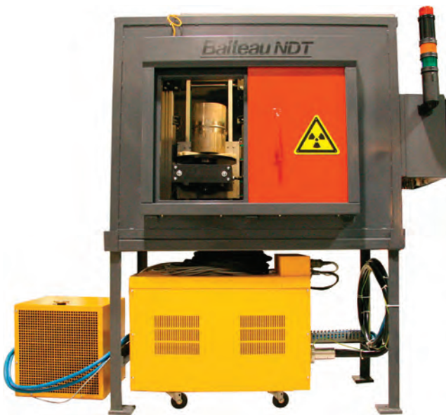
Figure 14.9 X-ray generator cabinet
