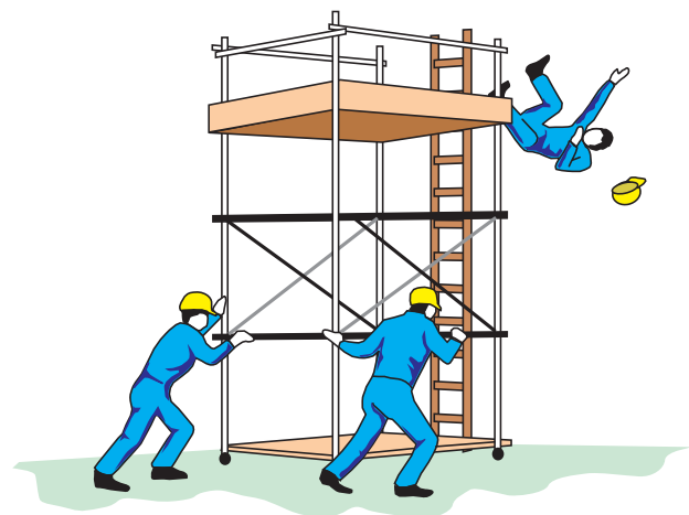
Figure 7.9 Falling from a height – tower scaffold has inadequate handrails (no centre rail) and should never be moved while in use
