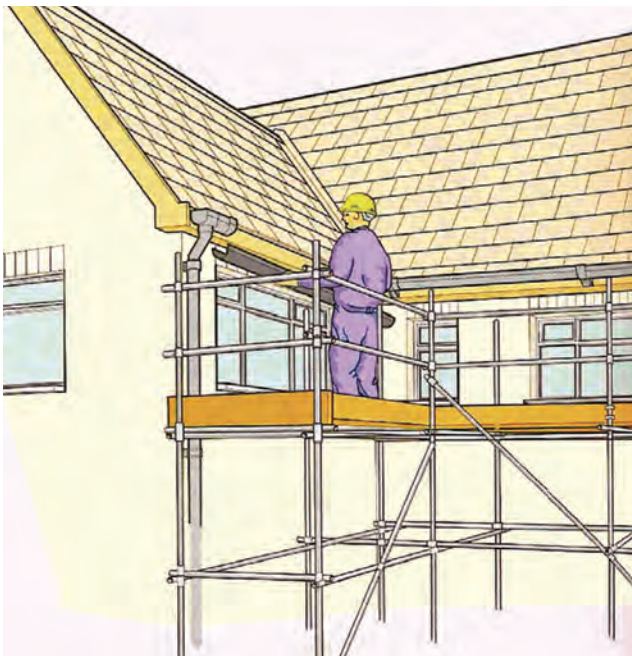
Figure 7.17 (a) Components of a typical independent tied scaffold; (b) fixed scaffold left in place to fit gutters
