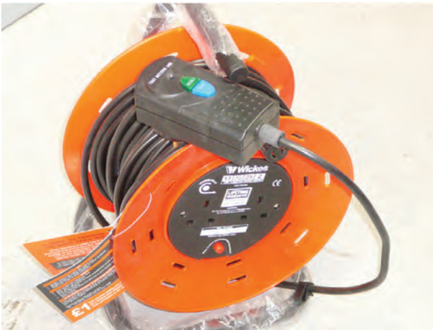
Figure 11.11 Multi-plug extension lead and special plugs and sockets: (a) reduced voltage normally 110V; (b) 240 volt lead with cut out
