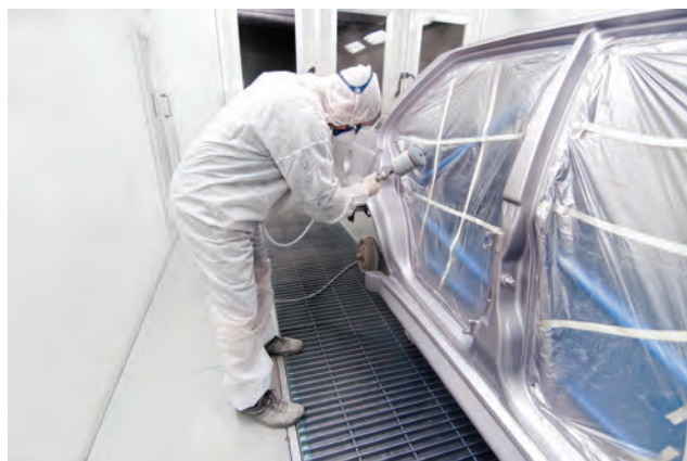
Figure 13.13(c) Paint-spraying inside a special room with general ventilation to remove fumes
