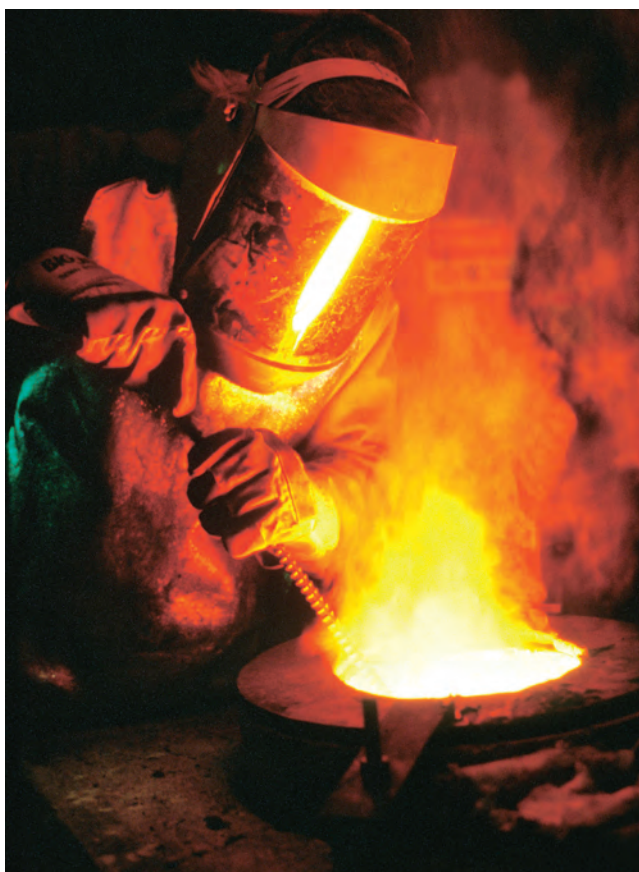
Figure 14.12 Metal furnace - source of infrared heat
