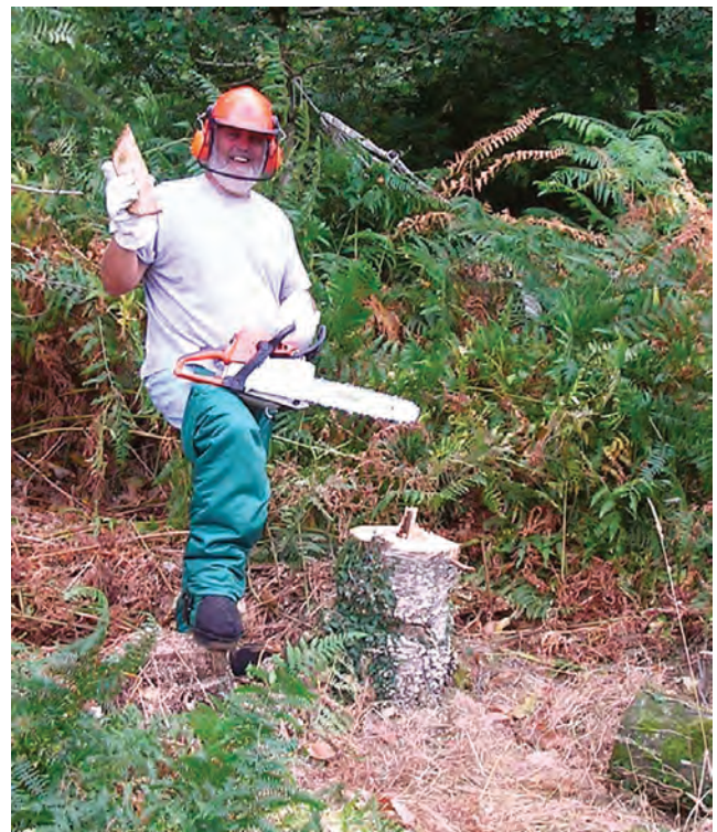
Figure 10.26 Kevlar gloves, overtrousers and overshoes providing protection against chainsaw cuts. Helmet, ear and face shield protect the head. Apprentice under training – first felling
