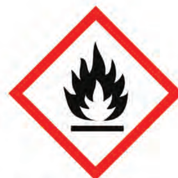
Danger Extremely Flammable Gas
