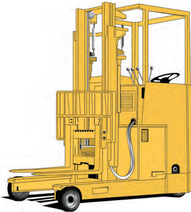
Figure 9.13 Reach truck, designed so that the load retracts within the wheel base to save space
