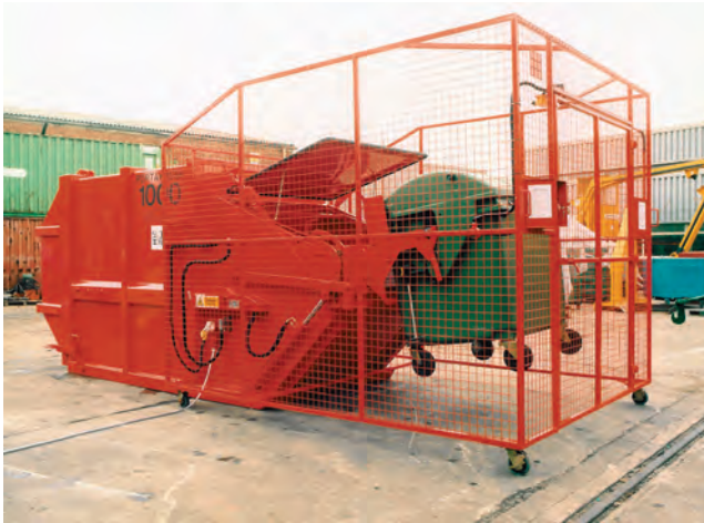
Figure 10.27 Typical retail compactor
