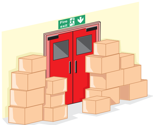
Figure 12.13 Partly blocked fire exit door
