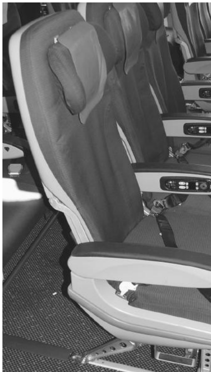
FIGURE 6.20 “This seat has a nice thin backrest at knee level, but the seat pan is somewhat short.”
