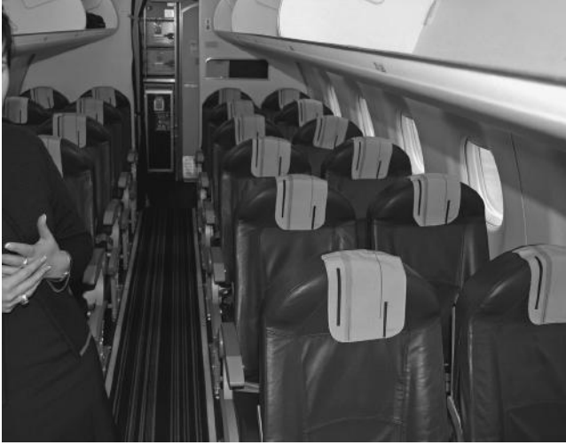
FIGURE 3.10 Some airplanes have two seats abreast, which has a positive effect on the comfort experience.
