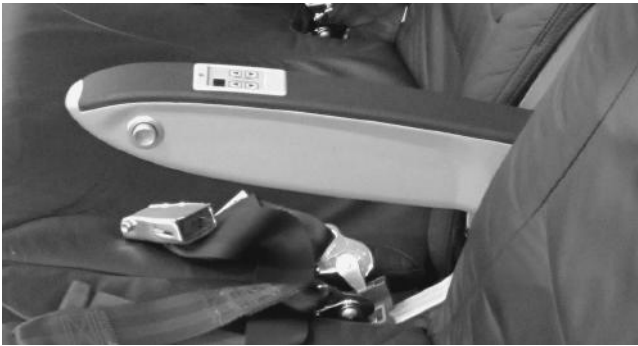
FIGURE 6.27 A passenger mentions that buttons on the top of the armrest are better, visible, and easy to touch compared with buttons on the inner side.
