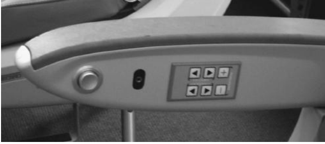
FIGURE 6.26 Compared with figure 6.27, a passenger mentions that this position is wrong as the buttons on the side make you step out of your seat to see and reach the buttons.
