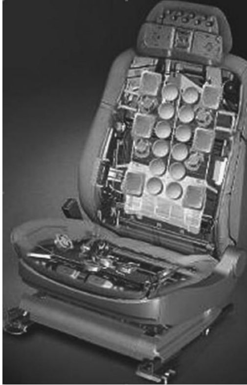
FIGURE 4.2 The BMW seat with the massage system of Franz (2010). The 12 round and 6 square elements are inflatable and generate the massage effect.
