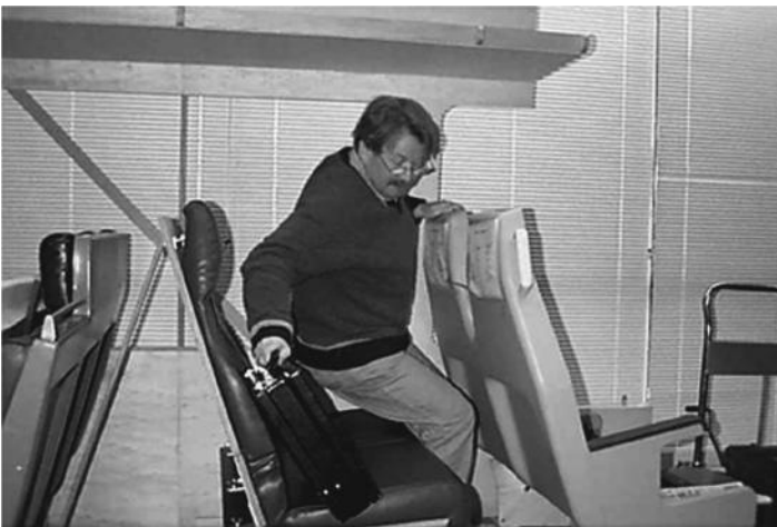
FIGURE 4.7 One of the experiments done with a mock-up to test the in- and egress for the railway seats.
