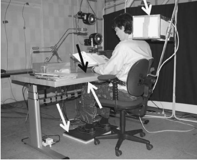
FIGURE 5.11 Studying the effect of local heating systems on comfort (Oeffelen et al., 2009). The arrows are local heating sources.
