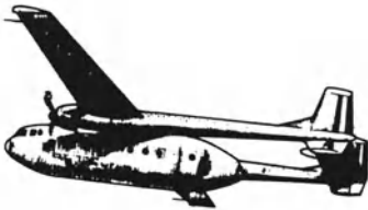
b. Freighter aircraft (Nord 2508) with tail booms and short fuselage afterbody
