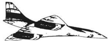
c. Aérospatiale/BAC Concorde supersonic passenger transport; fuselage length/diameter \sim 20
