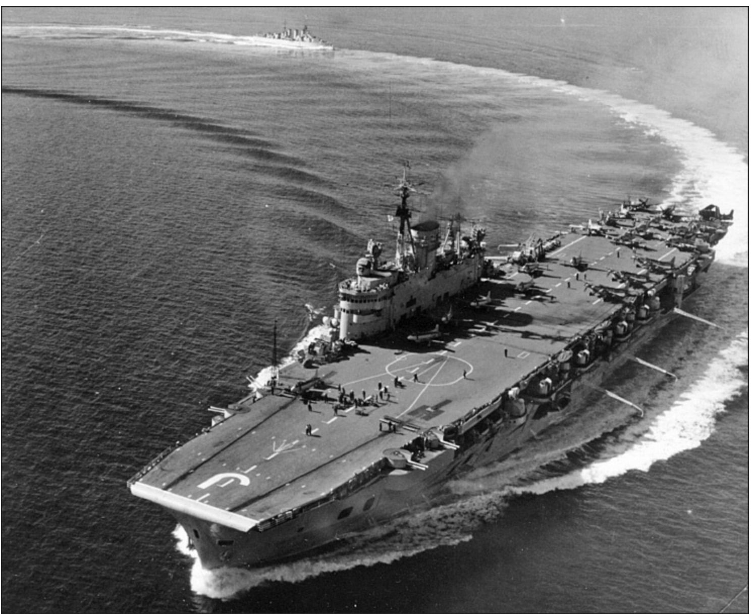
Eagle turns into wind to start a launch, with an Attacker on the starboard catapult. Other aircraft in the range include more Attackers, Fireflies, Sea Hornets and Skyraiders. (AUTHOR'S COLLECTION)
