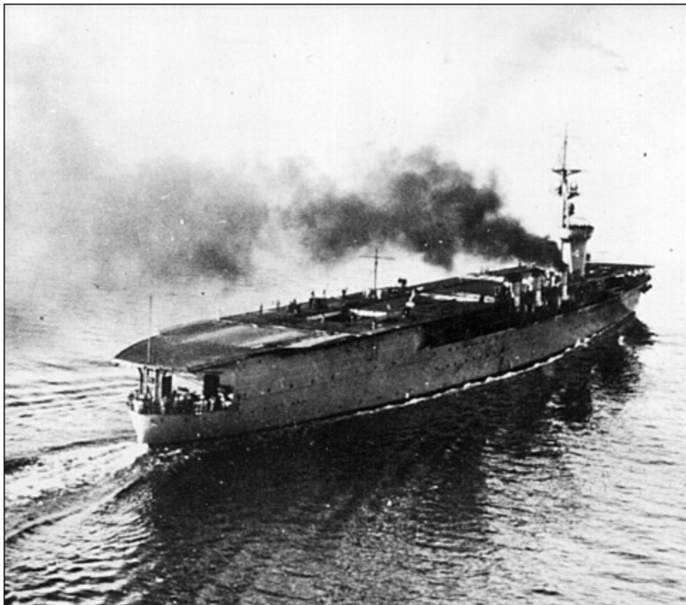
Hosho as built, with a small starboard-side island. (AUTHOR'S COLLECTION)
