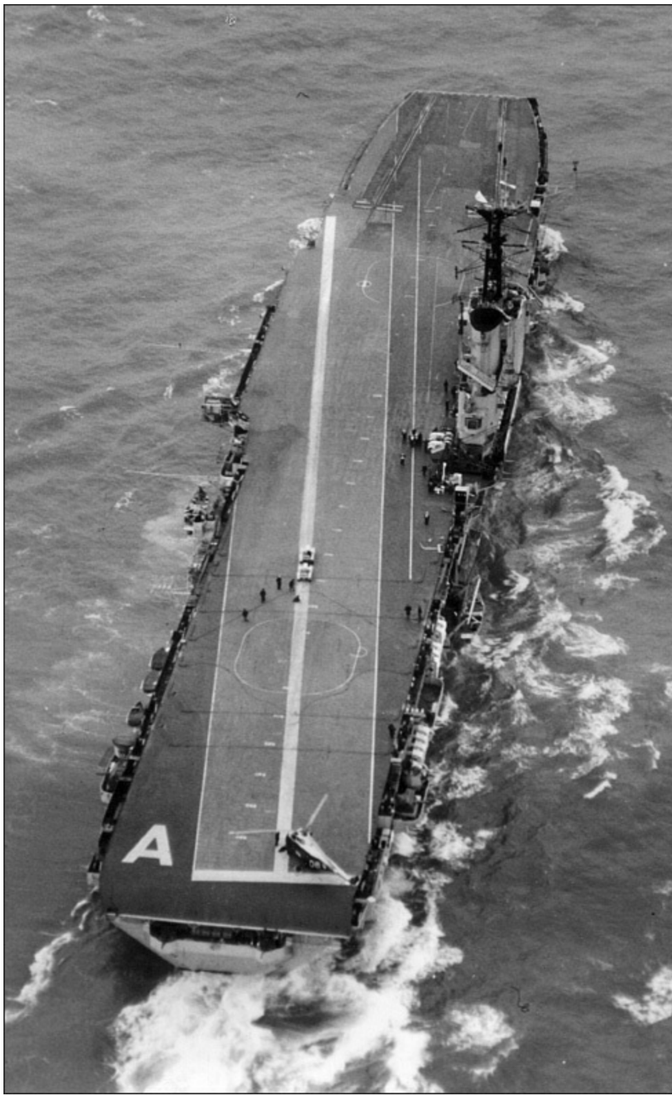
A flight-deck tractor pulls out Albion 's fourth arrestor wire for maintenance in January 1960. The helicopter parked aft is a Whirlwind. (AUTHOR'S COLLECTION)
