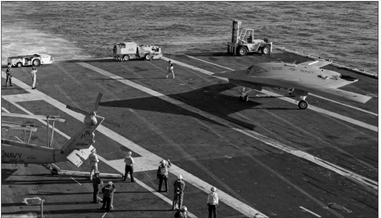
An X-47B taxis around the flight deck of the USS Harry S. Truman . It is directed by a 'yellow-jacket' marshaller in the normal way, but controlled by men with hand-held remote-control units. There are two of the latter in this photograph; one at the top left and one at the bottom centre. Both are facing the X-47. (USN)
