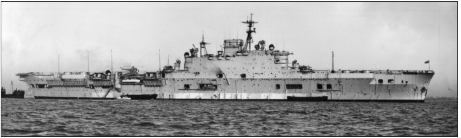
Eagle shortly after her completion as the largest aircraft carrier in the Rn. She was finished to substantially the original Audacious design, but has the most extensive radar outfit yet installed, including two Type 982, two Type 983 and a single Type 960 for long-range air search as well as fire-control and navigation sets. The aircraft on deck is a Dragonfly helicopter. (AUTHOR'S COLLECTION)
