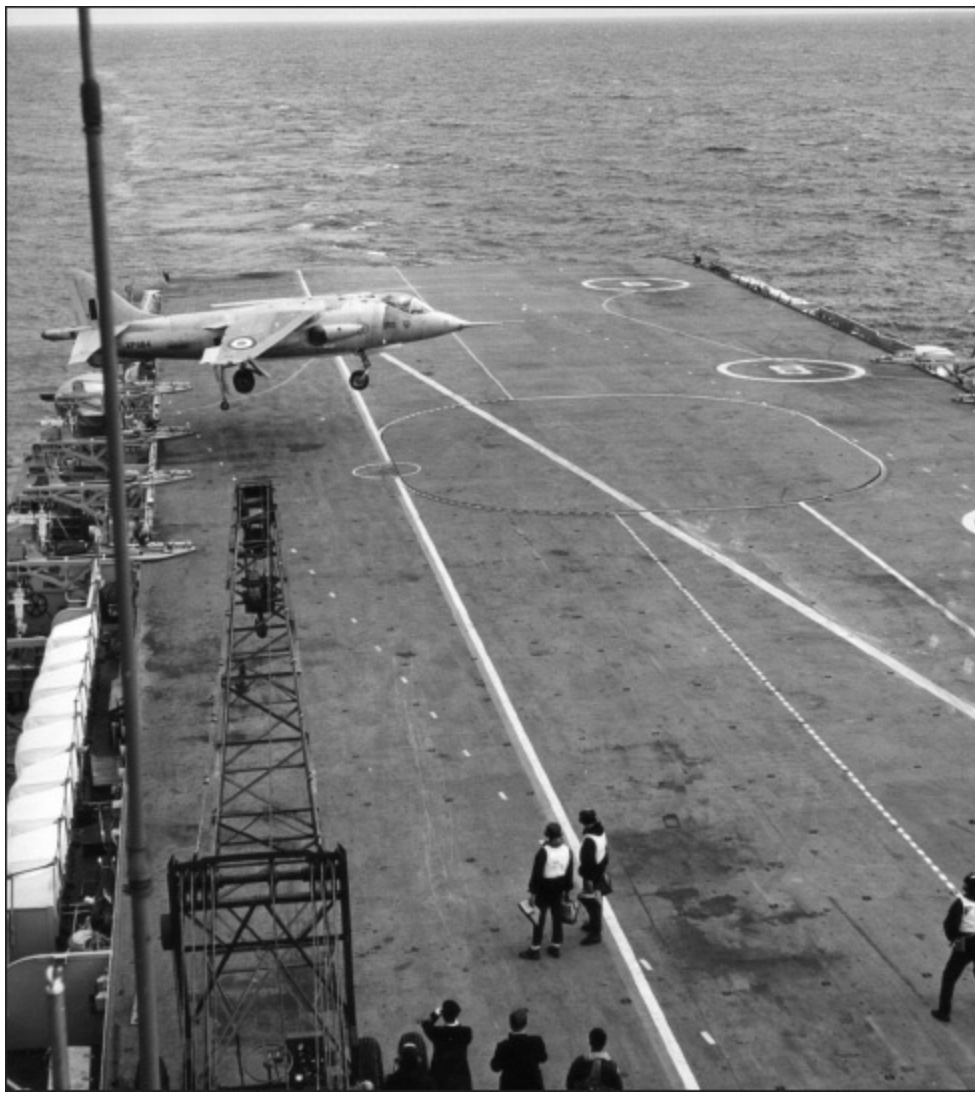
A P.1127 demonstrates its ability to land across the deck with a relative wind on the port beam. While this proved practical on Bulwark in 1966, it was to prove much less practical in the narrower Invincible Class. (AUTHOR'S COLLECTION)
