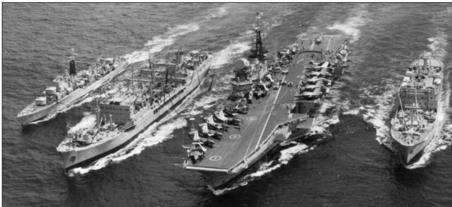
Hermes taking part in a four-ship replenishment at sea with the Far East Fleet while the author was serving in her in 1968. From left to right the ships are the destroyer Diana , a Tide Class RFA tanker, Hermes and the air-stores ship RFA Reliant . Stores from the last-named are being taken on to the side lift, from where they are easily taken into the hangar and struck down. Aircraft on deck are Sea Vixens, Buccaneers, Gannets and a Wessex helicopter. (AUTHOR'S COLLECTION)
