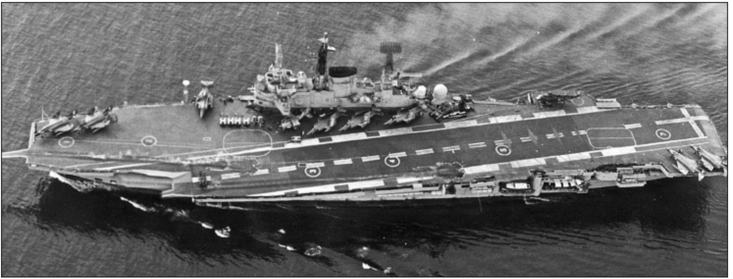
Ark Royal after her special refit, showing the white rectangles painted alongside the angled deck, intended to help pilots orientate their line-up during night deck landings. They showed up well under the low-intensity floodlights mounted on the island and, when clean like this, were very effective. On deck are Buccaneers, Gannets and a Sea King helicopter. (AUTHOR'S COLLECTION)
