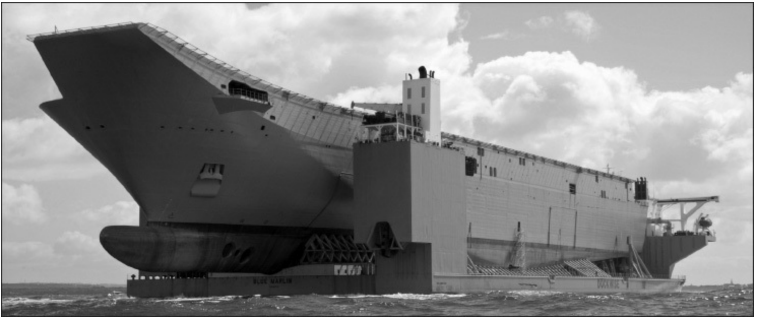
The hull of HMAS Canberra arrives in Australia from Spain, where it was built, on the heavy-lift ship Blue Marlin . (RAN)
