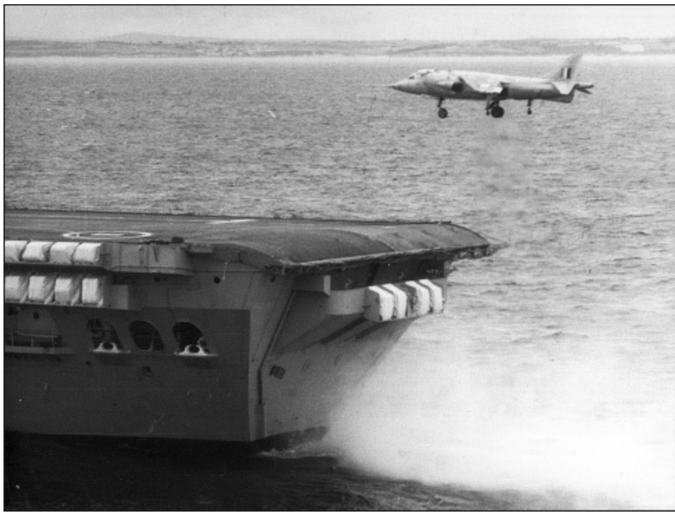
A P.1127 makes a hover-landing on Bulwark in 1966. The jet efflux and the spray it is causing are evident below the aircraft. (AUTHOR'S COLLECTION)
