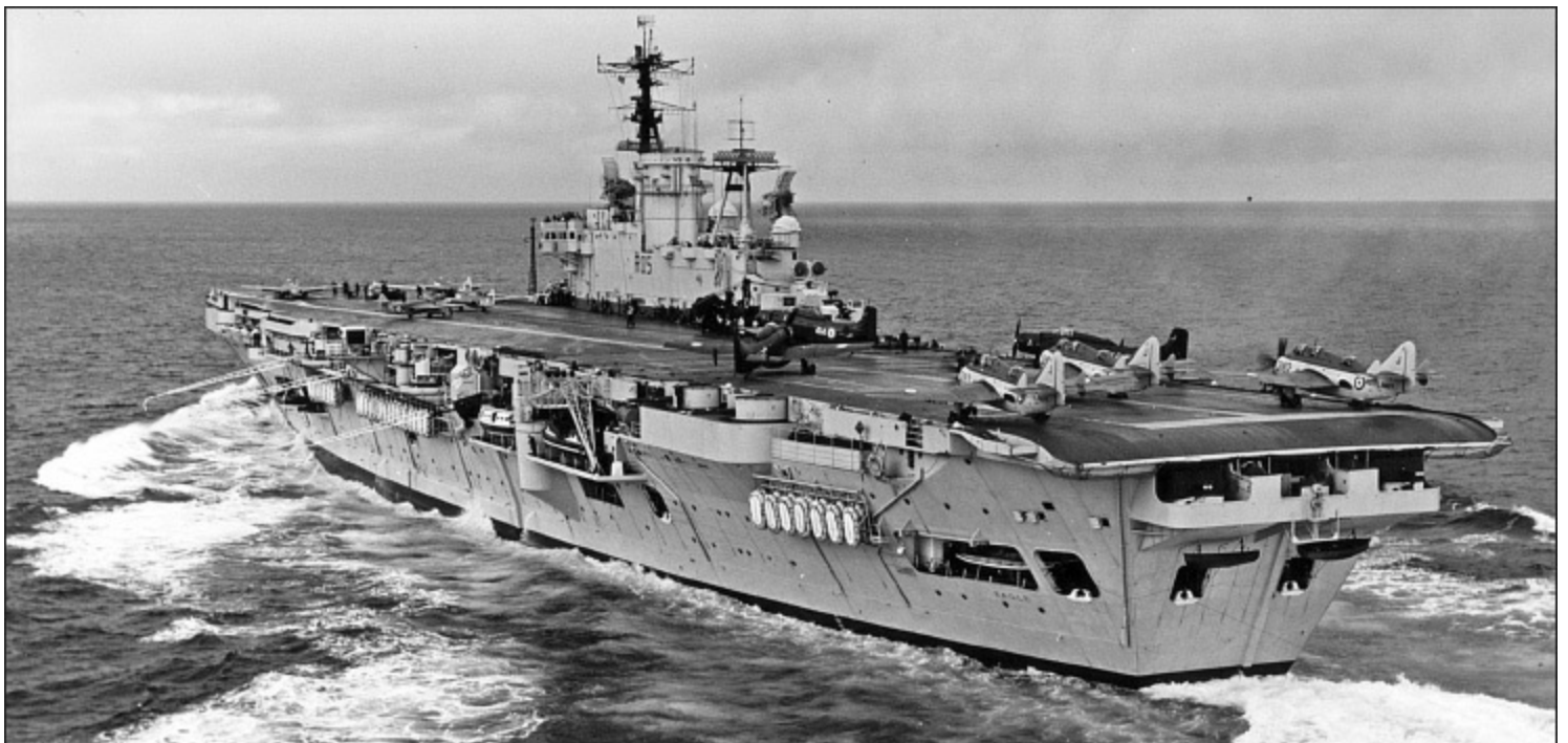
BOTTOM RIGHT Eagle launching her aircraft. Those on the catapults are Sea Hawks; further aft the first of three Skyraiders is beginning to taxi forward, while three antisubmarine Gannets are running, awaiting their turn to move up the deck. (AUTHOR'S COLLECTION)
