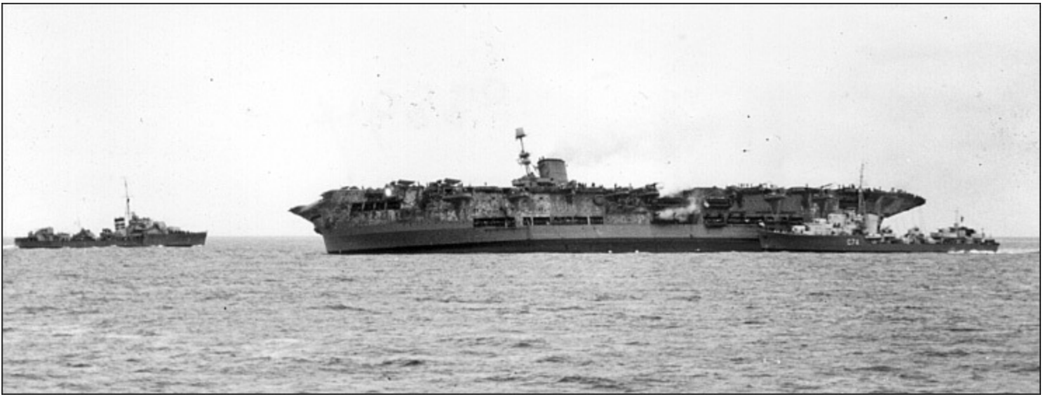
The destroyer Legion alongside Ark Royal 's port quarter. Smoke is issuing from one of the port boat bays, indicating that the normal exhaust trunking is already becoming blocked as flooding sinks the hull lower in the water and the starboard list is not corrected. (AUTHOR'S COLLECTION)
