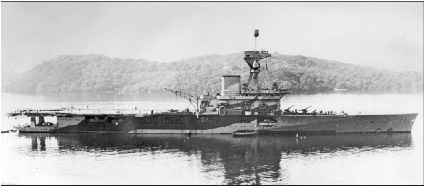
Hermes in a camouflage paint scheme, shortly before her loss in 1942. Note the Type 72 aircraft homing beacon fitted at the highest point of the foremast over the spotting top structure. (AUTHOR'S COLLECTION)
