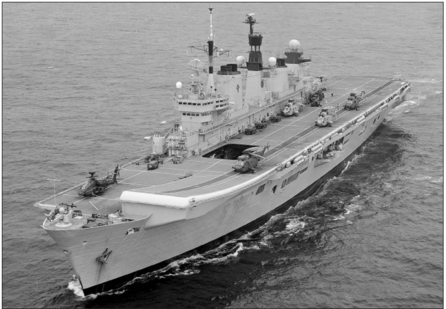
Illustrious operating in the LPH role during 2012. Helicopters on deck include both commando assault and ASaC Sea Kings and an AAC Apache in Fly 1. The latter shows how the extension of the flight deck to starboard of the 'ski-jump' has transformed it into a viable helicopter operating spot. (Crown Copyright/MoD 2012)
