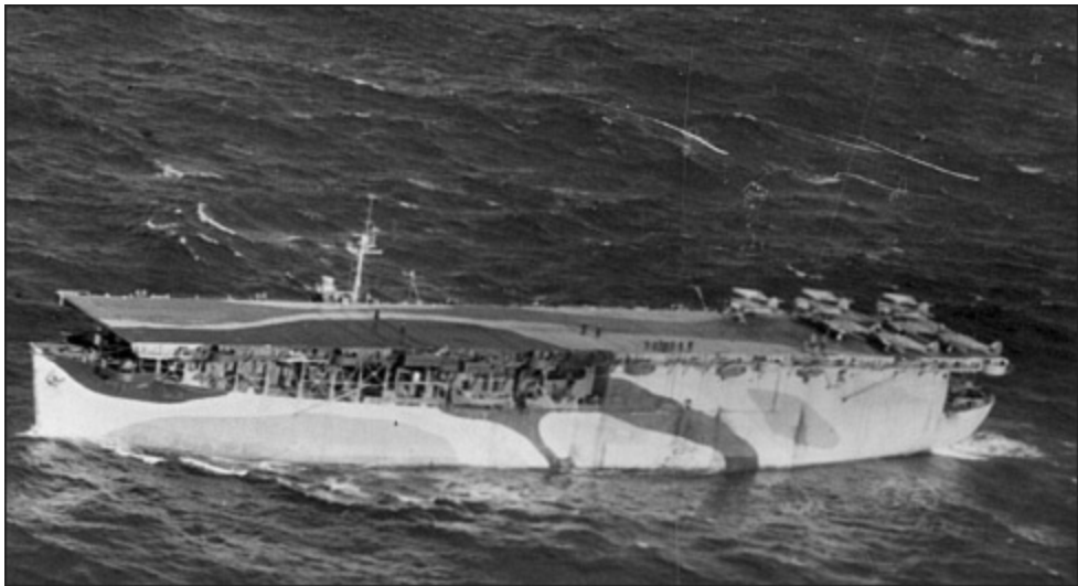
Avenger on 26 October 1942, with Sea Hurricanes and Swordfish ranged aft. The camouflaged flight deck must have made flying visual circuits difficult in some light conditions. (AUTHOR'S COLLECTION)
