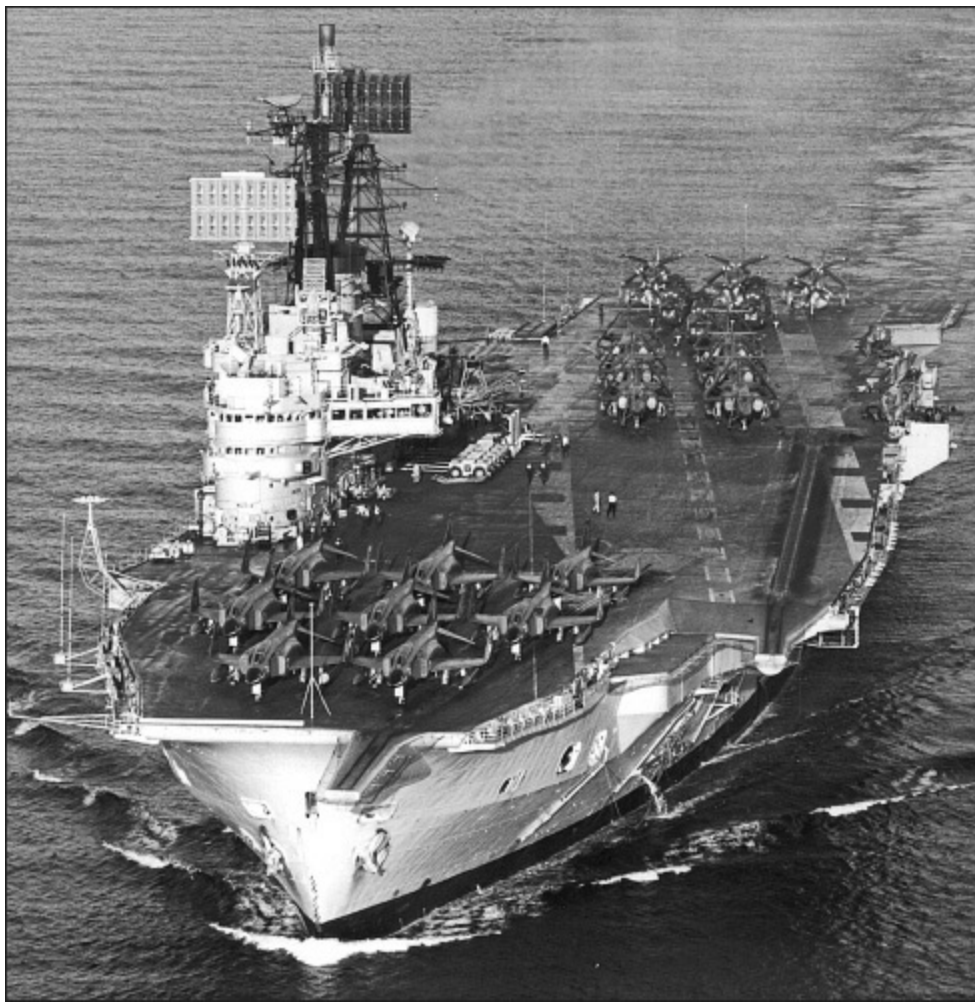
Ark Royal was not fitted with Type 984 radar and Cds, but had the two Type 965Q double arrays shown here. The ‘dustbin’ shape at the highest point of the mast is a Tacan homing beacon. (AUTHOR’S COLLECTION)
