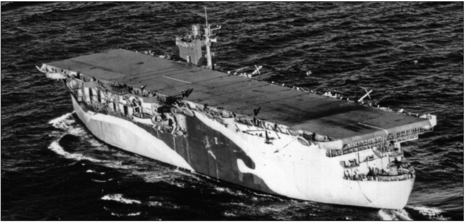
Biter's flight deck was painted grey rather than camouflaged. She is at recovery stations in this photograph, with her W/T masts lowered, but the barriers abreast the small island have not been raised. (AUTHOR'S COLLECTION)
