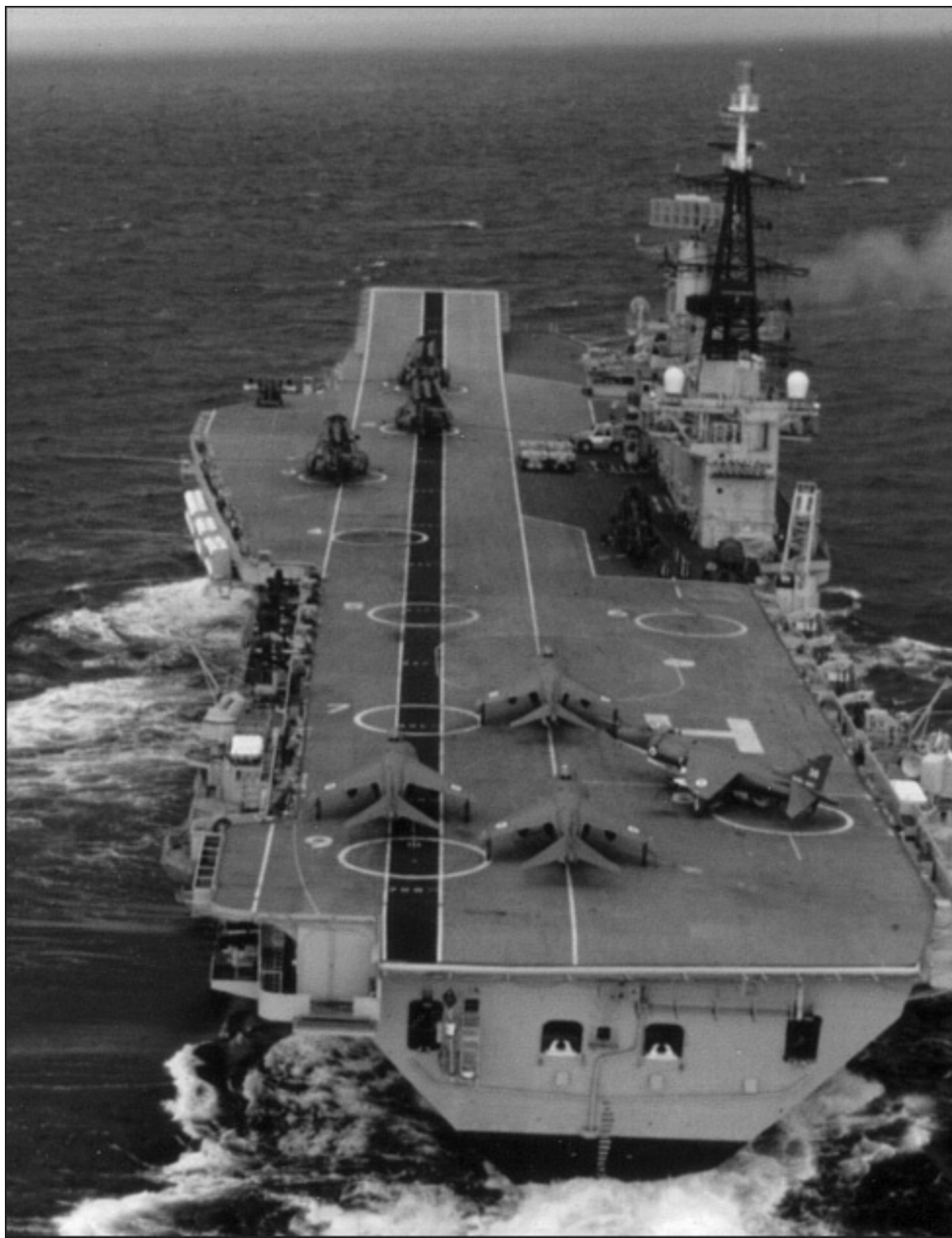
Hermes carrying out flying trials in 1981 after being fitted with a 12-degree 'ski-jump' forward and a new Stovl runway angled one degree to starboard. The projector sight forward of the side lift on the port sponson was part of a trial organised by the author to evaluate its suitability as a Sea Harrier landing aid. It was subsequently adopted and named the 'deck approach projector sight', intended to guide aircraft to a hover position rather than to a point on deck to catch a wire. (AUTHOR'S COLLECTION)
