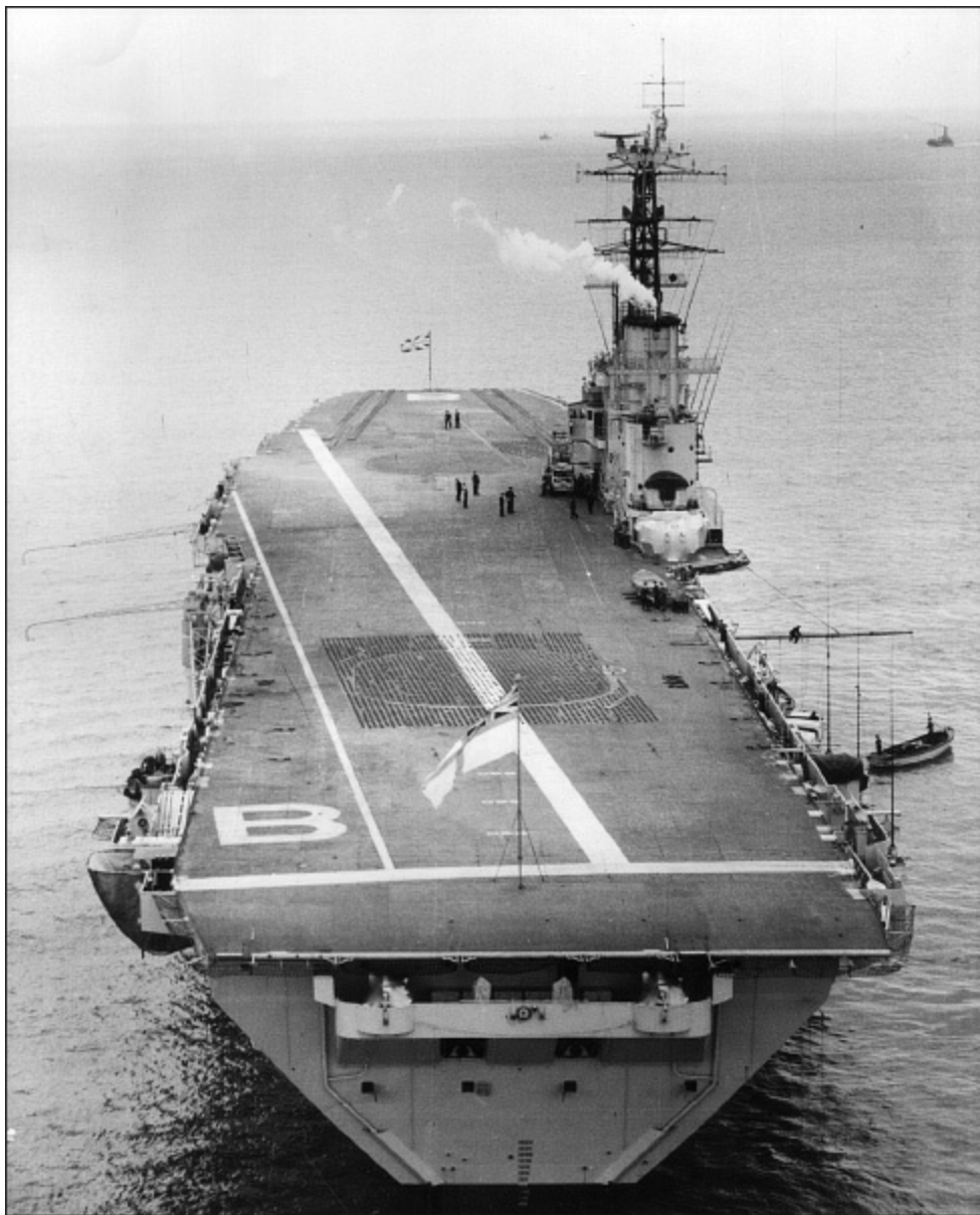
Bulwark only days after completion in November 1954. She is not yet fitted with a mirror landing sight, and the multiple Bofors mounting aft of the island is cocooned. (AUTHOR'S COLLECTION)
