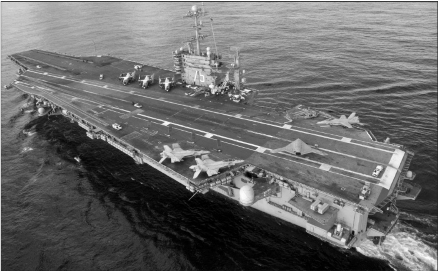
An X-47B on the flight deck of the USS Harry S. Truman , CVN-75, during the embarked compatibility tests that preceded launch and recovery trials. The other aircraft aft near the X-47 are F/A-18 Super Hornets and an MH-60 Seahawk helicopter. Three C-2 Greyhounds are parked forward of the island. (USN)
