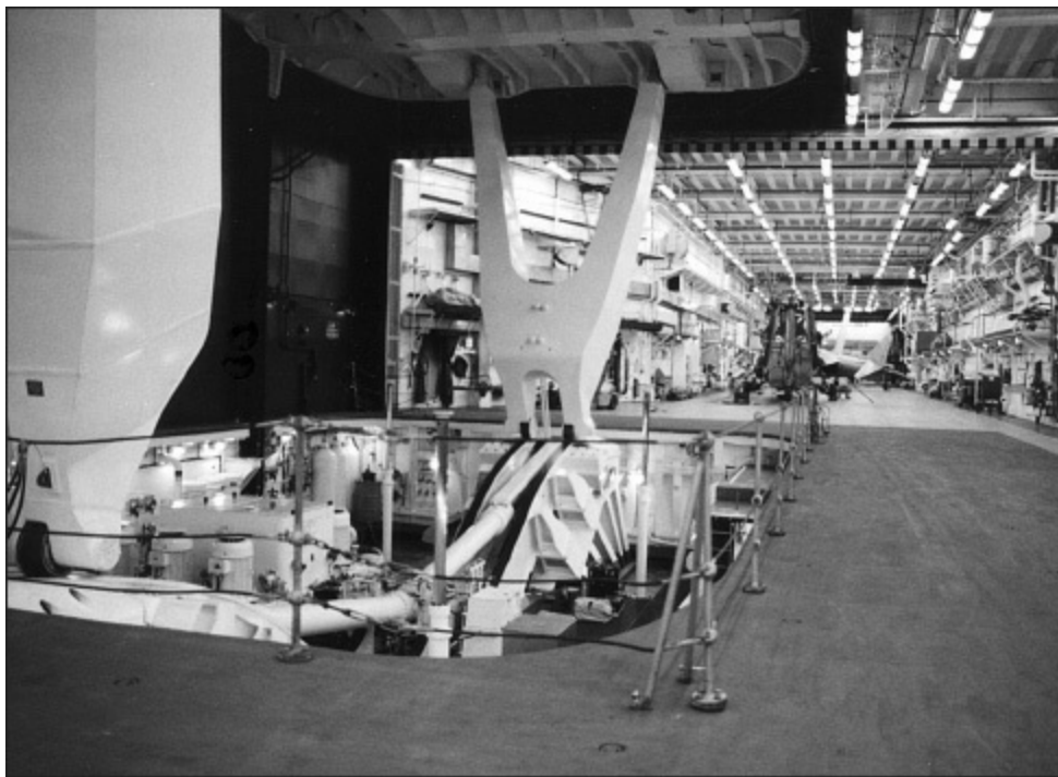
Ark Royal's hangar, looking from aft to forward, with the 'scissor' arms of the after lift in the 'up' position in the foreground. A Sea King and Sea Harrier are secured in the narrow part of the hangar, which was made so by the need for Olympus engine removal lifts, air intakes and exhausts. (AUTHOR'S COLLECTION)
