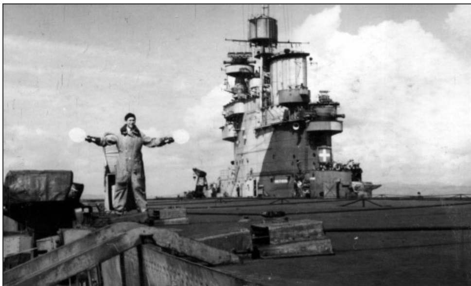
A batsman in Unicorn gives the 'come on' signal. The square 'permission to land' signal below the range-finder 'bandstand' on the rear of the island is showing the 'affirmative' signal. (AUTHOR'S COLLECTION)
