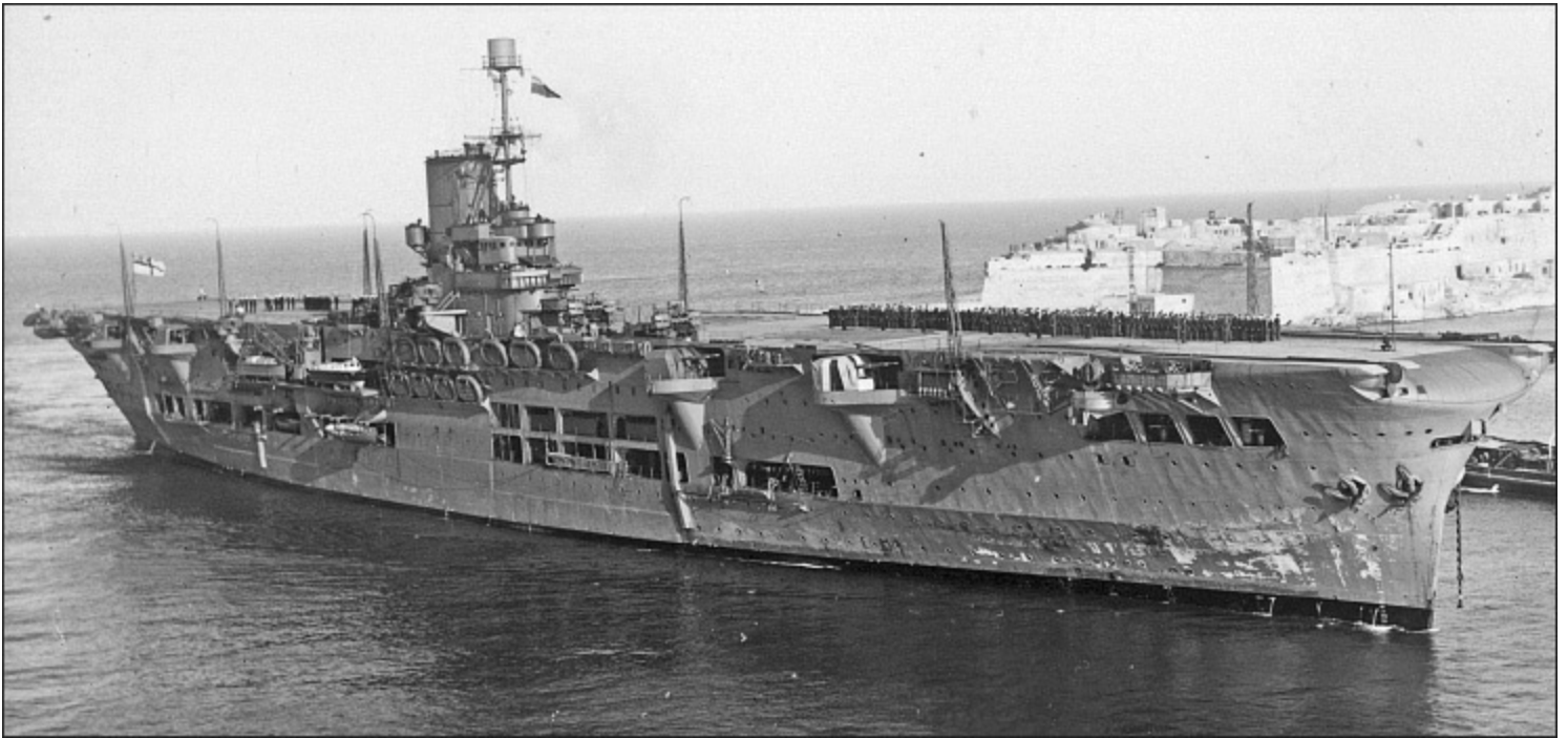
Ark Royal enters Grand Harbour, Malta, during her 'shake-down' Mediterranean cruise in early 1939. The S1 4.5in gun mounting is marked with the red, white and blue neutrality stripes which were painted on British warships during the Spanish Civil War, just coming to an end at the time. The poor state of the paintwork forward shows that she has been through rough weather. The area around the black boot-topping was often repainted by ships' companies as a short-term measure with inadequate preparation. The result, as seen here, was that it was easily washed off. (R A BURT COLLECTION)
