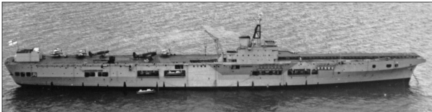
Perseus at anchor while carrying out steam catapult trials in 1951. The full size of the false deck installed to house the prototype catapult is evident. The funnel smoke shows that her bow is into wind, and aircraft are ranged aft ready to taxi forward on to the catapult. They include an Avenger, Sea Fury and two Sea Hornets. The fact that aircraft are to be catapulted into a low natural wind from a stationary carrier shows how powerful the new steam catapult was, and the
