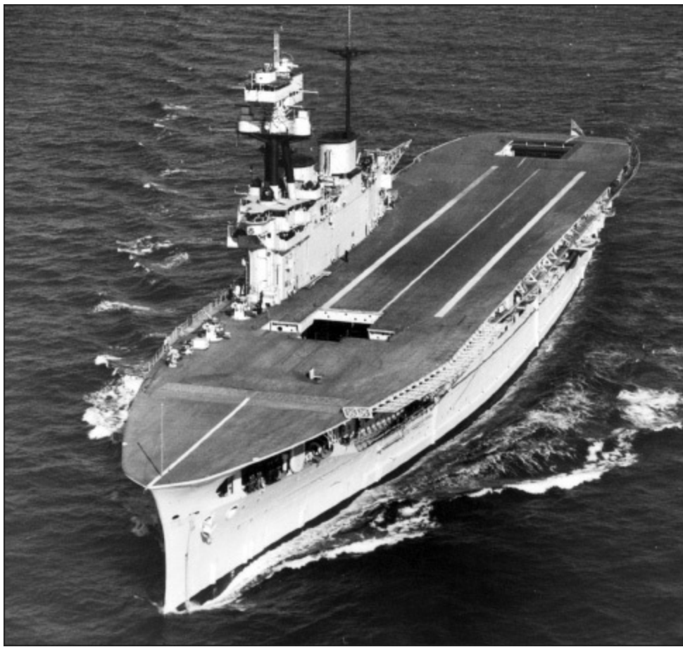
Taken in 1935, this photograph shows Eagle without arrestor wires, although the retaining wires have been removed. The ‘cruciform’ shape of the forward lift allowed aircraft to be struck down with their wings still spread to save time, as the deck had to be clear with the lift up before the next aircraft could land on. (AUTHOR’S COLLECTION)
