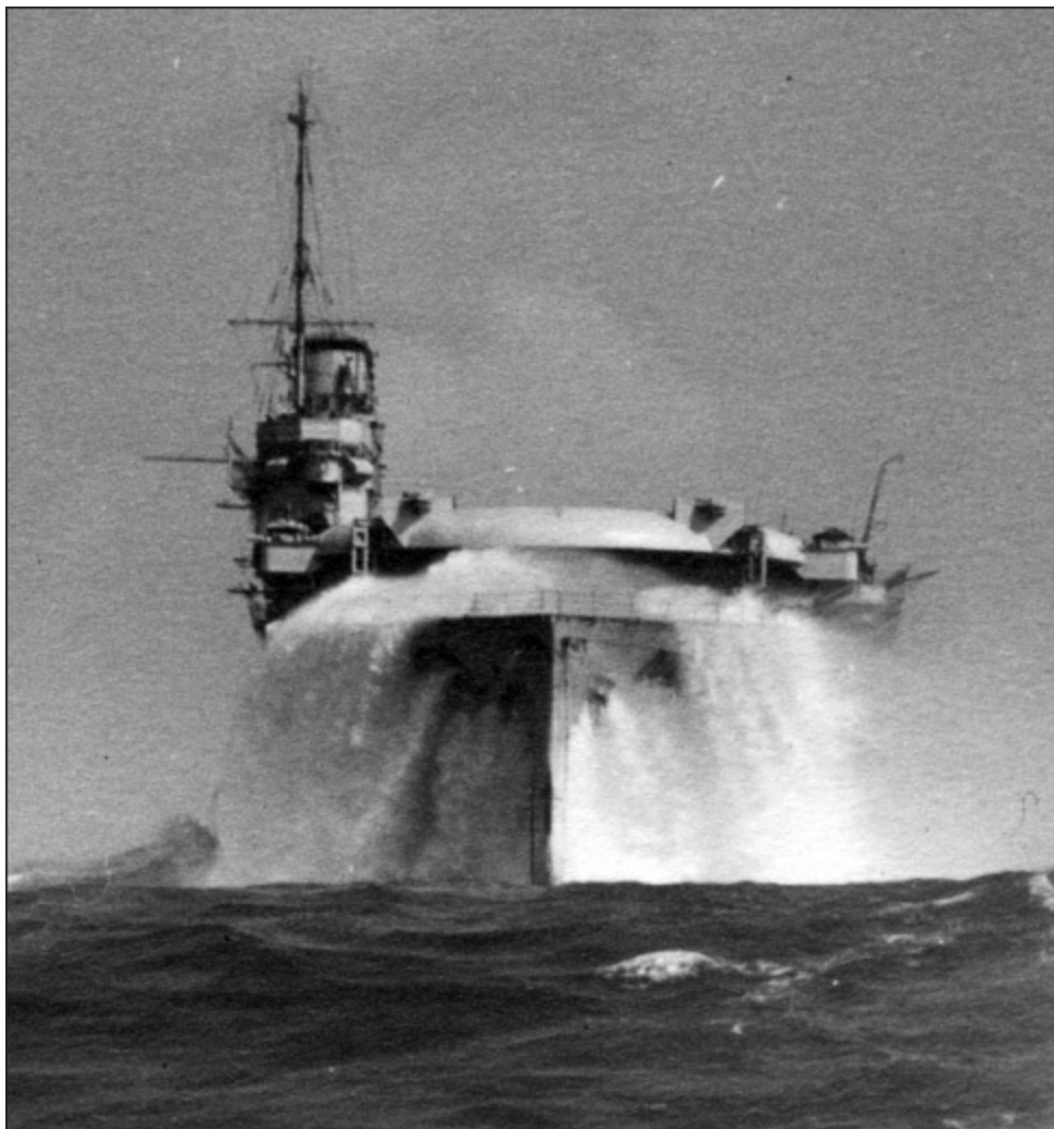
The sea water washing down Glorious ' flying-off deck and crashing into the hangar door show the disadvantage of the design in rough weather. (AUTHOR'S COLLECTION)
