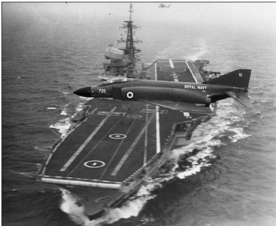
A Phantom from 700P NAS at RNAS Yeovilton over Hermes in the Channel in 1968. It was the requirement to operate Phantoms from Hermes ' relatively small deck that led to the UK variant being re-engined with Rolls-Royce Spey turbofan engines. (AUTHOR'S COLLECTION)
