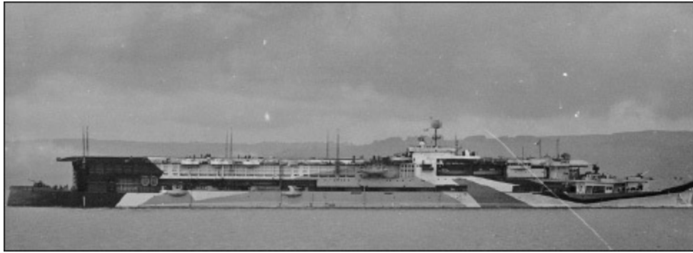
Furious after her final reconstruction, with a small starboard-side island and in Second World War camouflage. Note the anti-aircraft guns and a director mounted on the former flying-off deck forward. (AUTHOR'S COLLECTION)
