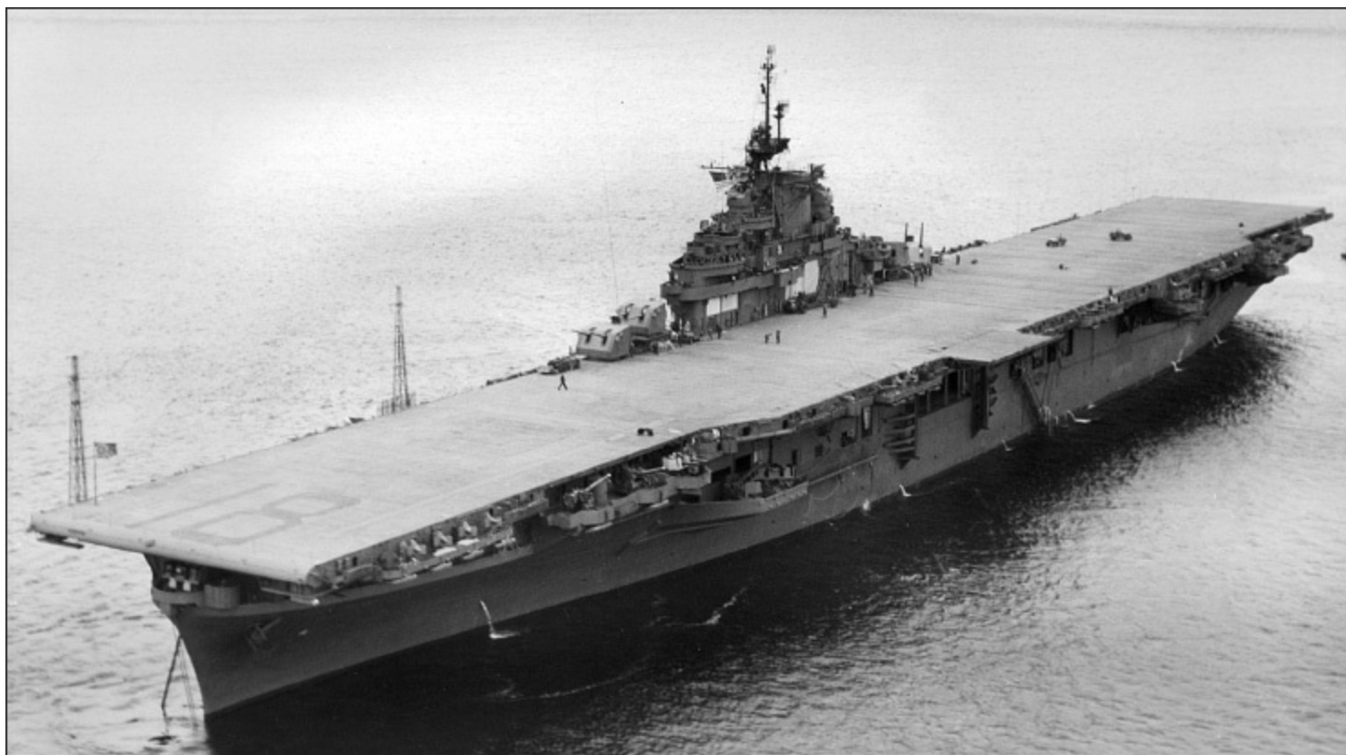
The Essex Class aircraft carrier USS Wasp , CV-18, on 9 June 1945. The structures supporting the side lift guides are clearly visible, as is the opening into the hangar. The white patches on the side of the island are charts showing the ship's company her former achievements in the Pacific Theatre of Operations. (A D BAKER III)
