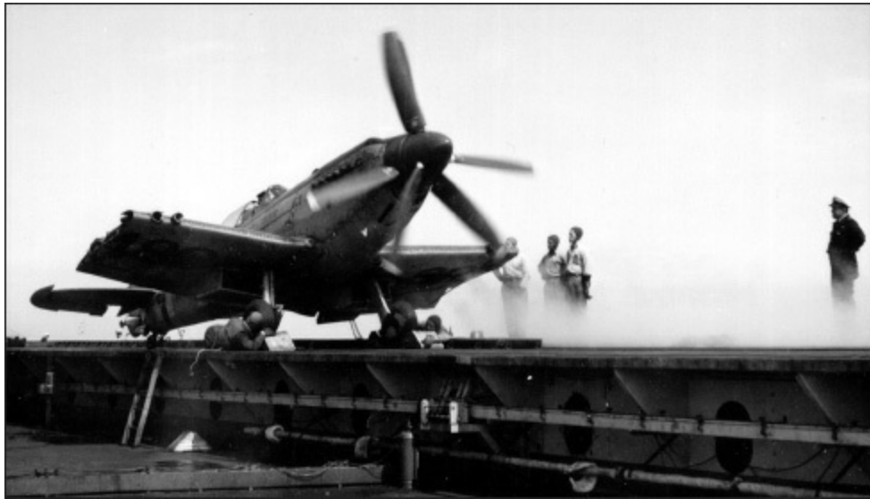
Seafire Vp460 about to be launched in 1951 without a pilot as a 'dead weight' during RN evaluation of Perseus ' prototype steam catapult. The outer wings were removed to ensure that the aircraft did not fly very far but, surprisingly, some of these 'retired' aircraft did not give up without a struggle and flew a considerable distance! (AUTHOR'S COLLECTION)
