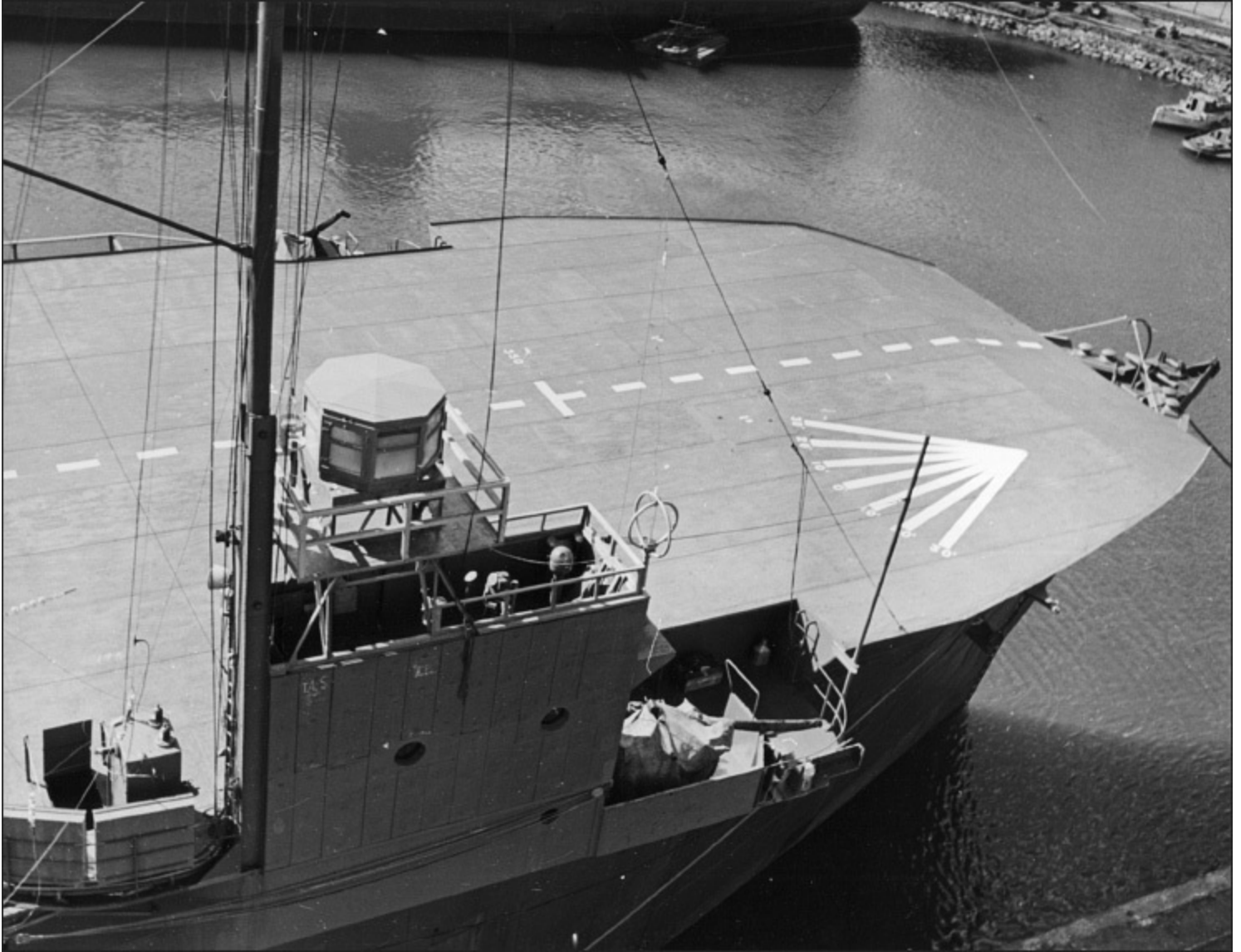
A detailed view of Empire MacAlpine 's island and forward flight deck. The angled white lines show the direction of the wind over the deck from a steam jet positioned at their forward end. (AUTHOR'S COLLECTION)
