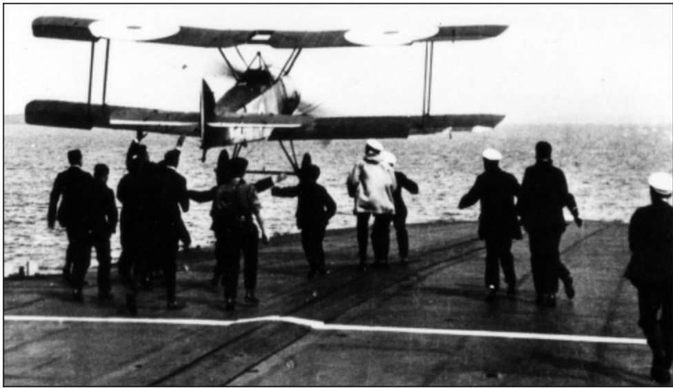
Dunning’s first landing in Pup N6453, the first by an operational naval aircraft flown by a naval pilot on a ship under way at sea. Strops were not fitted to the aircraft at this stage, there is no Vickers gun forward of the cockpit, and there is a triangle of white paint on the aft starboard tip of the lower starboard aileron. The white line painted on the deck is an ‘eye-line’ to guide the pilot over the ideal landing spot. (AUTHOR’S COLLECTION)
