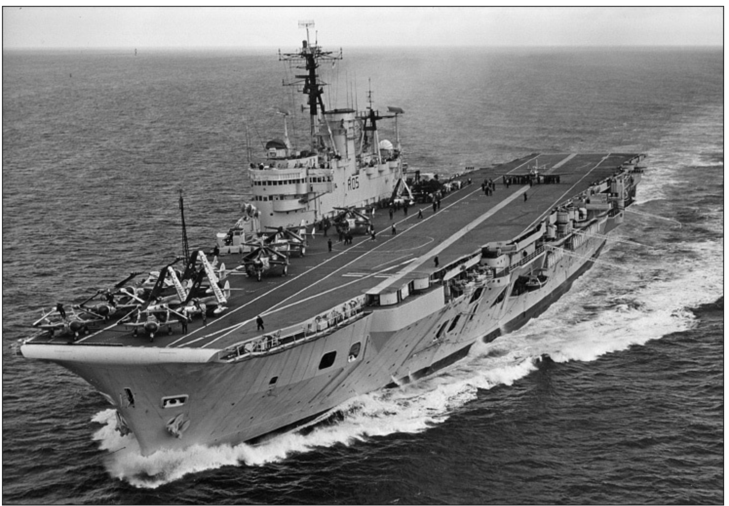
TOP RIGHT Eagle after her flight deck was modified with an interim 4-degree angle. The new centreline passes over the port forward 4.5in gun turrets, which have been plated over. Later 'hay-rake' Type 982 radar aerials have replaced the earlier variety. The aircraft on deck include Sea Venoms, Sea Hawks and Gannets. (AUTHOR'S COLLECTION)
