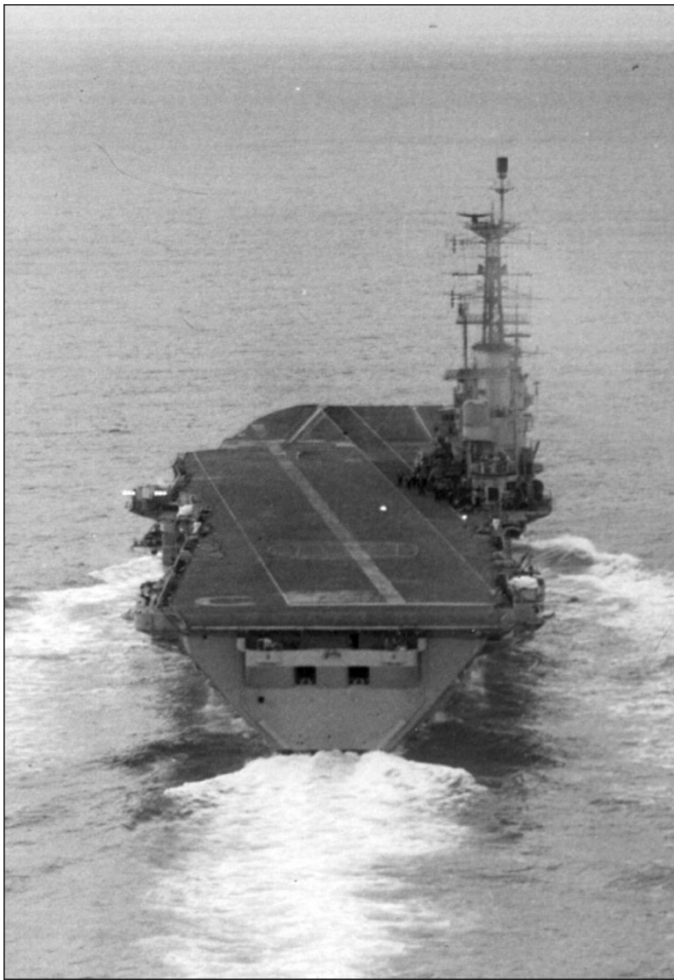
LEFT Centaur's mirror landing aid has been fitted in this photograph, and shows up clearly on the port side, despite the aircraft from which it was taken being lined up with the axial, rather than the angled deck. (AUTHOR'S COLLECTION)
