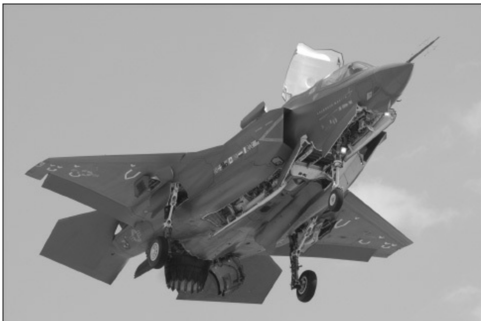
An F-35B in the hover before landing the USS Wasp . Note the rotating jet nozzle aft and the various doors that have to be
