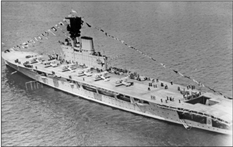
Hermes undergoing sea trials off Plymouth in 1923. The forward windbreak is raised and the tall mast next to it is a temporary, telescopic device with an anemometer on top, intended to give accurate readings of wind flow over the deck before flying trials. (AUTHOR’S COLLECTION)
