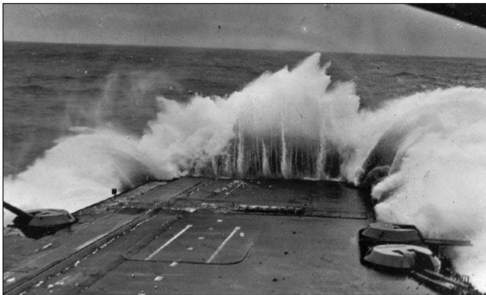
Victorious in rough weather, demonstrating the effectiveness of the British bow design in keeping water off the flight deck. (AUTHOR'S COLLECTION)
