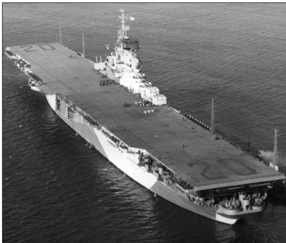
The USS Bennington , Cv-20, in December 1944. The twin 5in mountings fore and aft of the island are conspicuous, as are the raised W/T masts. (A D BAKER III)
