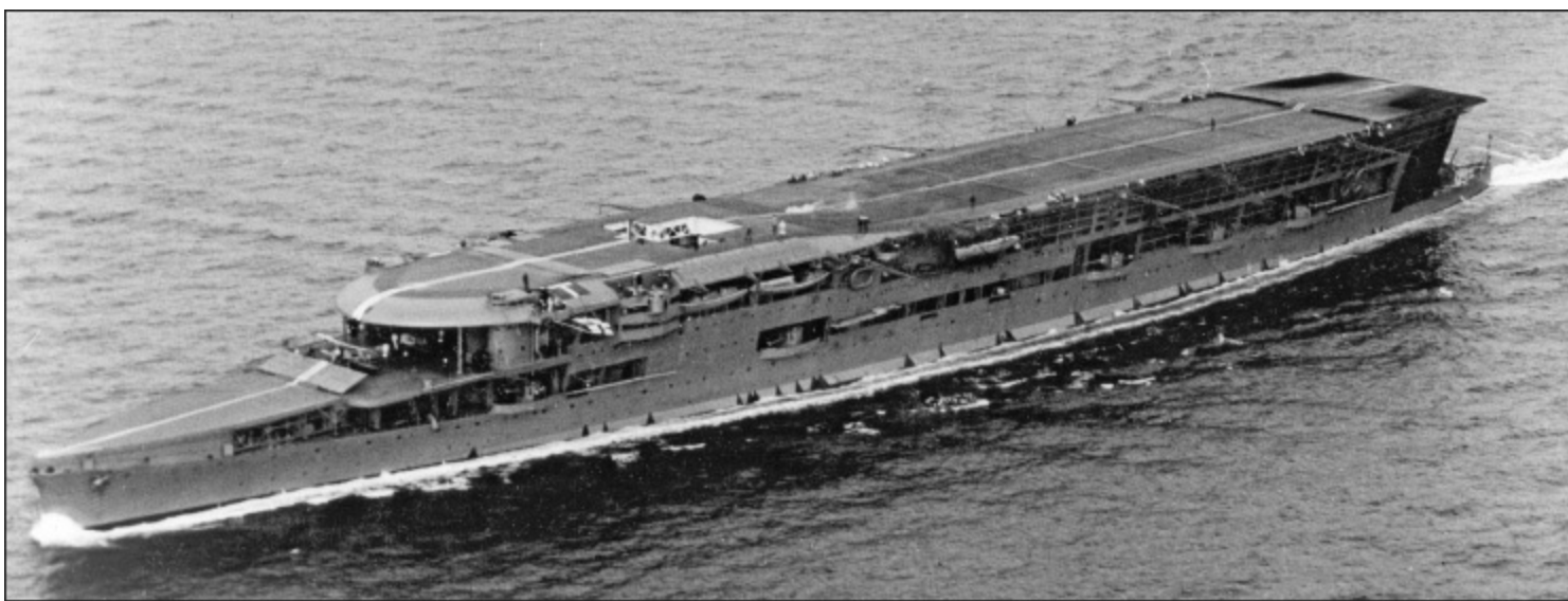
Furious after the third reconstruction completed in 1925. The 'cruciform' lift forward was intended to allow aircraft to be struck down with their wings spread. It was also to prove useful for the early marks of Seafire, which did not have folding wings. Note the soot stains from the funnel exhausts aft. In this photograph she is still fitted with her fore-and-aft retaining wires. (AUTHOR'S COLLECTION)
