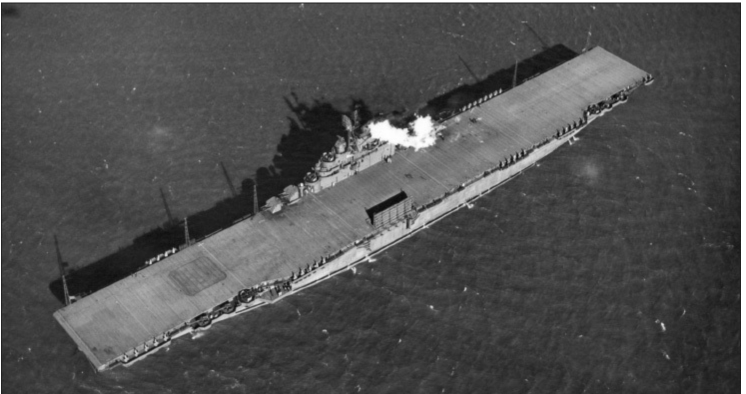
The USS Essex , CV-9, shortly after completion, showing how the side lift could be folded up to reduce the ship's width in pilotage waters. The flight deck is a simple rectangle uncomplicated by the cut-out segment built into British aircraft carriers to improve guns' arcs of fire. The heavy anti-aircraft armament is mounted on sponsons below flight-deck level. (A D BAKER III)
