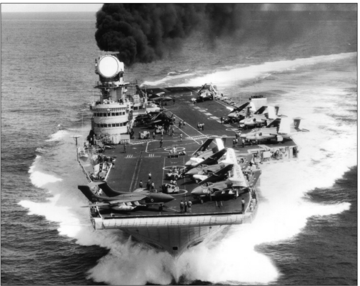
Victorious turning at speed and accelerating; hence the black smoke as more fuel is sprayed into the boilers. The aircraft on deck are Buccaneers, Sea Vixens and Gannets. (AUTHOR'S COLLECTION)
