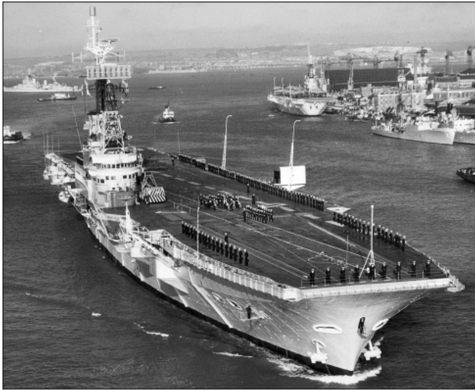
Centaur leaves Portsmouth in her final configuration during 1963, with Type 965 radar mounted on a new foremast. The carrier in the background is HMCS Bonaventure . (AUTHOR'S COLLECTION)
