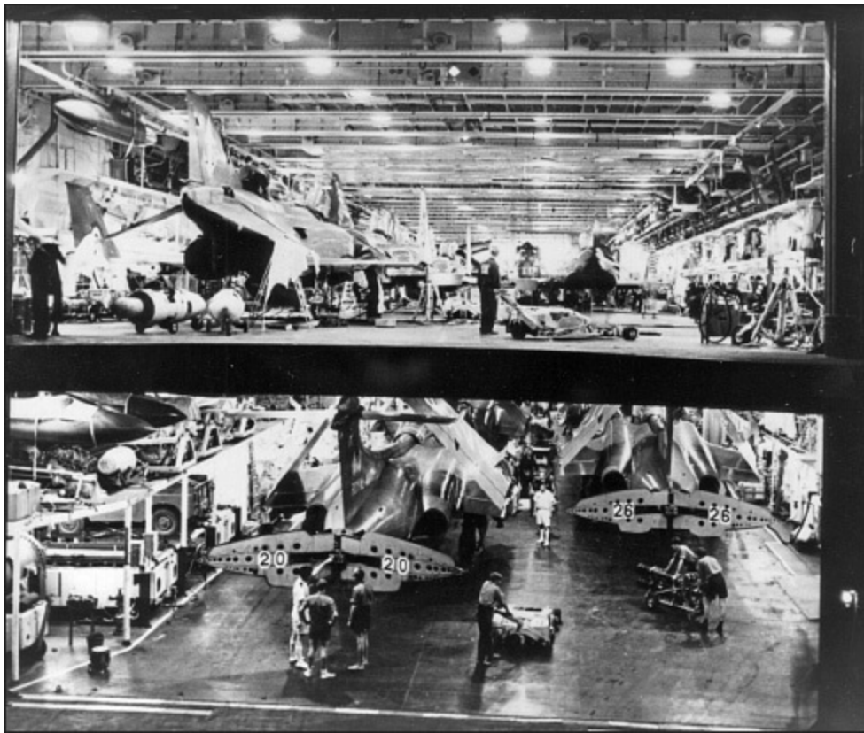
Ark Royal's two hangars photographed from the forward lift at its mid position. Buccaneers used the lower hangar; Phantoms, Gannets and Sea King helicopters the upper. (AUTHOR'S COLLECTION)
