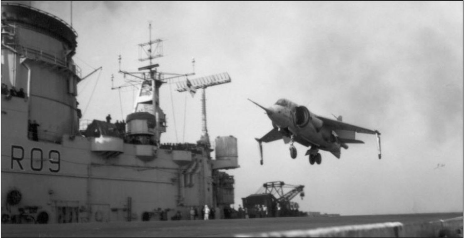
This iconic image shows a prototype Hawker P.1127 in the hover before making the world's first vertical landing by a fast-jet on an aircraft carrier. It took place on Ark Royal on 8 February 1963. (AUTHOR'S COLLECTION)
