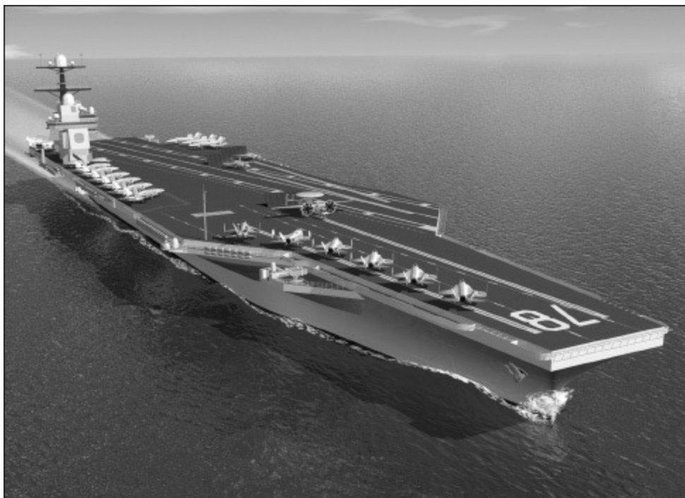
An artist's impression of the USS Gerald Ford , CVN-78, showing the smaller island sited further aft than in the previous Nimitz Class.
