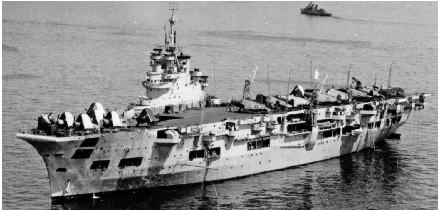
Unicorn serving with the B PF in 1945. She has Corsairs and Avengers on deck, and the two rectangular openings just below the flight deck right forward allow air to flow through the engine test bay so that engines can be run-up to full power inside. The B PF pennant number R108 is just visible below the after forecastle opening, on the panel of darker paint. (AUTHOR'S COLLECTION)
