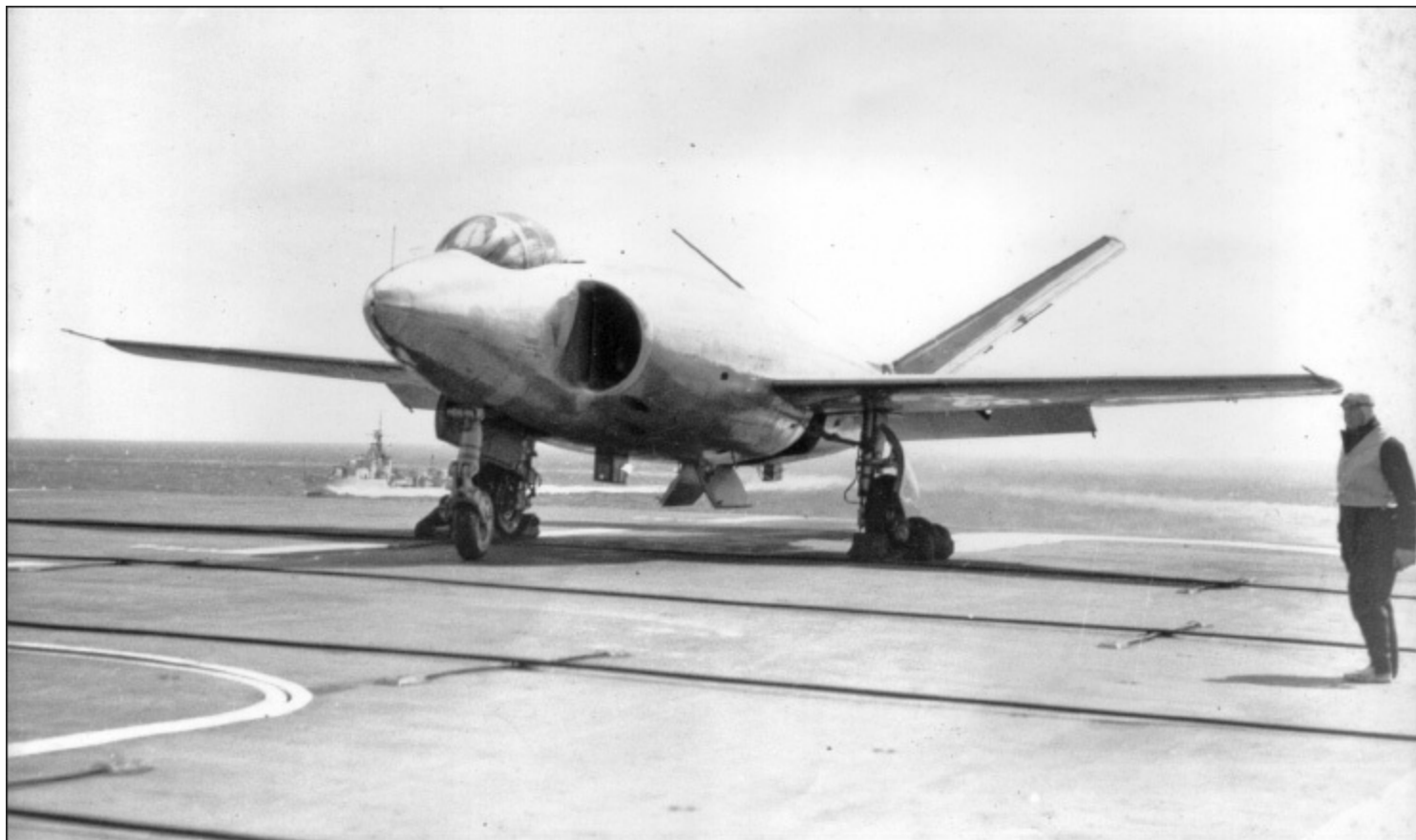
The prototype Supermarine Type 508 carrying out flying trials in Illustrious . The developed version was originally intended to operate without an undercarriage. (AUTHOR'S COLLECTION)
