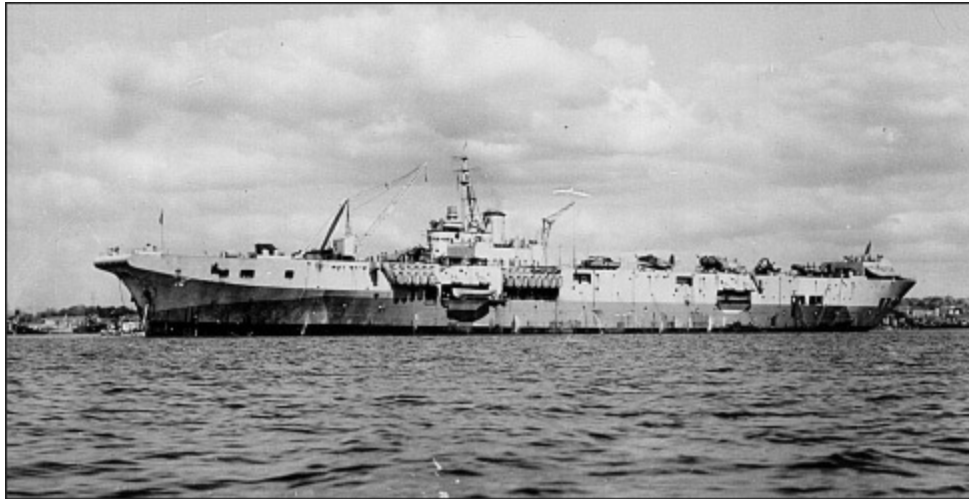
Pioneer in Sydney Harbour in 1945, showing the many differences between her and her half-sisters, the light fleet carriers. She has no sponsons, and single 20mm Oerlikons are mounted in 'tubs' around the upper deck edge. The distinctive crane on the port side forward is clearly visible, as is the boxlike structure to port of the island. (RAN)
