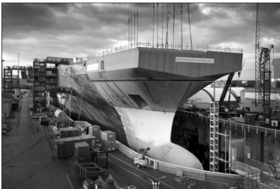
The final bow section, the last part of Queen Elizabeth's flight deck, being lowered into place in Number 1 Dock in Rosyth on 8 February 2013. (AIRCRAFT CARRIER ALLIANCE)
