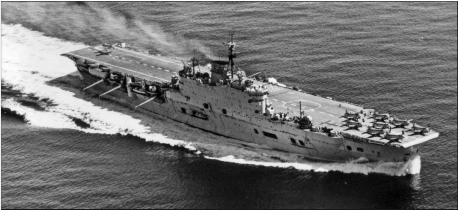
Eagle recovering Attackers of 800 and 803 NAs. Eight have already landed-on, and another is about to catch a wire. Just visible to port of the island are the two nylon barriers which had to be rigged for Attacker recoveries, since, without an engine in front of the pilot to absorb the impact, they could not use the normal steel wire barriers. (AUTHOR'S COLLECTION)
