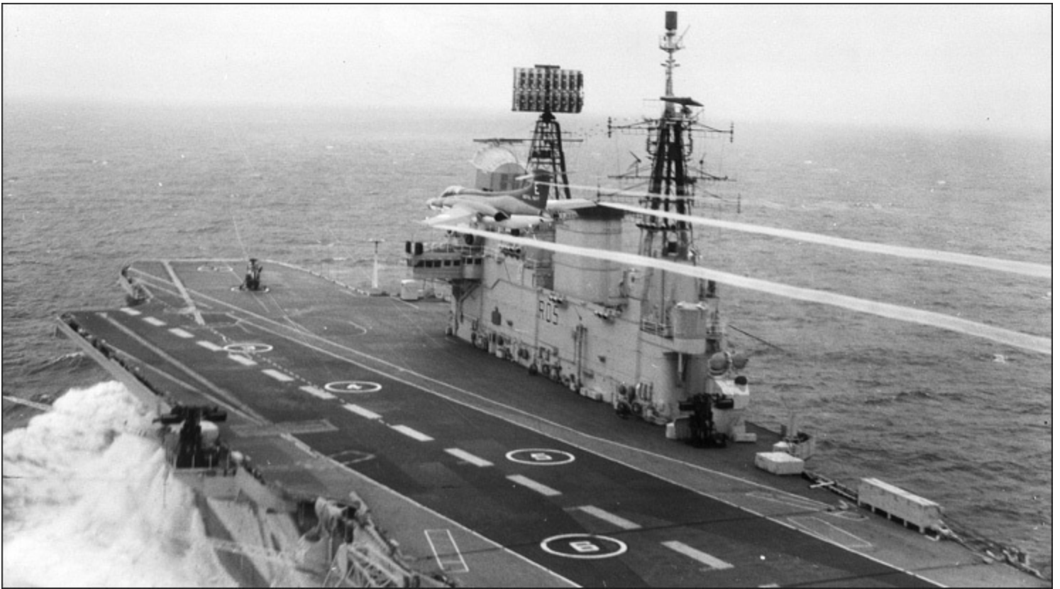
A Buccaneer of 800 NAS makes a low pass over Eagle . Wingtip vortices like these are common at high speed in the moist air close to the sea surface. (AUTHOR'S COLLECTION)
