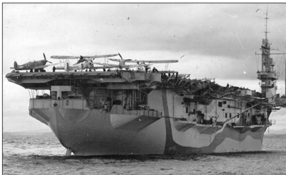
Seafires and Swordfish of 816 NAS ranged aft on Tracker . The H F /D F mast on the starboard side right forward is conspicuous. (AUTHOR'S COLLECTION)
