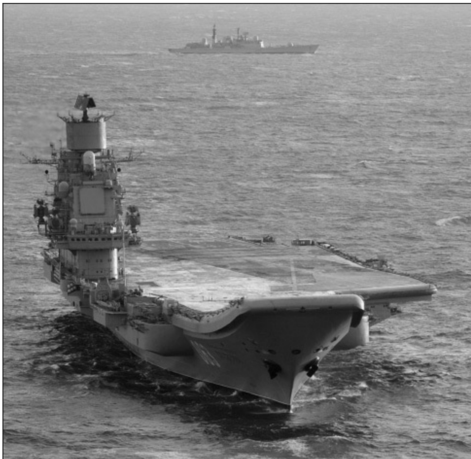
Admiral Kuznetsov with the British destroyer York in the background. This image shows the width of the flight deck across the angle and the prominent ‘ski-jump’ forward. (CROWN COPYRIGHT/MoD 2012)
