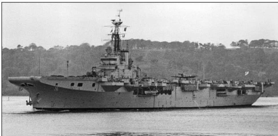
Warrior sailing from Devonport after her initial modernisation, which included the installation of a lattice mast. (AUTHOR'S
