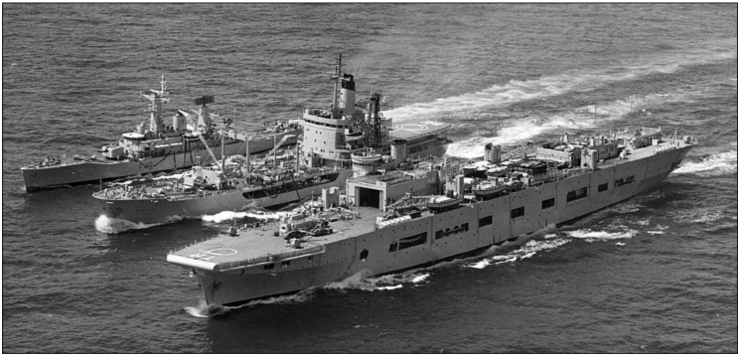
Triumph after conversion into a fleet repair ship, refuelling at sea from RFA Blue Rover , with Minerva on the other side of the tanker. The box-like structure to port of the island is a hangar for helicopters disembarked from ships alongside for maintenance; the circle painted on the deck near the bow is their designated landing spot. A Wasp helicopter is parked aft of the spot, with the crane 'Jumbo' secured astern of it. (AUTHOR'S COLLECTION)
