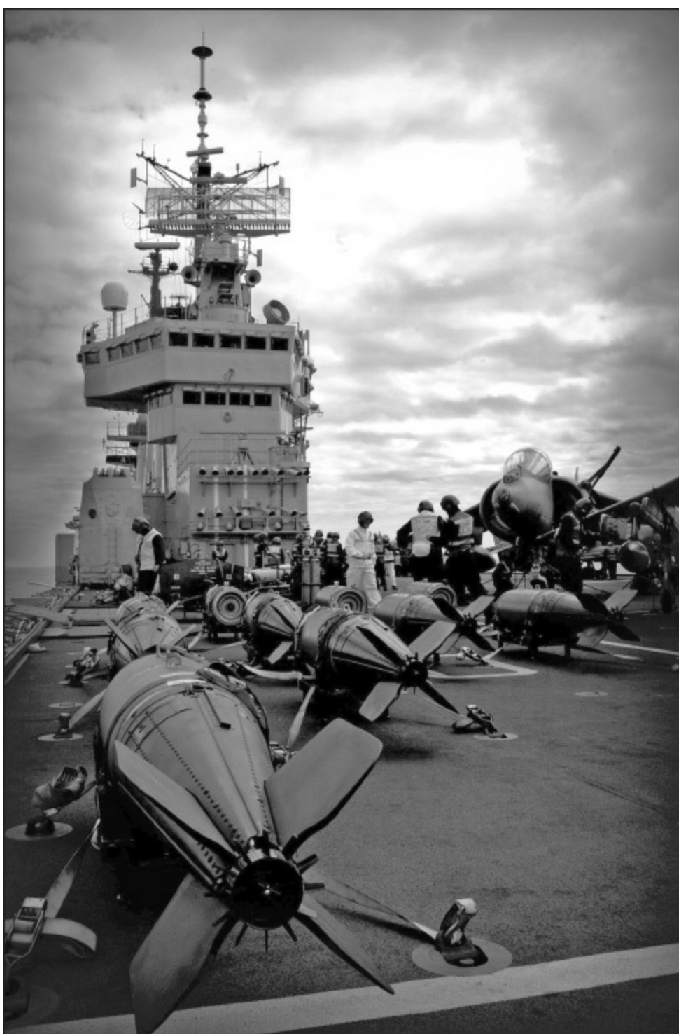
Preparing 1,000lb bombs in Illustrious ' Fly 1 for Harriers of the Naval Strike Wing. (Crown Copyright/MoD 2012)
