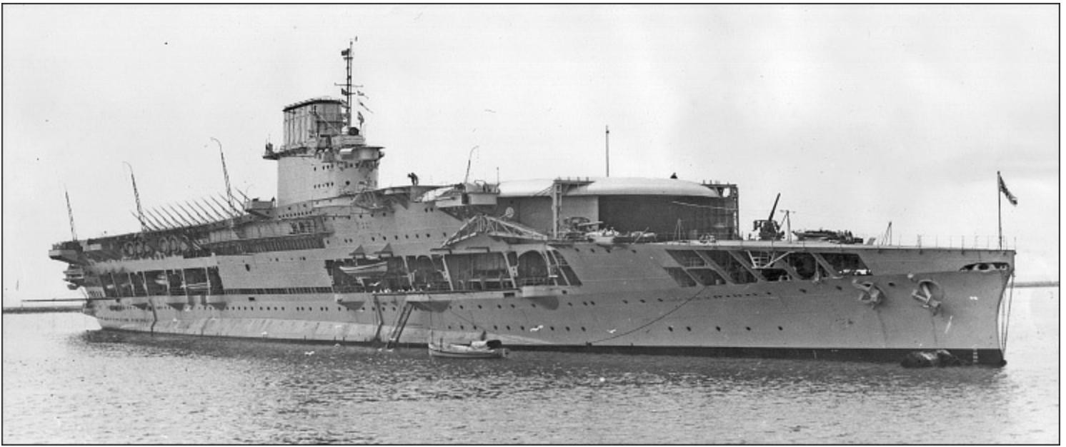
Courageous before she was fitted with catapults and arrester wires. The door from the upper hangar on to the flying-off deck is open. (AUTHOR'S COLLECTION)
