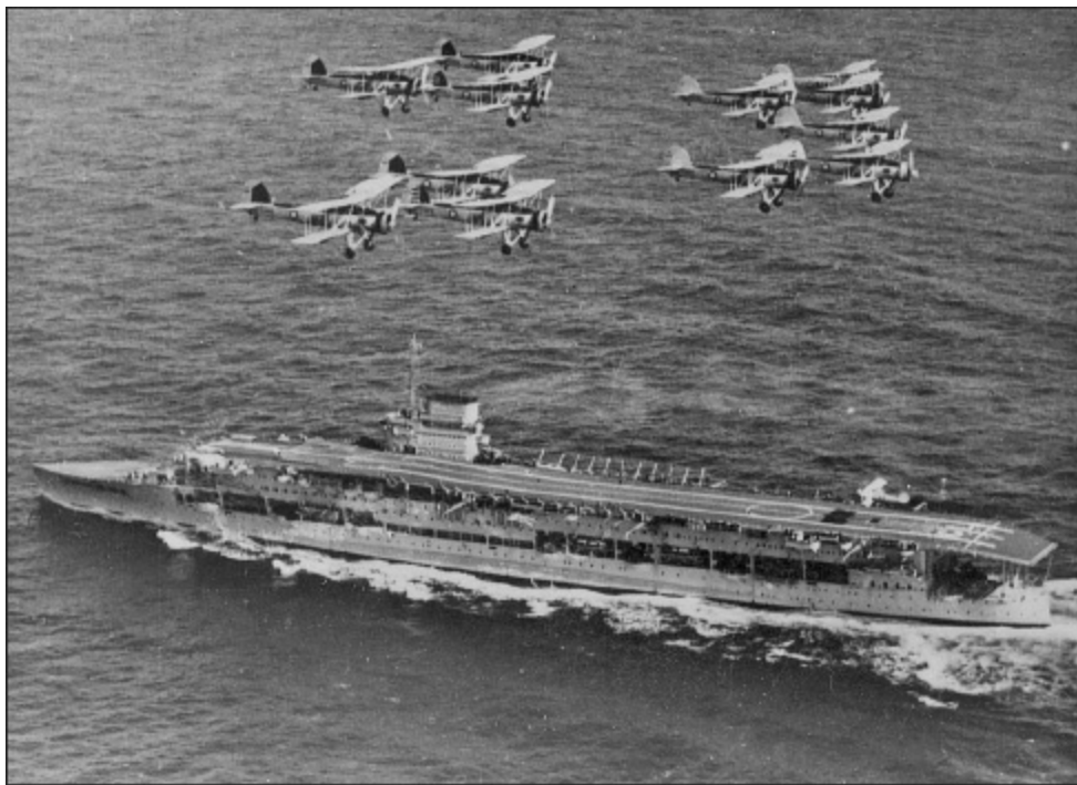
A Swordfish lands on Glorious while others join overhead in formation. The 'W' shaped bracket under the extended round-down is a distinctive recognition feature for this ship, but the letters GL painted on the after part of the flight deck confirm her identity. (AUTHOR'S COLLECTION)
