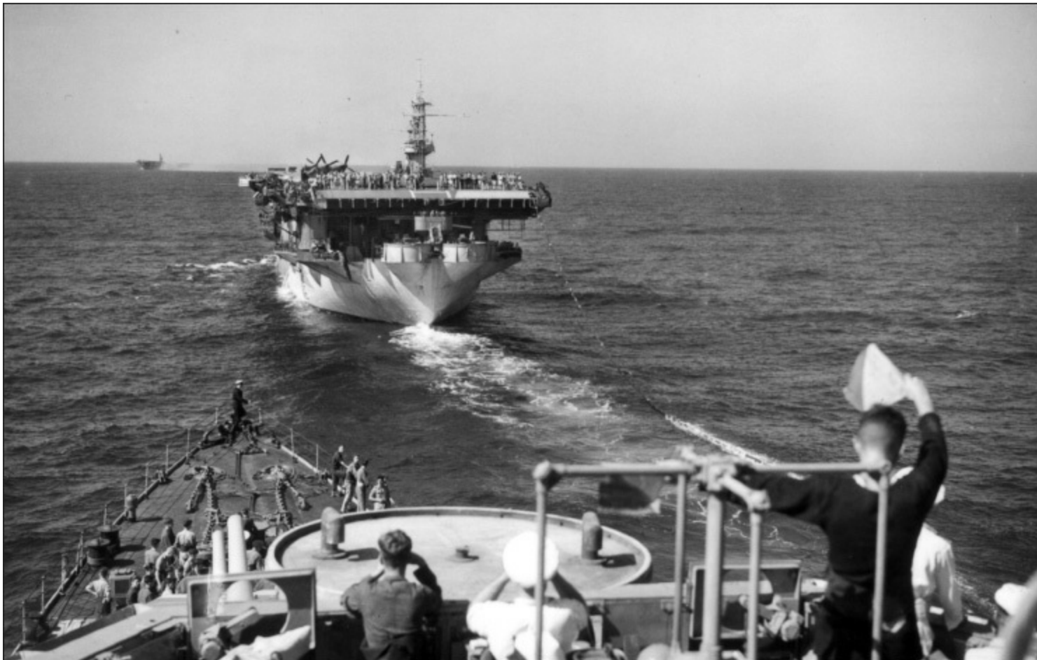
A tactical signalman sending a semaphore message from Royalist to Hunter while the cruiser takes on fuel from a buoyant hose towed astern of the Cve. The escort carriers' large fuel stowage made them additionally useful for replenishing other warships at sea. (AUTHOR'S COLLECTION)
