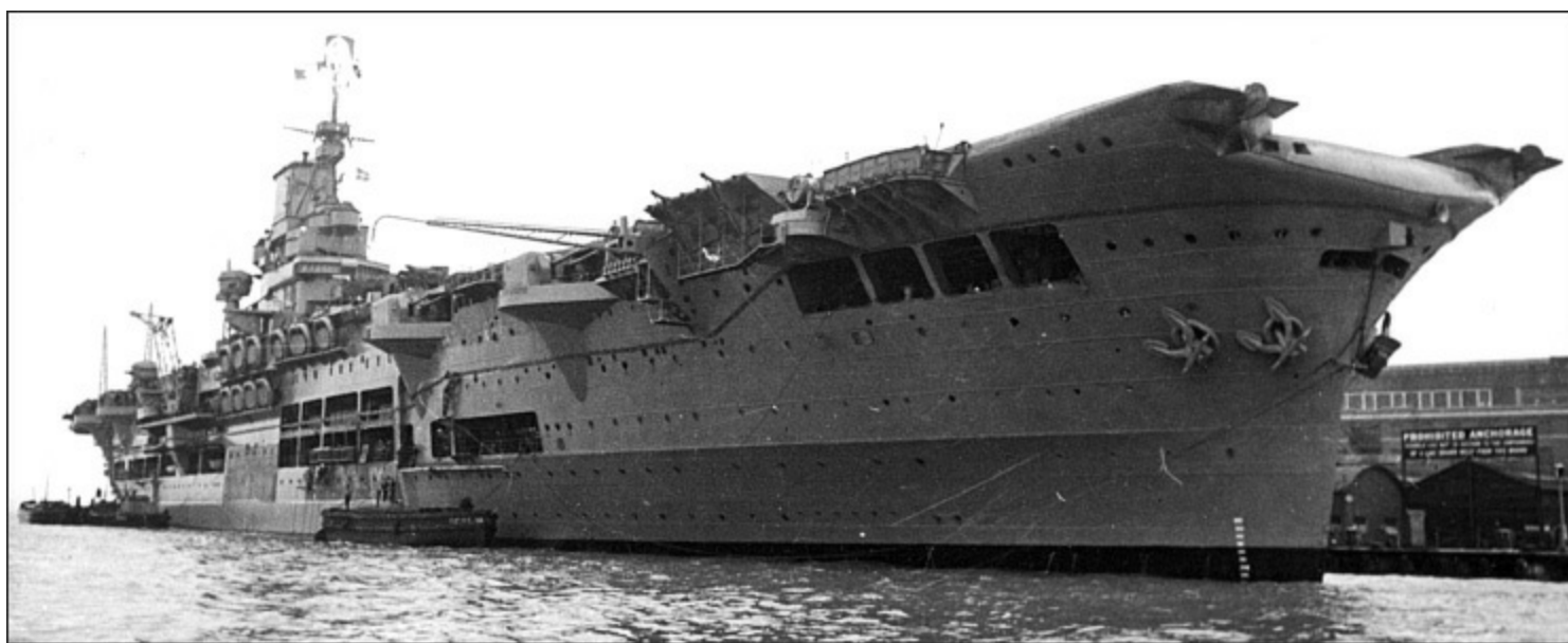
Ark Royal alongside in Portsmouth early in the Second World War. The censor has made a halfhearted attempt to blank out the Type 72 aircraft homing beacon, but this photograph gives a good view of the structure that supported the two catapults. The recently fitted external degaussing coil also shows up well. (AUTHOR'S COLLECTION)
