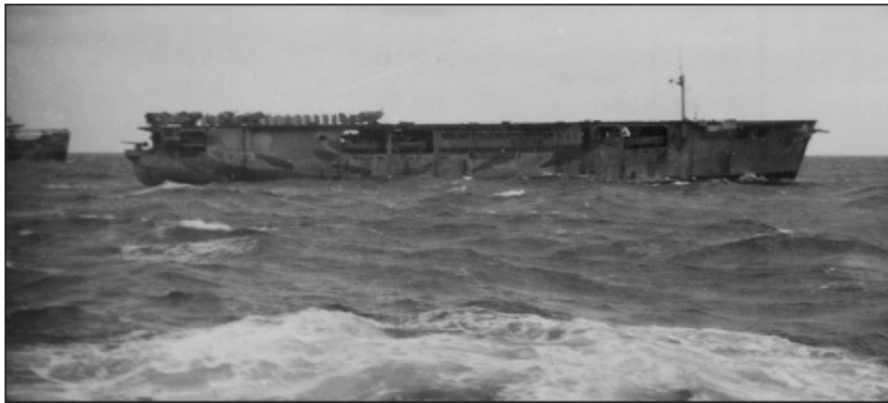
Audacity seen from the starboard beam, with a CAM-Ship in the background. The aircraft ranged aft are Martlets of 801 NAS, partly protected against the elements by the windbreaks. (AUTHOR'S COLLECTION)
