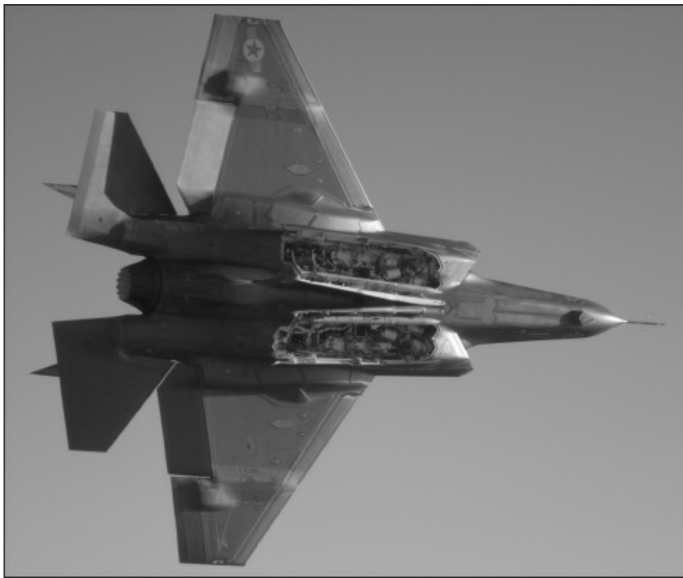
An F-35C Lightning II joint strike fighter in flight, showing its two weapons bays open. (USN)
