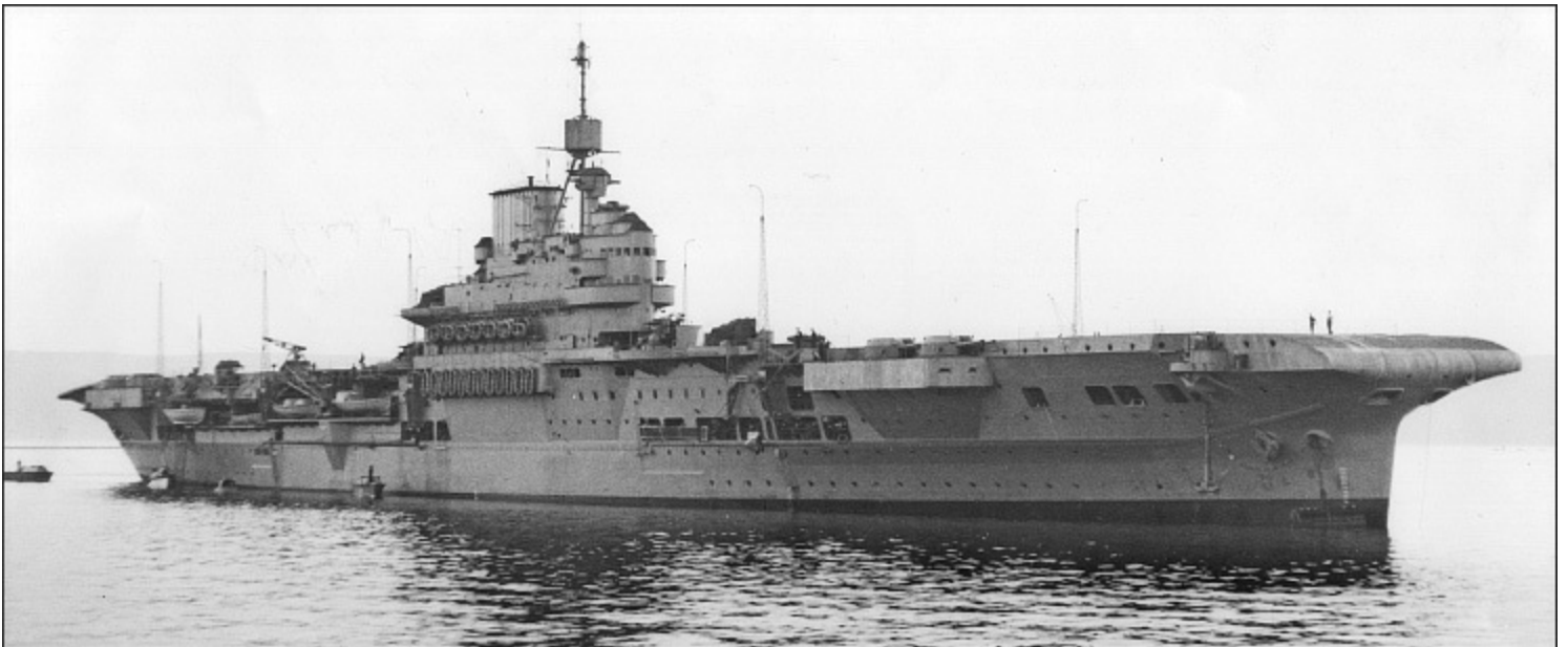
Illustrious' flight deck, showing the narrow areas fore and aft needed to incorporate the 4.5in medium-range-gun mountings. (AUTHOR'S COLLECTION)
