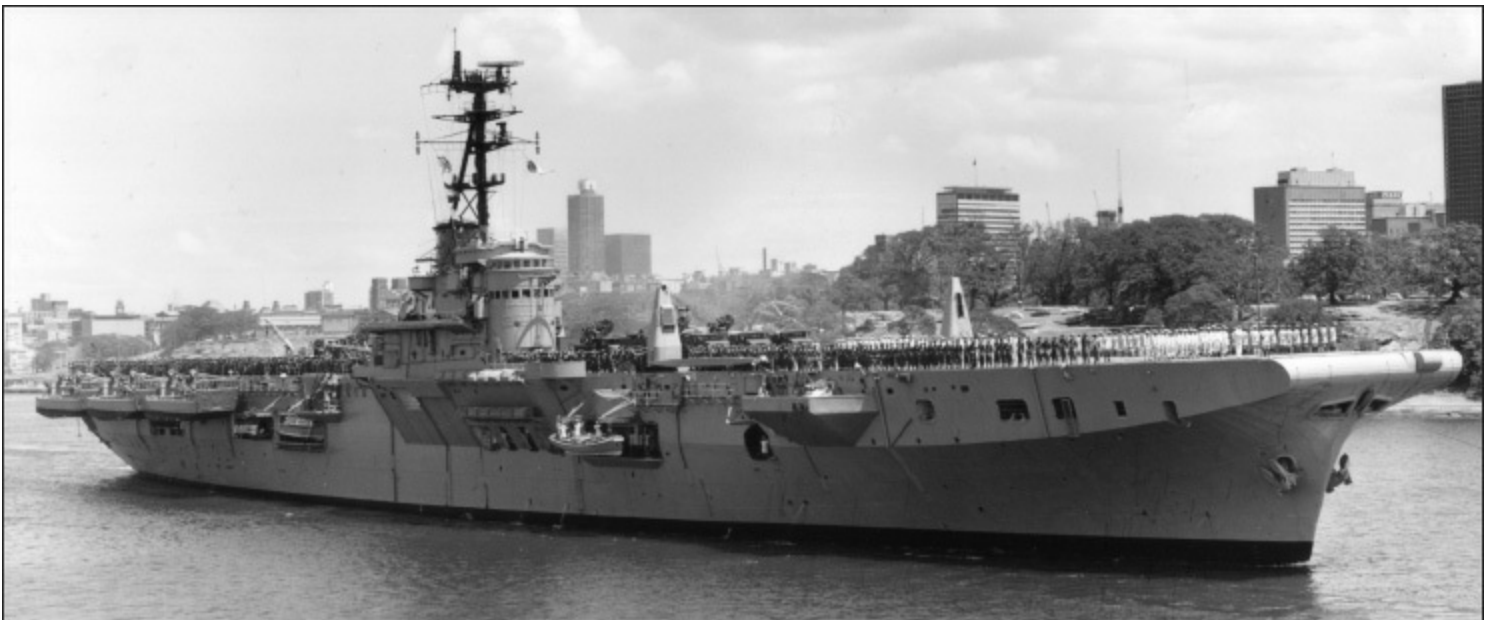
HMAS Sydney after conversion to a fast troop transport, loaded with troops and equipment for Vietnam. Note the two cranes added to the flight deck forward. (RAN)
