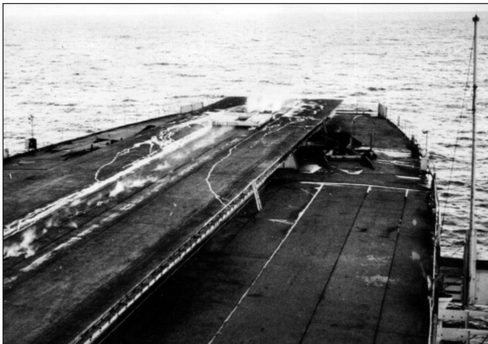
The structure housing the prototype Bxs-1 steam catapult on Perseus during a test with a 'light shot'. The pole mast has an anemometer on top of it to give accurate wind speeds over the deck near the catapult. (AUTHOR'S COLLECTION)
