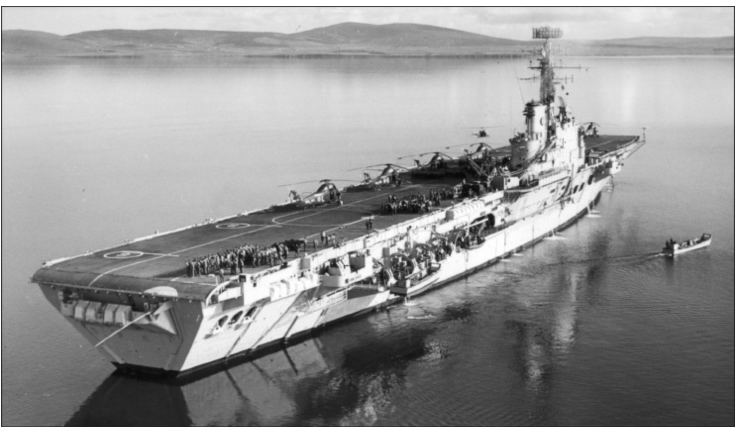
Albion in Scapa Flow during March 1971, clearly showing the landing craft on the starboard side. One is already in the water and the second is being lowered. The Type 965 radar on top of her mast distinguished her from her sister ship Bulwark . (AUTHOR'S COLLECTION)
