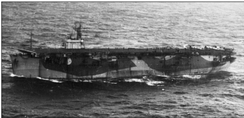
Chaser with Swordfish and Wildcats of 816 NAS ranged aft on 29 February 1944. The H F /D F mast to starboard in Fly 1 is prominent. (AUTHOR'S COLLECTION)
