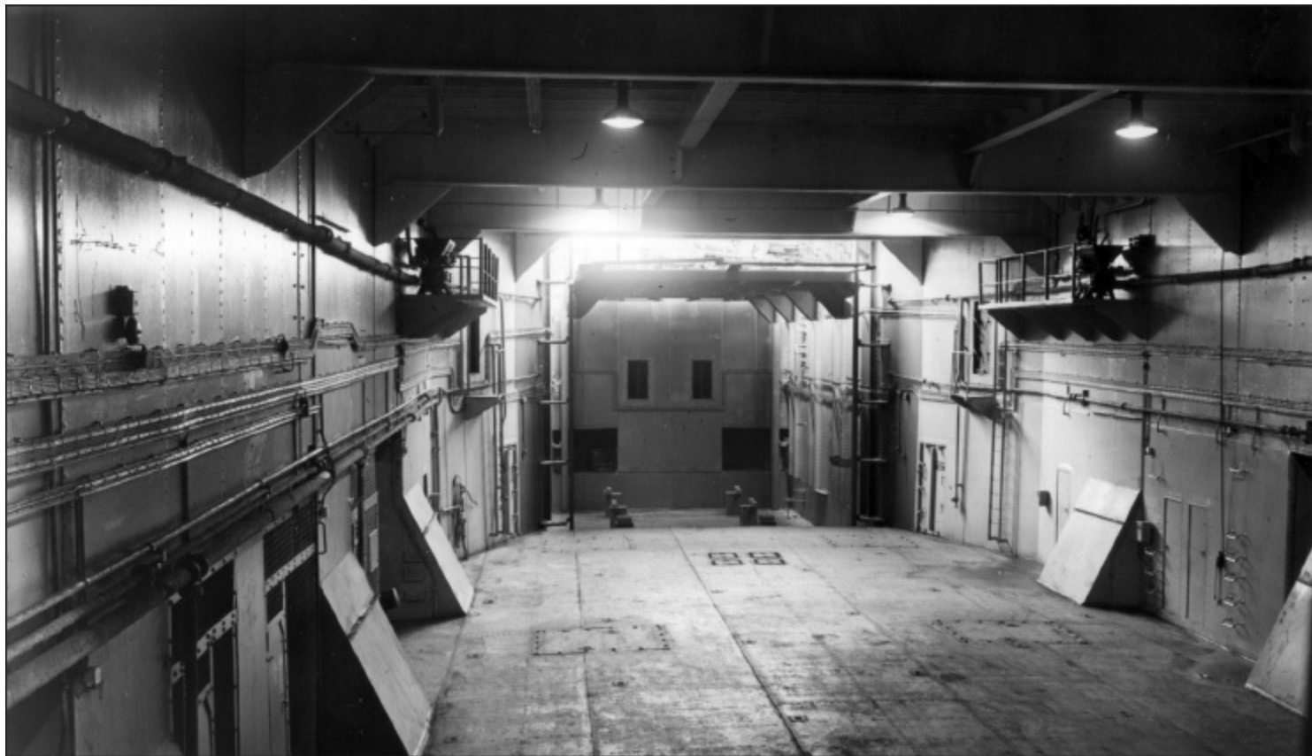
A view of Empire MacAlpine 's hangar from forward to aft, showing the lift platform stopped just below flight-deck level to provide light. The main hangar lighting was quite dim. (AUTHOR'S COLLECTION)
