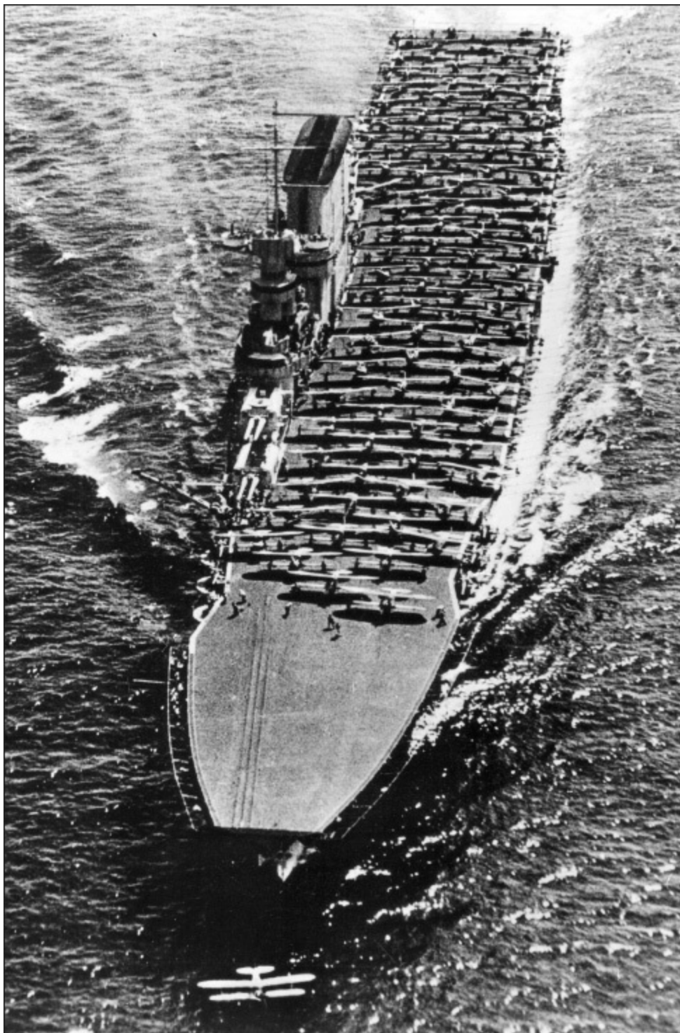
The USS Lexington , Cv-2, as built, showing her capability to launch an enormous deck-load strike. The first aircraft out of the range has just got airborne, and the two twin 8in turrets are visible forward of the island. The forward two twin 8in gun turrets can be seen before the island. (AUTHOR'S COLLECTION)
