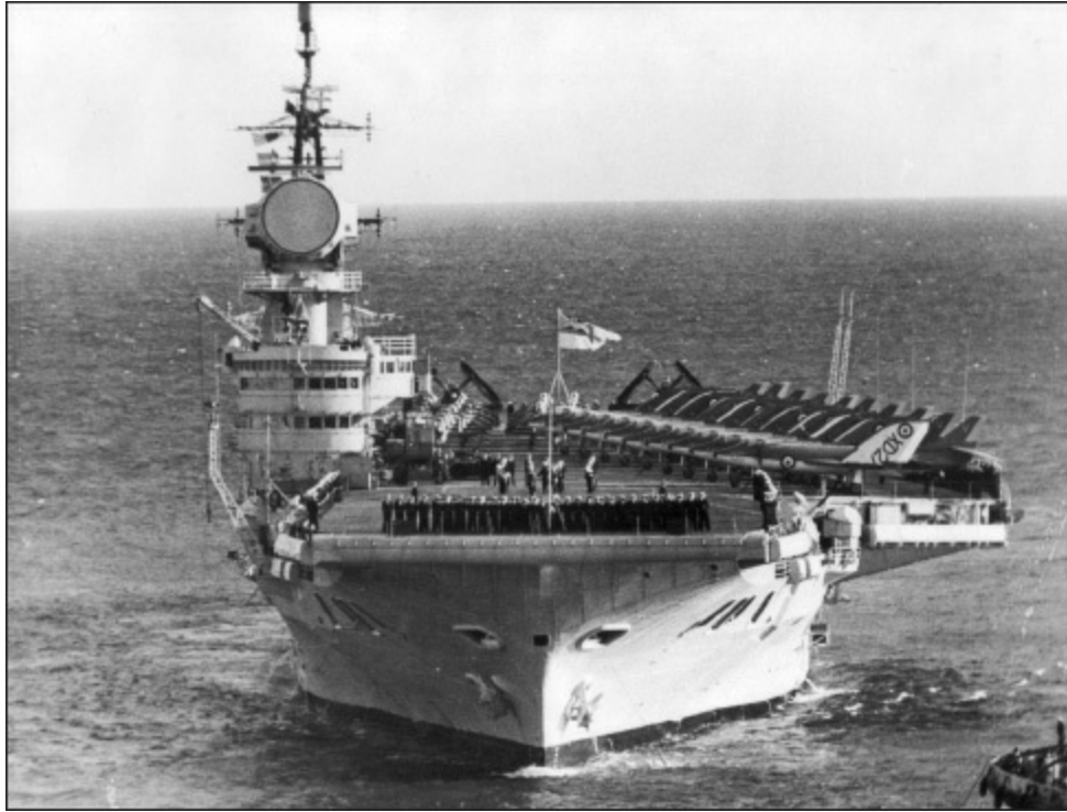
The scale of the new port-side sponson and the Type 984 radar aerial mounted on the island are evident in this photograph, taken as Victorious entered Malta in 1959. On deck are Scimitars, Sea Venoms and Skyraiders. (AUTHOR'S COLLECTION)
