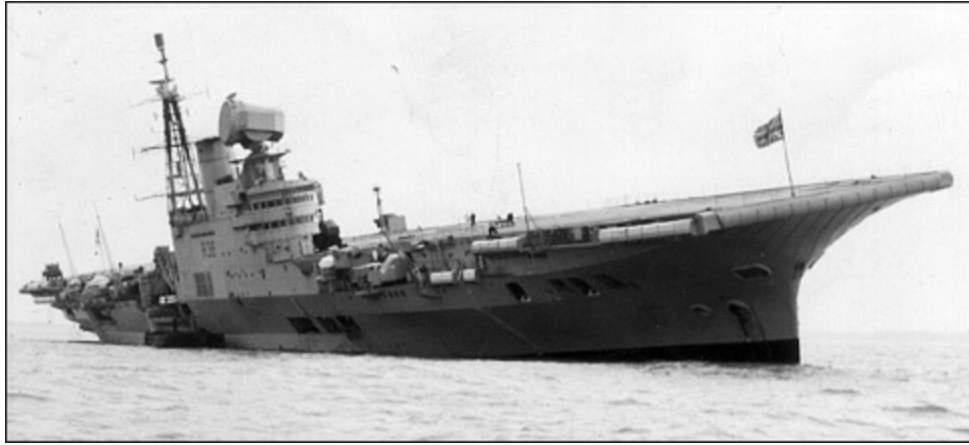
Victorious listed 12 degrees to starboard during her post-reconstruction inclining experiment. (AUTHOR'S COLLECTION)
