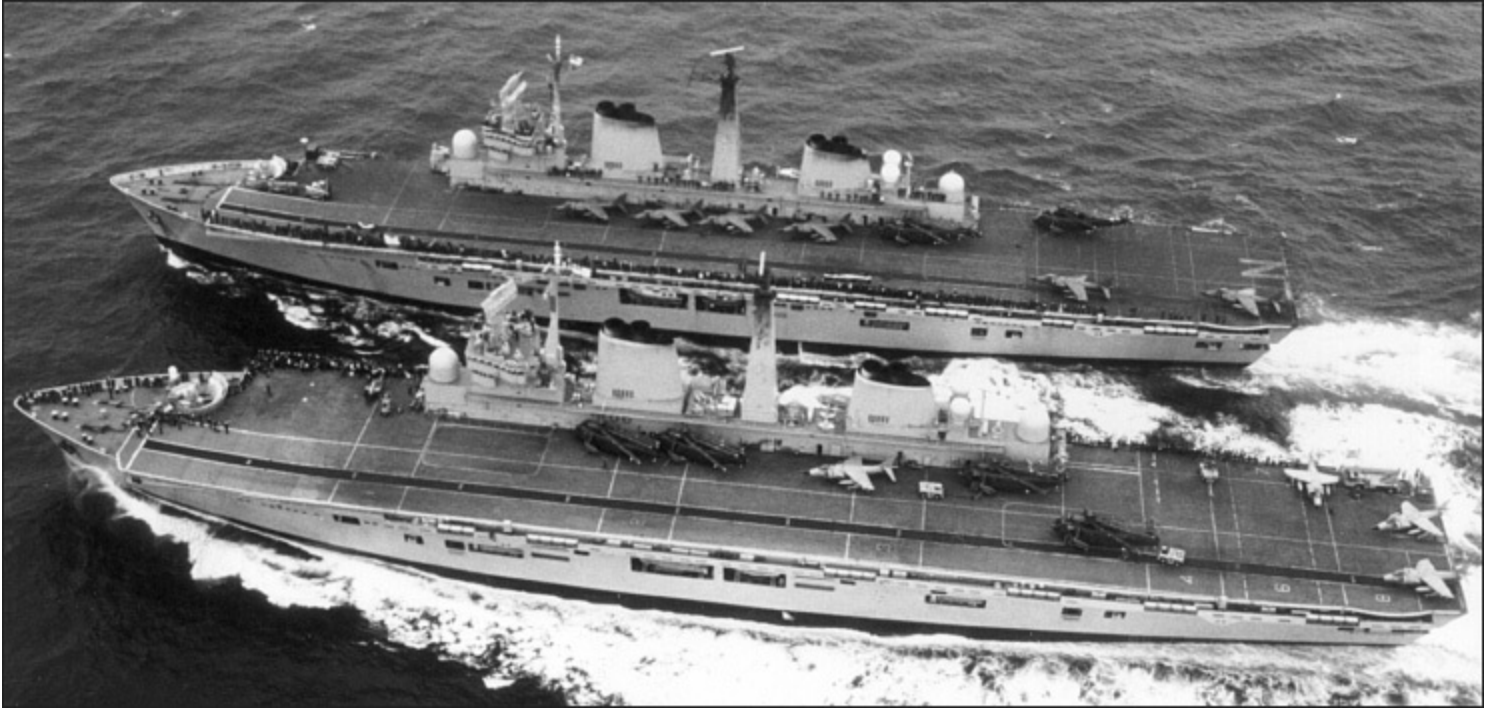
Invincible being relieved by Illustrious , the nearer ship, in the South Atlantic during 1982. The narrowness of the deck is clearly evident; Invincible has four Sea Harriers and a Sea King in the narrow Fly 2 alongside the island. Illustrious has three Sea Kings and a Sea Harrier. The deck markings were designed for their purpose by the author, who ran the flying trials in both ships. They differed from previous designs in having no circles to mark designated landing spots. (AUTHOR'S COLLECTION)
