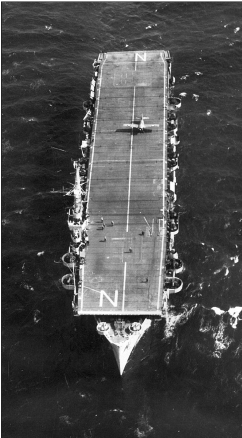
A Wildcat lands on Puncher . Both barriers are down, and marshallers are guiding the aircraft forward into Fly 1. (AUTHOR'S COLLECTION)
