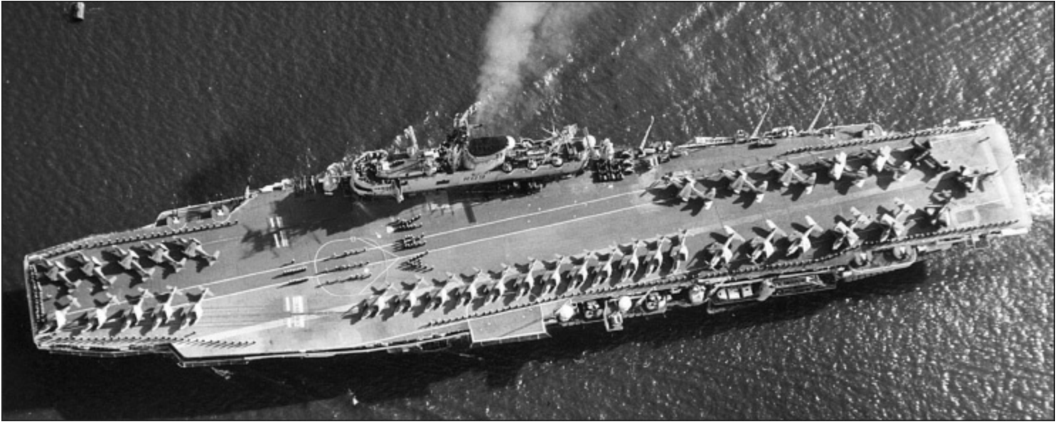
Ark Royal in May 1957. She still has the side lift, but the port 4.5in gun turrets have been removed and the flight deck has been extended over their sponson. Aircraft on deck include Sea Hawks, Wyverns, Gannets and Skyraiders. Note the sailors forming 'ARK' just aft of the forward lift. (AUTHOR'S COLLECTION)
