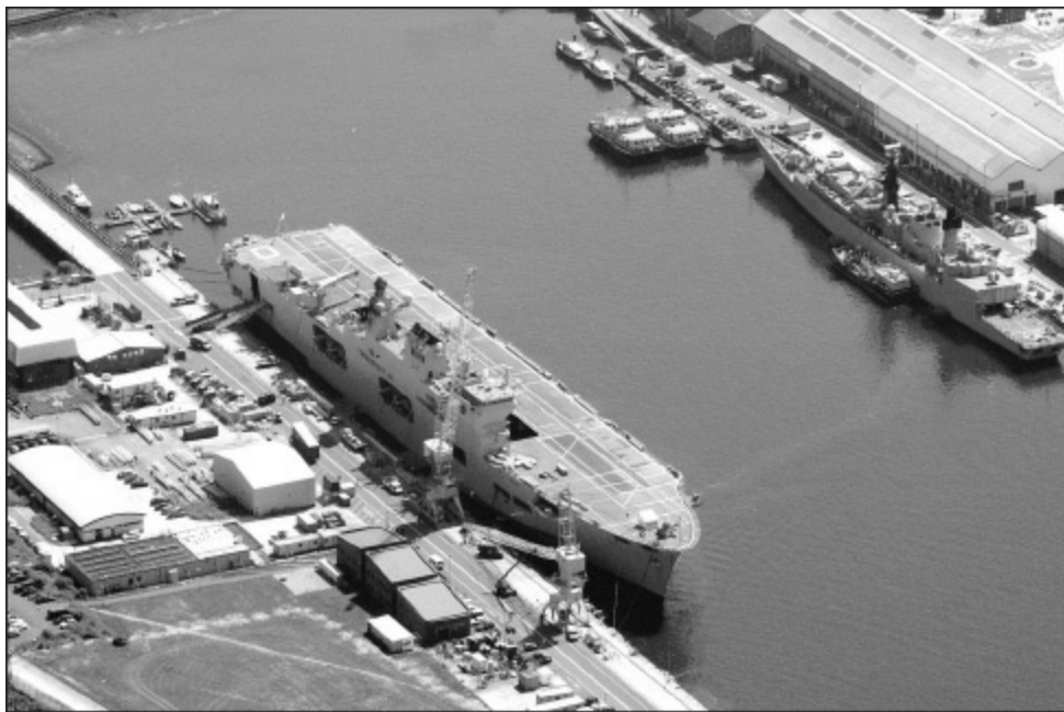
Ocean alongside her normal berth in Devonport Naval Base. The large openings in the ship's side are where the assault landing craft are secured to davits; there are a further two on the port side. They are usually lowered while in harbour to allow their crews to train with other RM assault units. (CROWN COPYRIGHT/MOD 2012)
