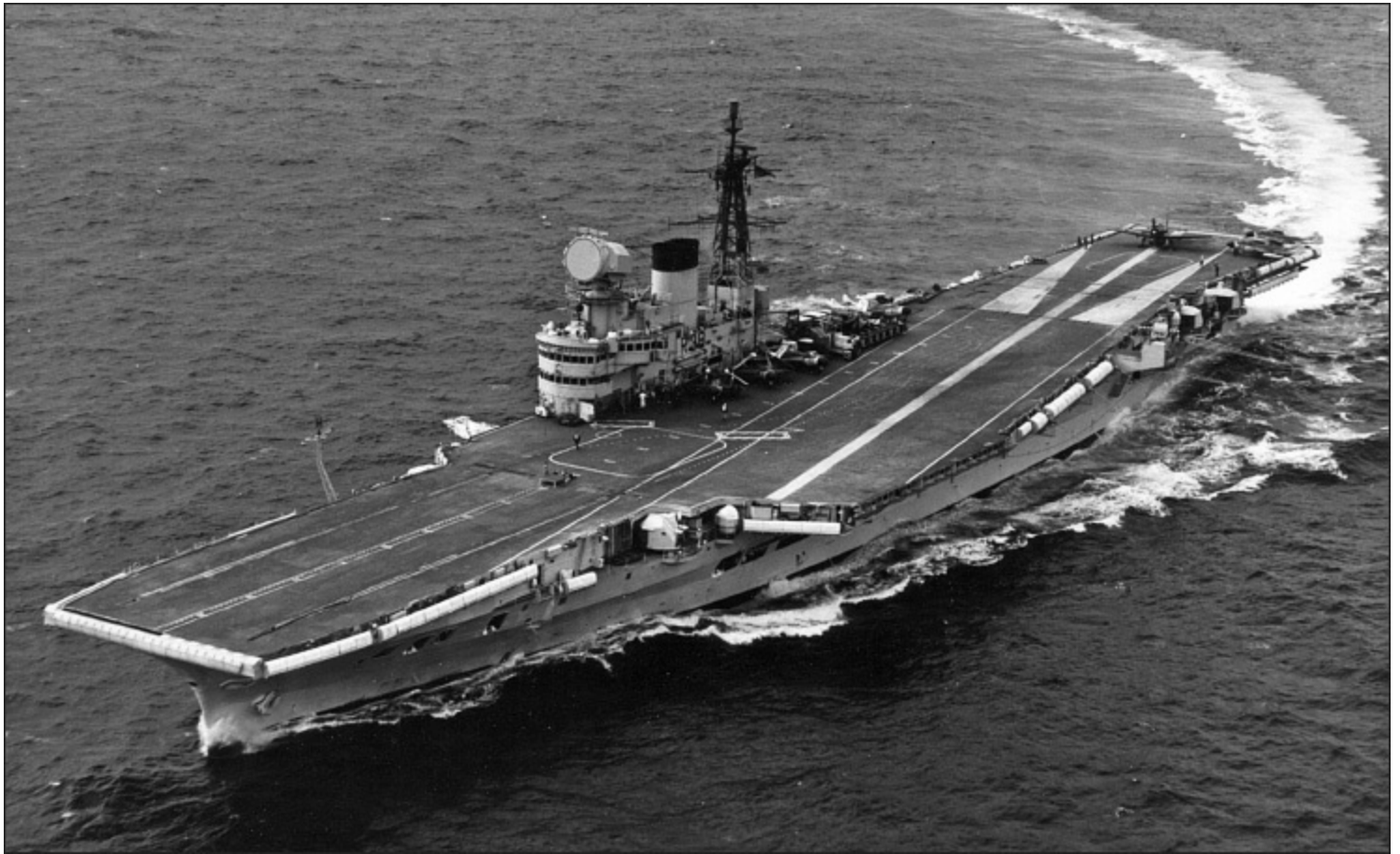
Victorious in 1959. The aircraft by the island in Fly-2 are Sea Venoms, and more Sea Venoms and a Skyraider are ranged aft. The latter is about to make an unassisted free take-off from the angled deck. (AUTHOR'S COLLECTION)
