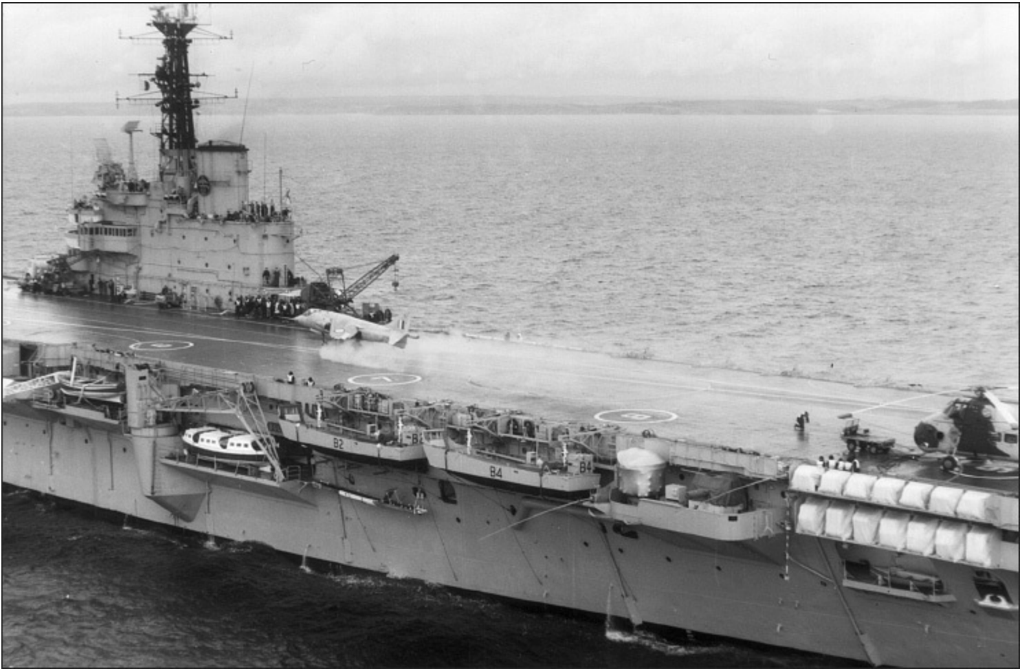
A P.1127 carries out a running take-off from Bulwark in 1966. The jet blast has no effect on the Wessex helicopter parked on 9 spot with its blades spread. (AUTHOR'S COLLECTION)
