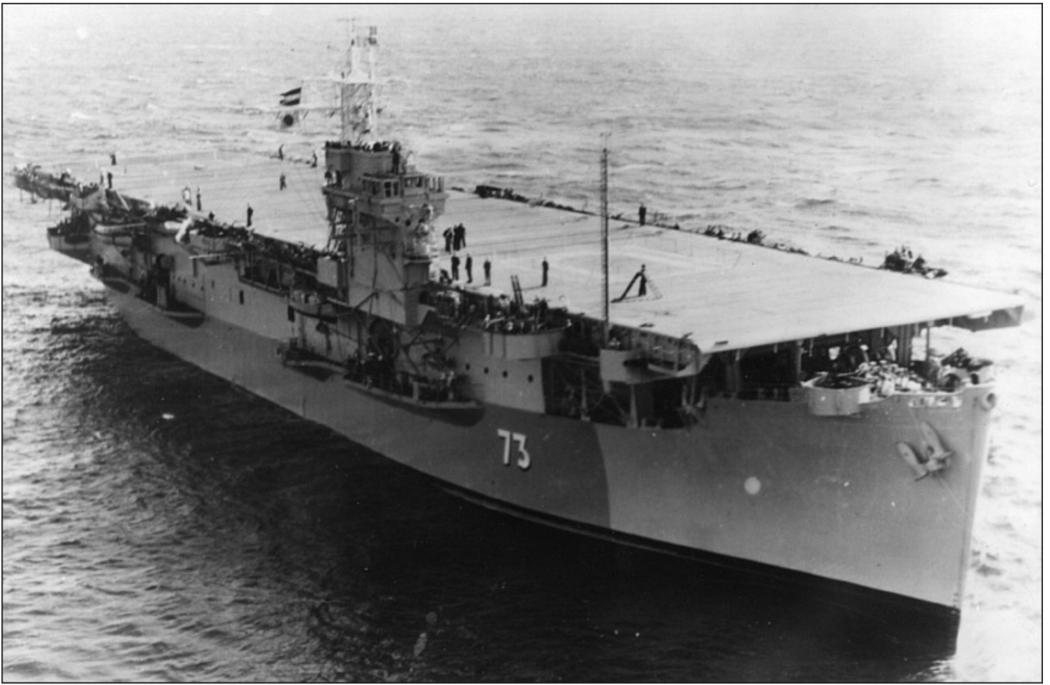
Her improved bridge structure is evident in this photograph of Pursuer , taken in July 1945 after her refit in Durban. (AUTHOR'S COLLECTION)
