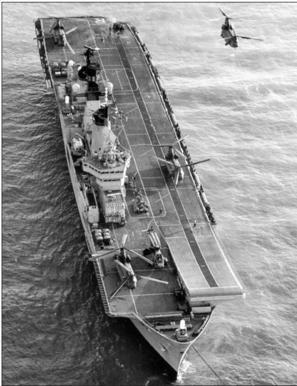
Ark Royal operating RAF Chinook helicopters in the Northern Gulf during the Second Gulf War in 2003. The extended Fly parking area allows a Chinook and Sea King ASaC.7 to be parked in it comfortably. Note the amount of space taken up by the Chinooks, which do not have folding rotor blades. (AUTHOR'S COLLECTION)
