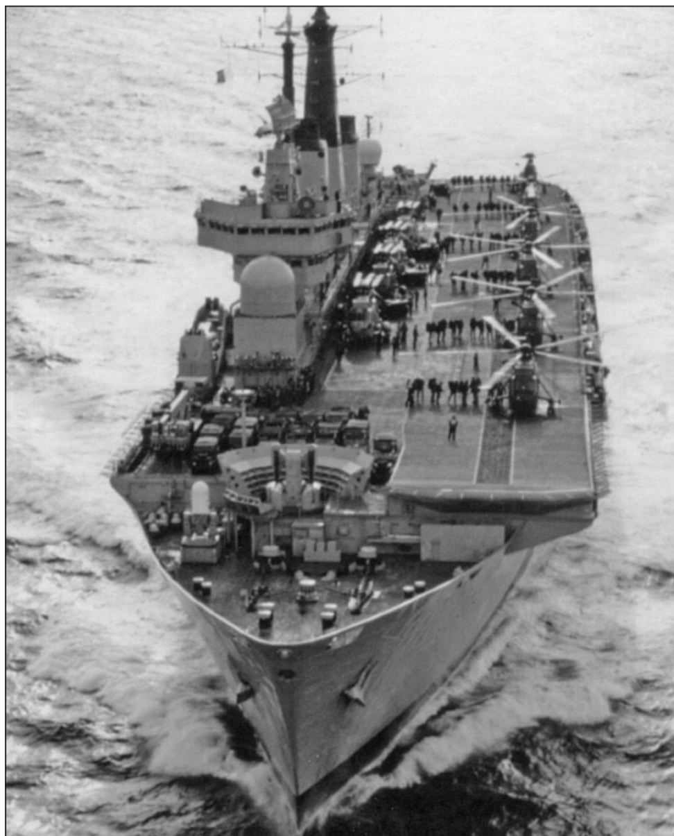
Illustrious operating in the LPH role with marines moving out to five Sea Kings running on spots. A further four Sea Kings in Fly 2 have tractors attached, ready to pull them out on to spots from which they will be launched as a second assault wave. The small parking space in Fly 1 has RM Land Rovers stowed in it. (AUTHOR'S COLLECTION)
