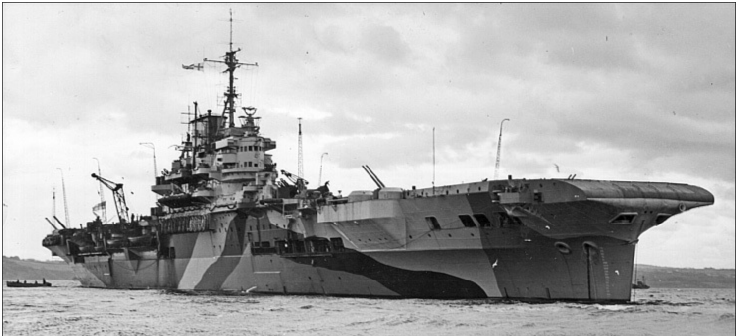
Formidable at anchor after her U's refit in 1941, flying a church pennant to show a religious service is taking place. A 'Y' homing beacon on a telescopic mast attached to the funnel has replaced the Type 72, but the forward round-down still limits the amount of deck space available for parking in Fly 1. (AUTHOR'S COLLECTION)
