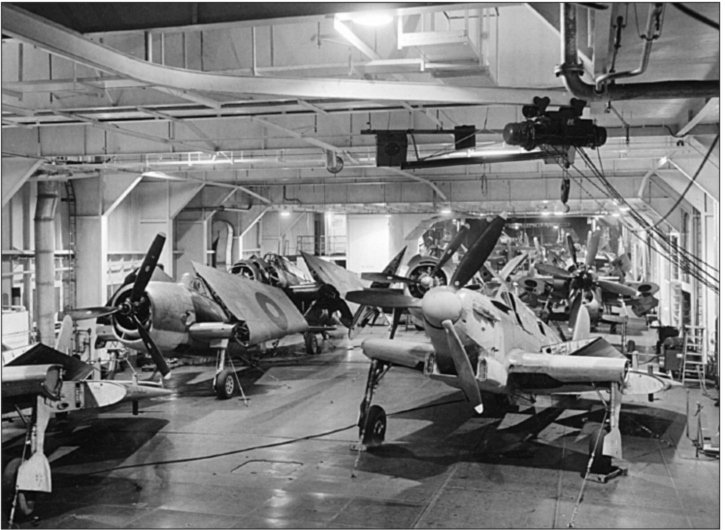
A Hellcat, Fulmars, Avengers and Barracudas in Ravager's hangar while she operated as a deck-landing training carrier in 1945. The overhead hoist system was used for the removal and replacement of heavy components. (AUTHOR'S COLLECTION)
