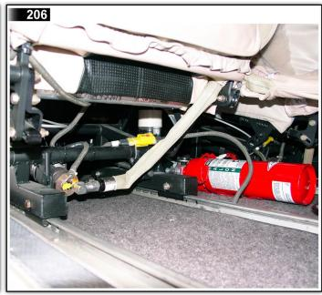
Inflatable restraints are located under the crew seats on each aircraft.
