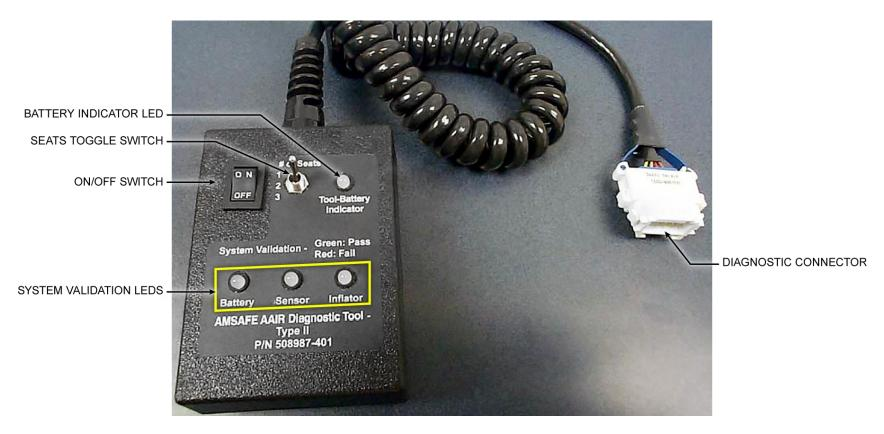
The AmSafe Seat belt Airbag diagnostic check provides a system functional analysis of the AmSafe Seatbelt Airbag circuits as a whole. Fault isolation of the systems components is accomplished by replace-and-retest method.
