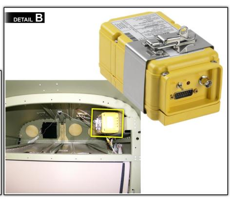
The Artex ME406 Emergency Locator Transmitter (ELT) system includes an ELT unit, an integral battery pack, warning buzzer, internal G-switch, antenna, remote switch, cable assembly, and antenna coaxial cable.
