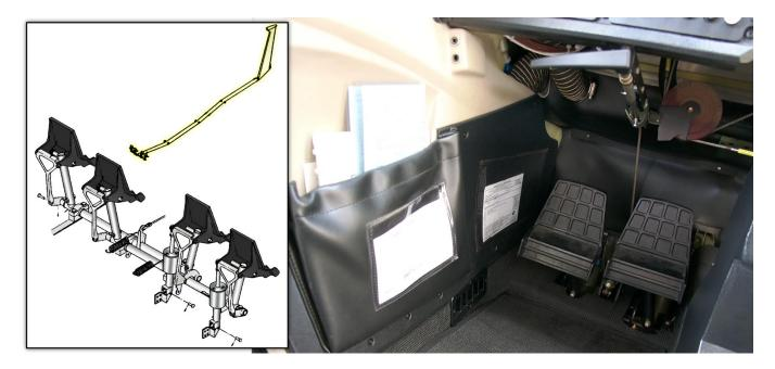
Rudder control operates using conventional rudder pedals that also controls nose wheel steering.
