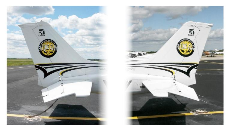
The elevators operate by power transmitted through forward and aft movement of the control yoke. A manually operated elevator trim system is on this airplane. To trim the elevation of the aircraft using the elevator trim tab, rotate the vertically mounted trim control wheel on the center pedestal. Forward rotation of the trim wheel will trim nose down, aft rotation will trim nose up.
