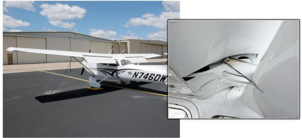
necessary flap setting, the attached cam activates one of the micro-switches, and that activates the flap motor.
