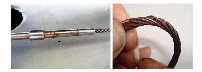
For IN-DEPTH explanations of cable wire breakage and corrosion limits, refer to the flight control system maintenance practices maintenance manual.
