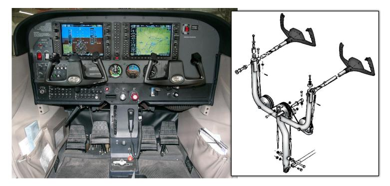
The ailerons receive input from the pilot or copilot control wheel through a series of sprockets, chains, pulleys, cables, bell cranks, and pushrods.
