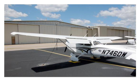
The Fowler-type wing flaps, are extended or retracted by positioning the wing flap control lever on the instrument panel to the desired flap deflection position.
