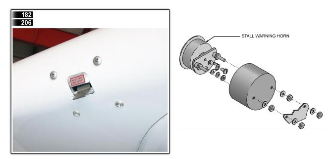
182 / 206 are the same - The stall warning system includes a stall warning horn and stall detector.
