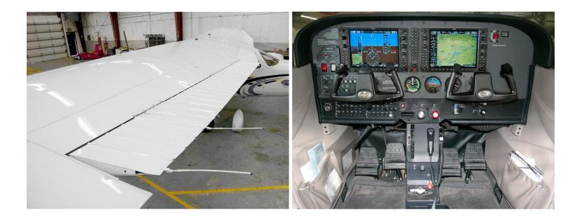
The ailerons receive input from the pilot or copilot control wheel through a series of sprockets, chains, pulleys, cables, bell cranks, and pushrods.
