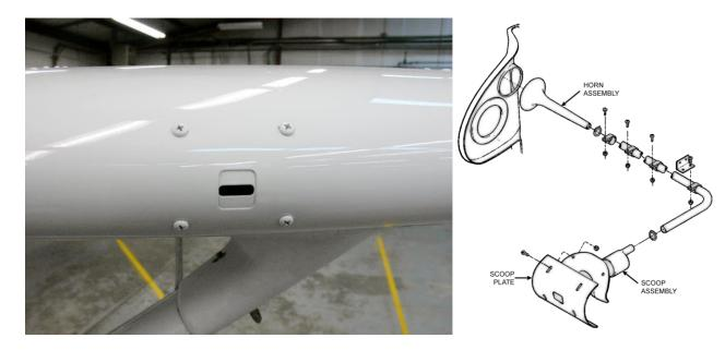
The stall warning system includes a stall warning horn and a scoop assembly.
