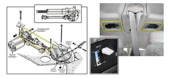
The flap follow up and indicating system consists of a sheathed cable assembly, pointers and micro switches.
