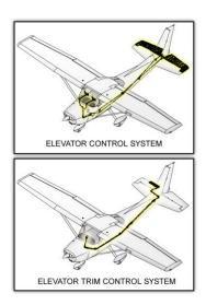
a bearing point for the travel stop bolts. A trim tab mounts to the right elevator.
