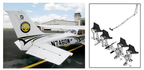
extension, which contains a balance weight. Rudder control operates using conventional rudder pedals that also controls nose wheel steering.
