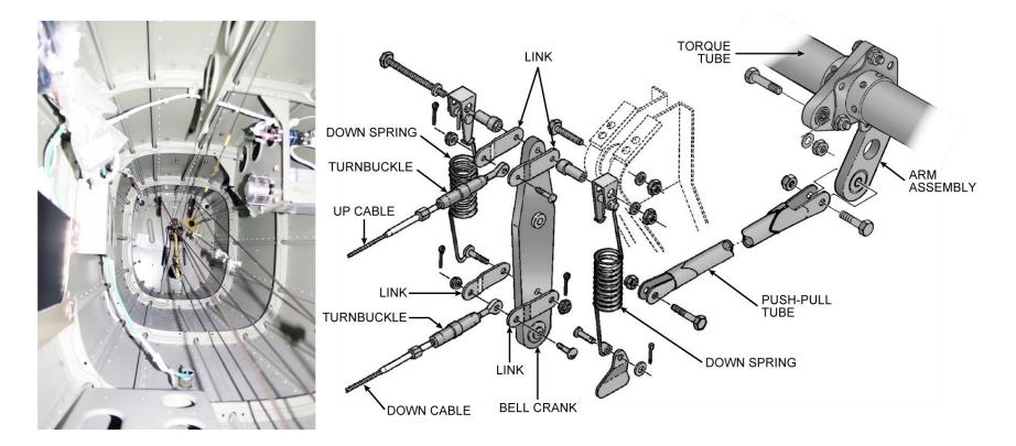
It is very important to lubricate springs, linkage, and cables periodically according to the maintenance manual. If dry and not lubricated, there will be a popping sound when ailerons move.
