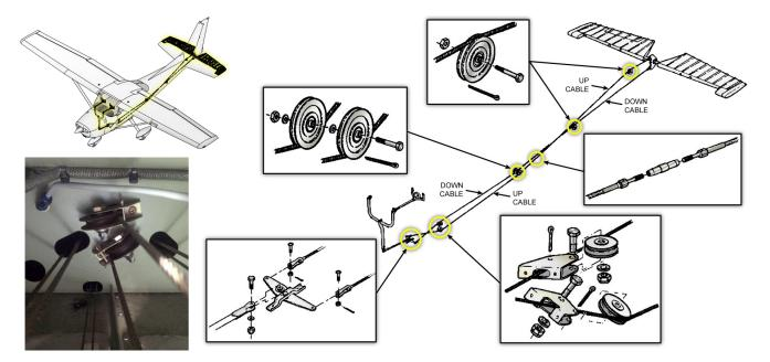
The elevators operate by power transmitted through forward and aft movement of the control yoke.
