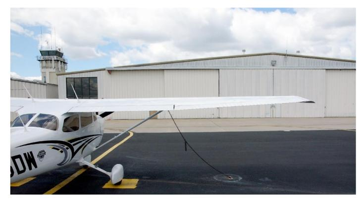
The airplane's flight control system consists of conventional aileron, rudder, and elevator control surfaces. The control surfaces operate by cables and mechanical linkage using a control wheel for the ailerons and elevator, and rudder/brake pedals for the rudder. The first flight control surface we will discuss is the ailerons. The ailerons receive input from the pilot or copilot control wheel through a series of sprockets, chains, pulleys, cables, bell cranks, and pushrods.
