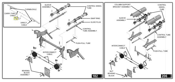
the control wheel tube. Attached to the square tube is a quadrant that operates the aileron system. The two control wheels control the aileron system. The interconnect cables, turnbuckle, and adjustment terminals give synchronized control to the two control wheels. The forward end of the square control tube is in a bearing block on the firewall. It rotates with the control wheel and does not move in a fore-and-aft direction.
