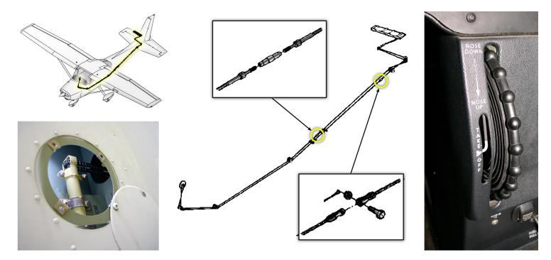
The trim wheel in the pedestal controls the elevator trim tab on the right elevator.
