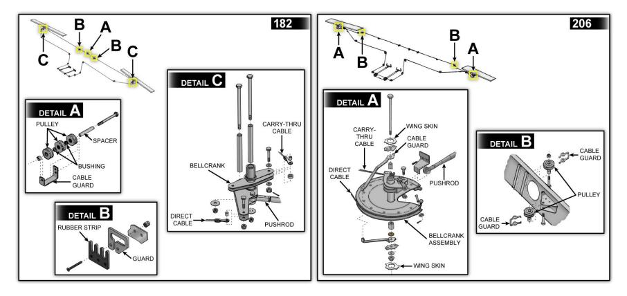
Components for 206 aircraft are designed differently but operate the same, also the mechanical components are built stronger.
