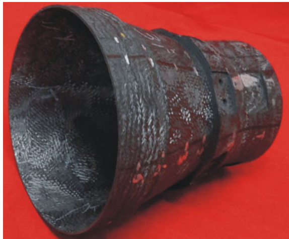
Fig. 15.7 A typical C/C composite nozzle test article
