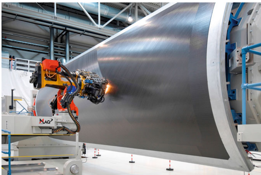
Fig. 14.7 Automated tape laying: CFRP tape layers being placed on the lay-up tool for an Airbus A350 upper shell fuselage skin section: Premium AEROTEC, Nordenham, Germany
