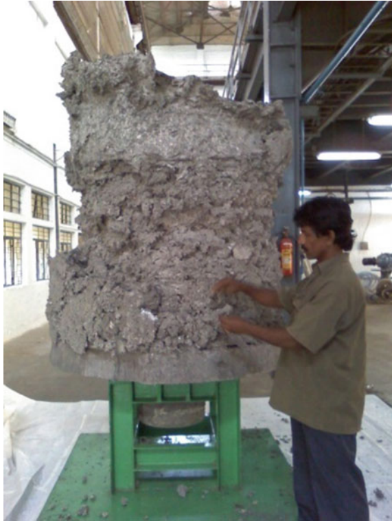
Fig. 4.4 Titanium sponge cake (weight about 3500 kg) produced at the DMRL technology demonstration plant
