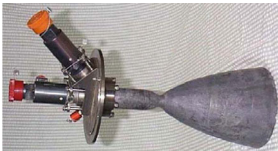
Fig. 15.13 Typical C/SiC thruster test articles
