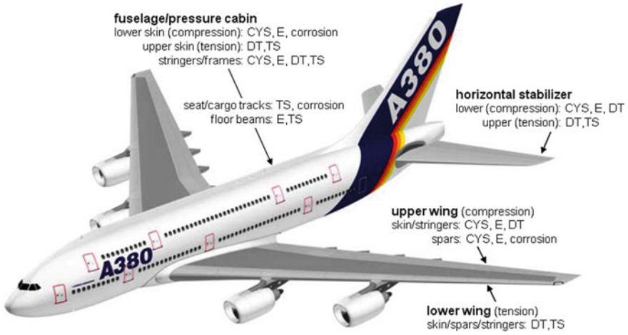
Fig. 3.1 Engineering property requirements for a transport aircraft. See the text for the abbreviations [1]
