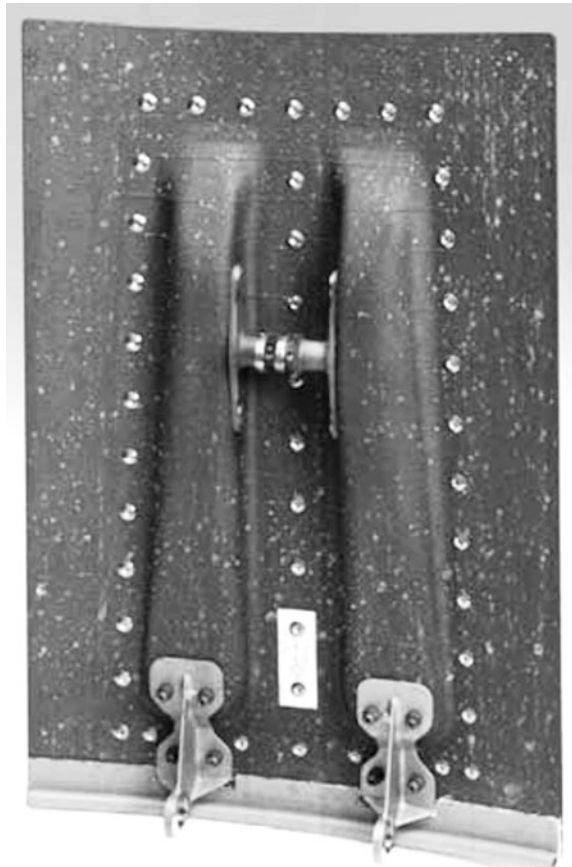
Fig. 16.9 C-SiC composites for thermal protection systems (TPS)
