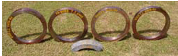
Fig. 6.13 Aeroengine high pressure compressor rings made of Titan 29A
