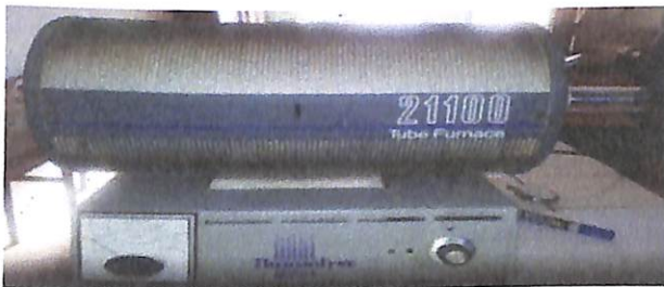
Fig. 4. Picture of Thermolyne Tubular Furnace (21100 Furnace Tube)
