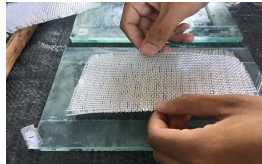
Peletakan Reinforcement serat woven roving
