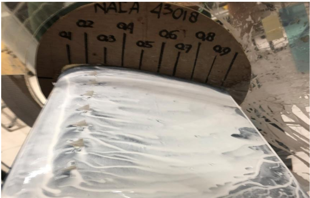
A21.Airfoil VG \alpha = 19^{\circ} , x/c=20\% & RE = 9.6 \times 10^5
