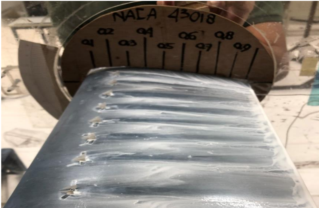
A13. Airfoil VG \alpha = 2^\circ , x/c=20\% & RE = 9.6 \times 10^5
