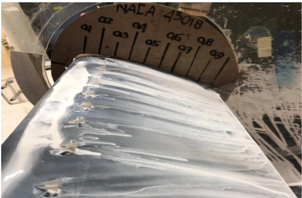
A20. Airfoil VG \alpha = 16^\circ , x/c=20\% & RE = 9.6 \times 10^5
