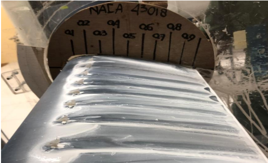
A17. Airfoil VG \alpha = 10^\circ , x/c=20\% & RE = 9.6 \times 10^5
