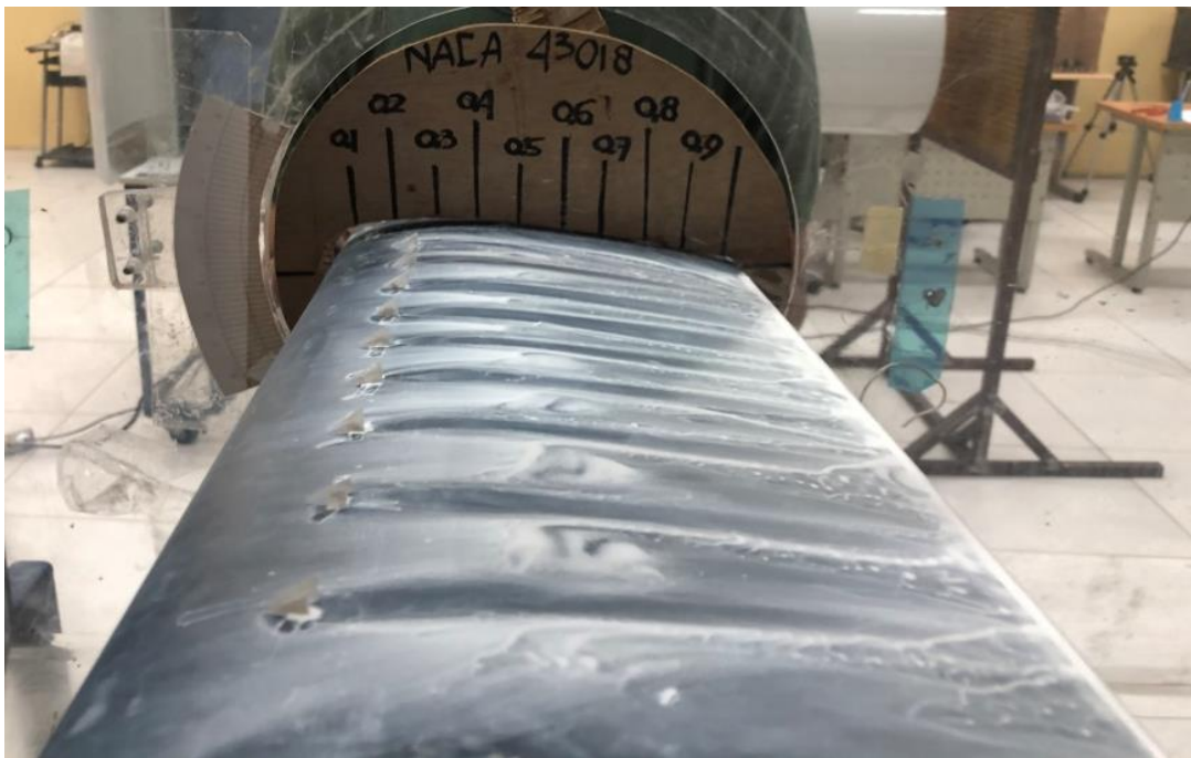
A12. Airfoil VG \alpha = 0^\circ , x/c=20\% & RE = 9.6 \times 10^5
