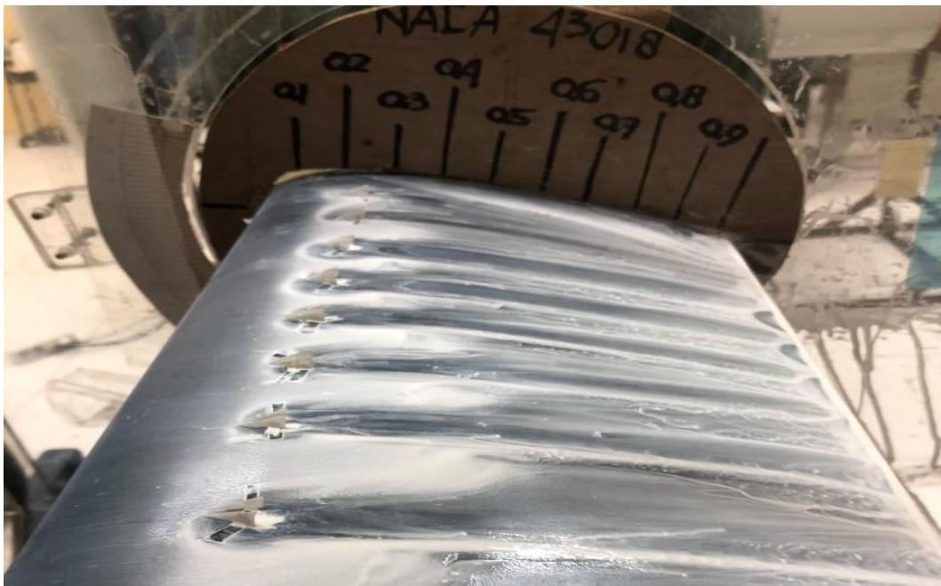
A16. Airfoil VG \alpha = 8^\circ , x/c=20\% & RE = 9.6 \times 10^5
