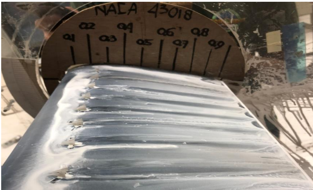
A18. Airfoil VG \alpha = 12^\circ , x/c=20\% & RE = 9.6 \times 10^5
