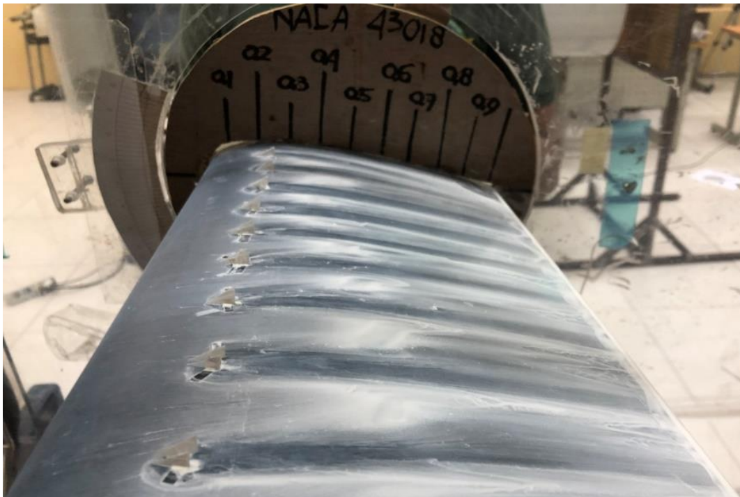
A14. Airfoil VG \alpha = 4^\circ , x/c=20\% & RE = 9.6 \times 10^5
