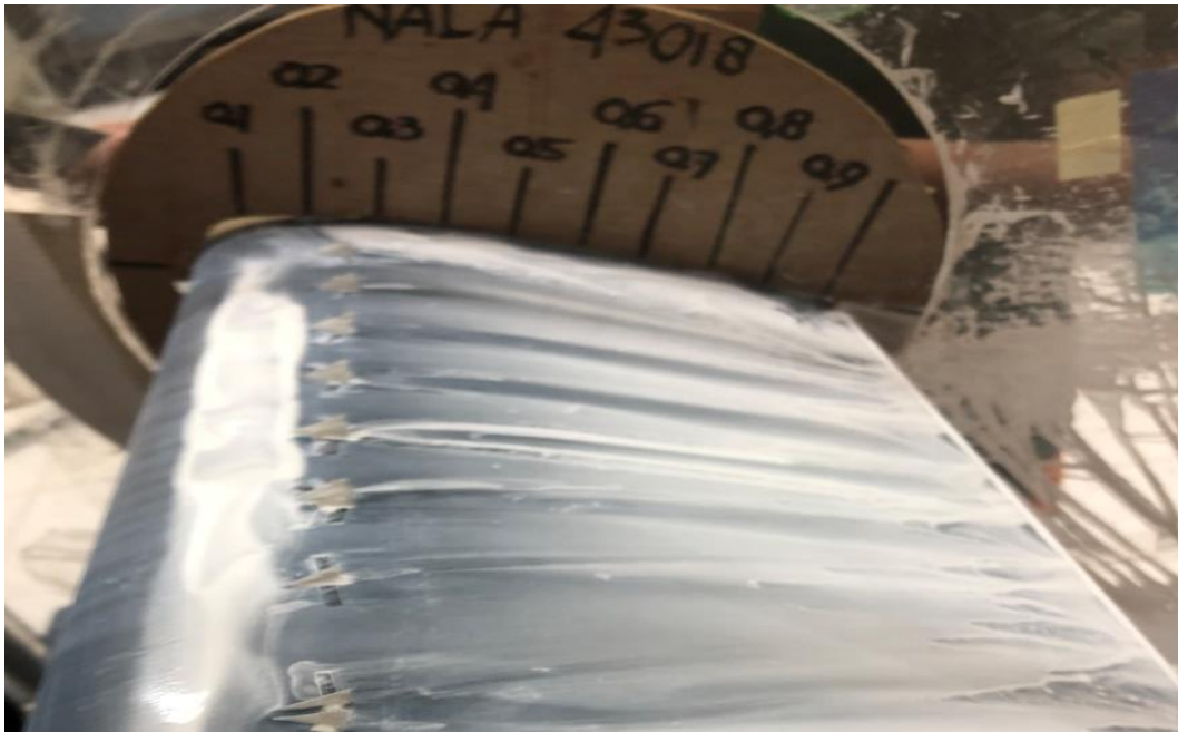
A19. Airfoil VG \alpha = 15^\circ , x/c=20\% & RE = 9.6 \times 10^5
