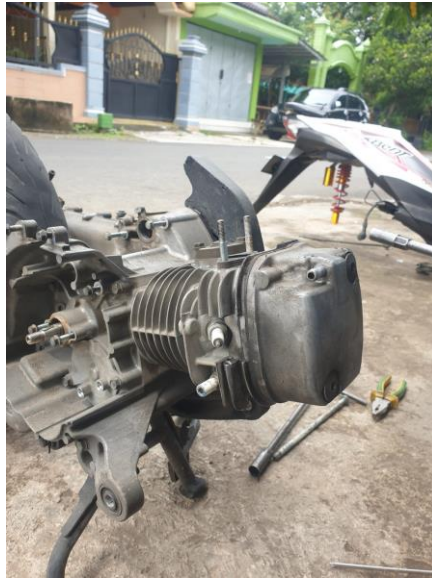
Proses penggantian piston head
