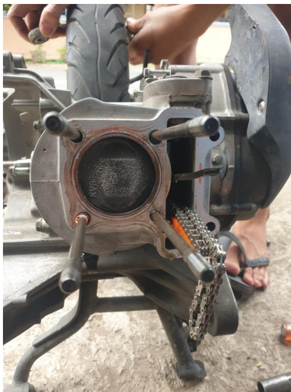
Proses penggantian piston head
