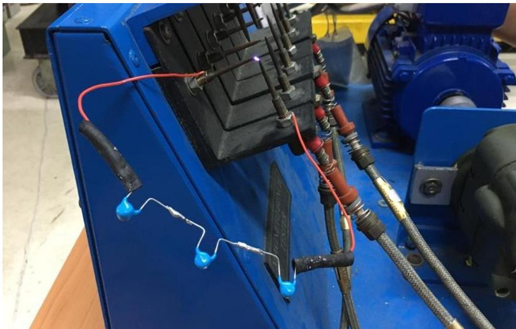
Lampiran 7 Pemasangan Capacitor Pada Magneto Bench Tester
