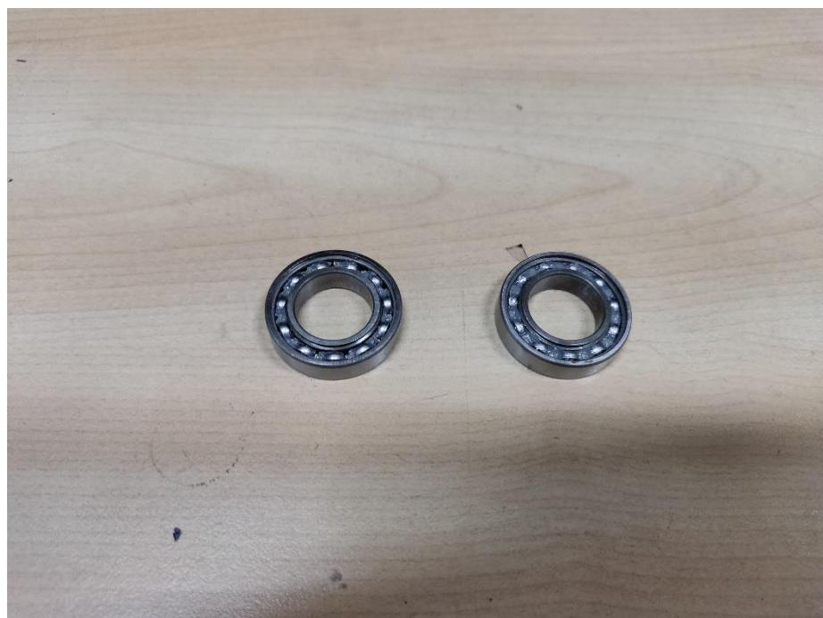
A2. Deep Groove Ball Bearing Material Steel Berdimensi 17×30×7mm
