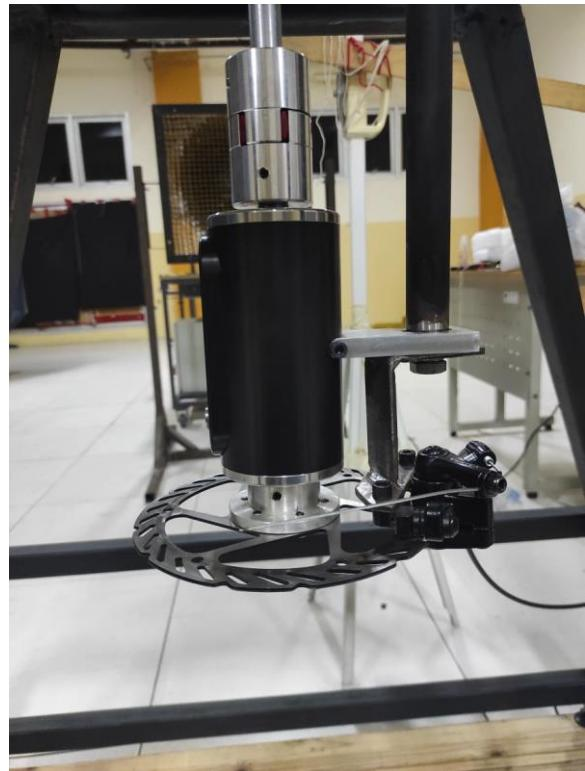
A7. Datum M425 Torque Transducer
