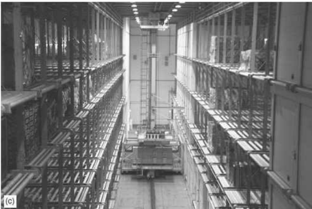
FIGURE 10.7 (a) Air cargo interior—low-technology freight terminal. (b) INFRAERO cargo terminal, São Paulo International Airport. (Courtesy of INFRAERO, Brazil.) (c) An ETV. (Courtesy of INFRAERO, Brazil.)
