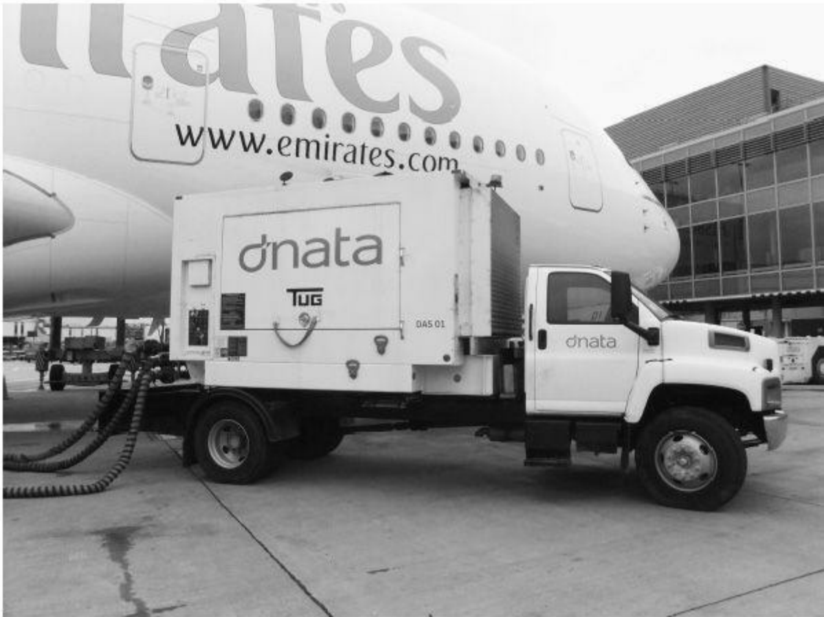
FIGURE 6.9 Mobile apron engine air-start vehicle.
