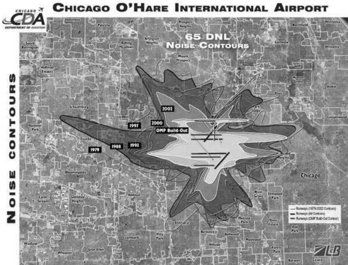
FIGURE 3.10 Historic and predicted future noise contours at Chicago O’Hare International Airport. (Courtesy: Chicago O’Hare International Airport.)
