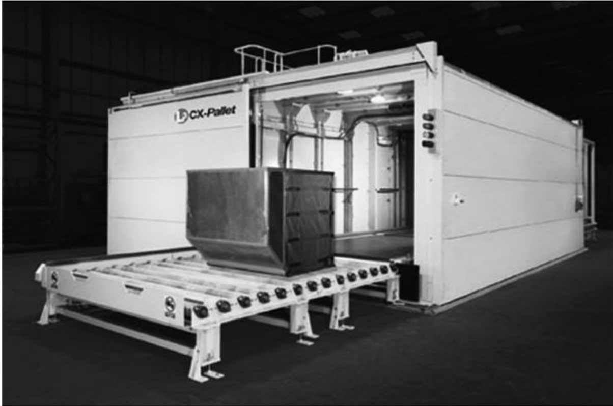
FIGURE 9.11 Freight x-ray machine. (L-3 Security & Detection Systems.)
