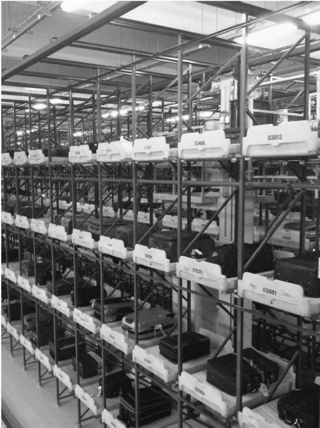
FIGURE 7.14 Crane-served bag store.
