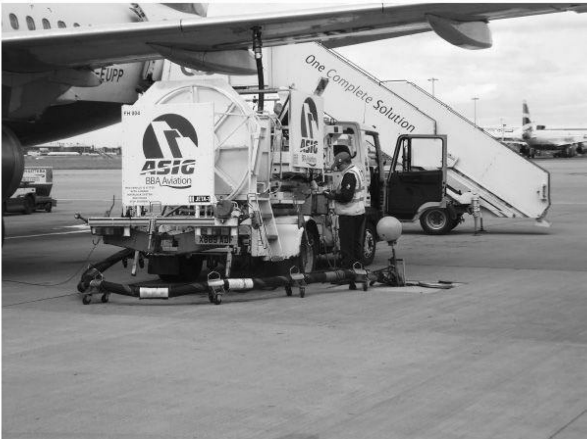
FIGURE 6.12 Mobile aircraft fuel dispenser for fueling from apron hydrant system.
