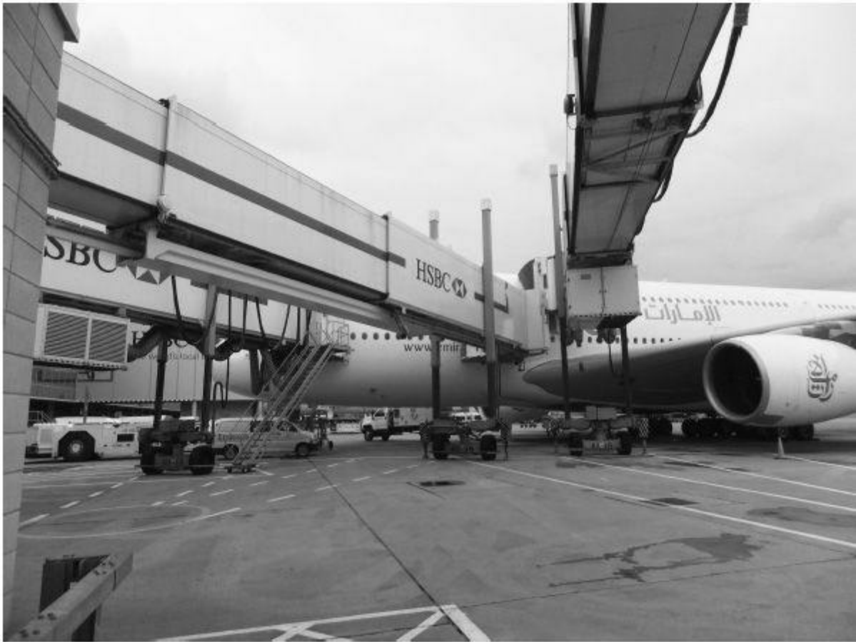
FIGURE 6.5 Three-loading-bridge configuration serving an A380.
