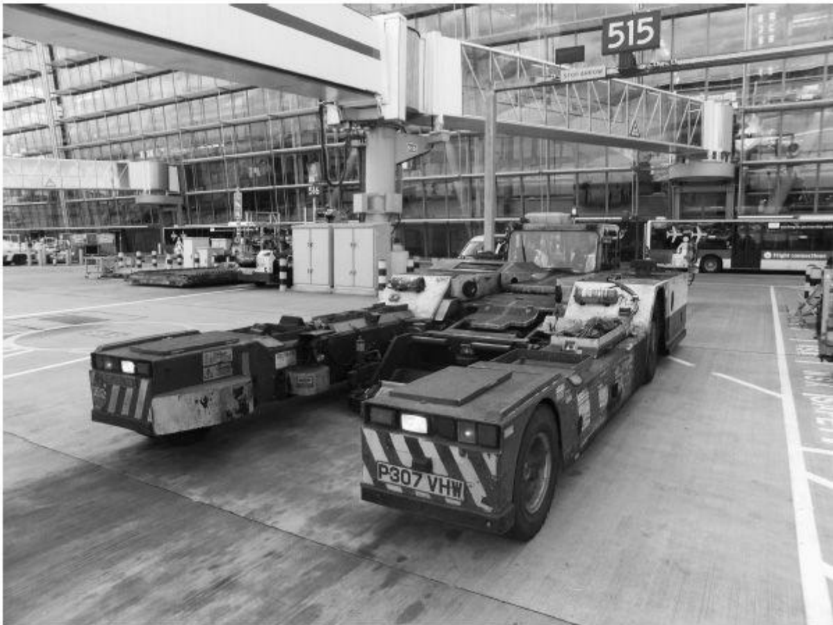
FIGURE 6.10 Aircraft tow tractor.
