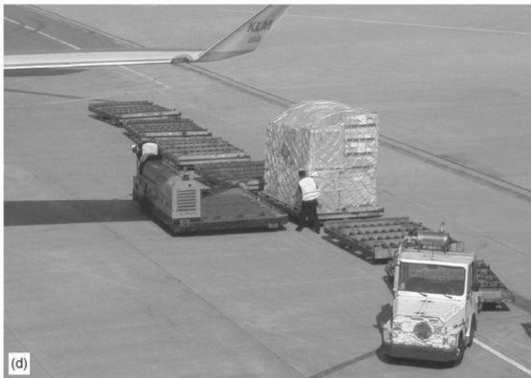
FIGURE 10.10 (a) Upper-deck freight container loader. (b) Lower deck freight container loader (Courtesy: Munich International Airport.) (c) Nose loader for freighter in position. (Courtesy: Chapman Freeborn Air Chartering.) (d) Cargo container transporter.
