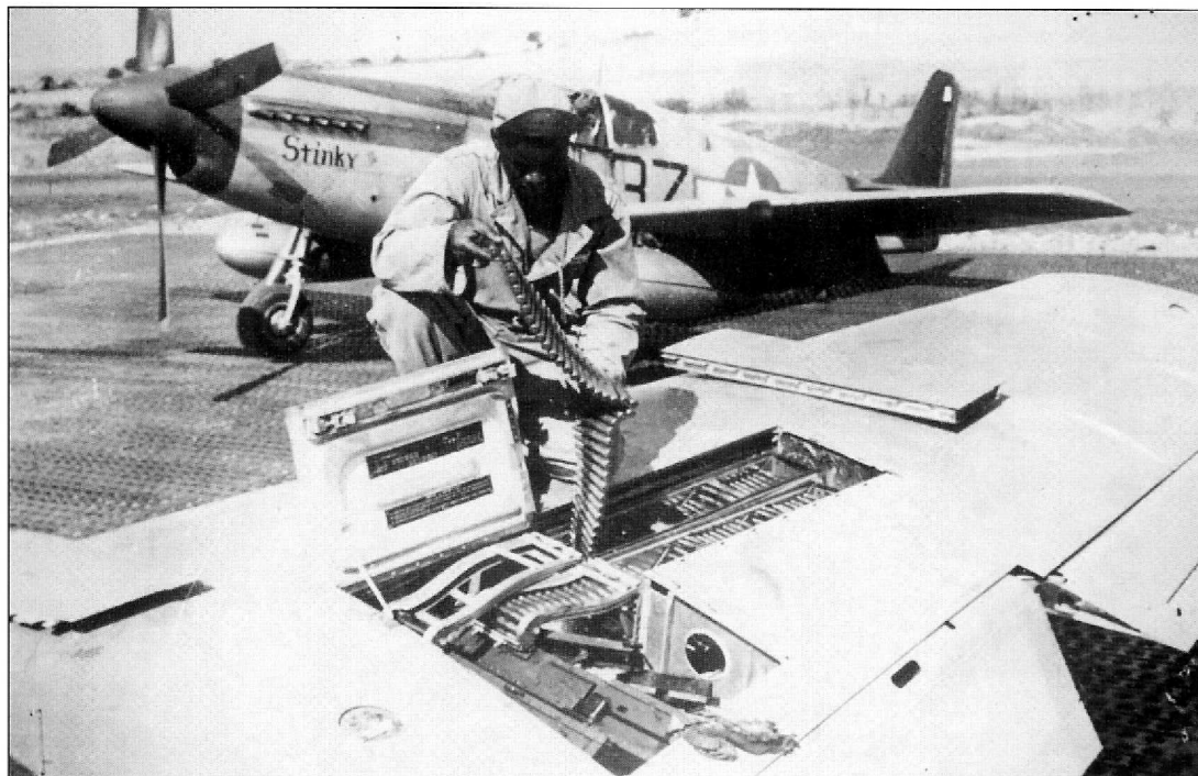
A 100th FS armorer reloads the trays of his B-model Mustang with ammunition at Ramitelli at the height of the airfield strafing campaign in the autumn of 1944 ( National Museum of the USAF )
