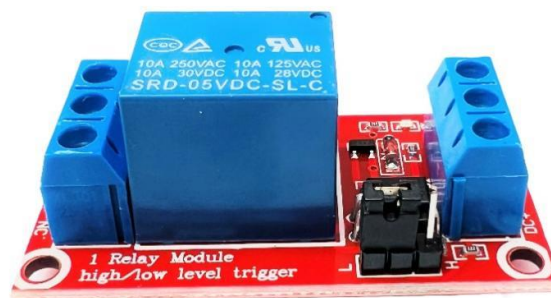
Gambar 2. 7 Relay 1 Chanel Sumber : (Siregar & Reymod, 2015)
