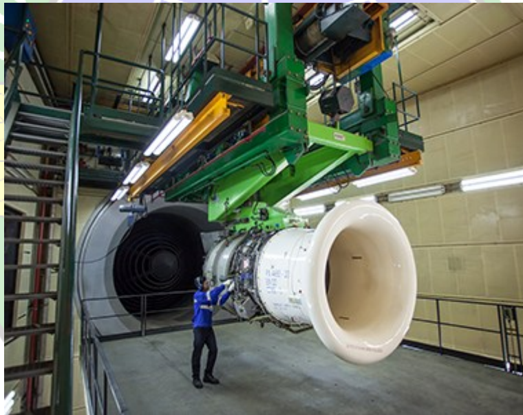
Gambar 2. 5 Engine Test Cell (source: https://short-link.me/17tSm )
