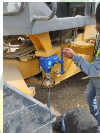
California Bearing Ratio test
