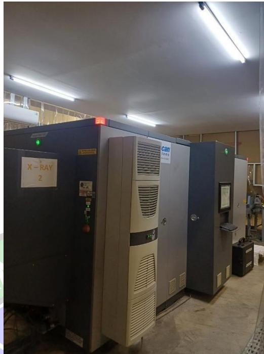
Gambar 3. 19 X-Ray Hold Baggage Screening (HBS) Sumber: Dokumentasi Penulis
