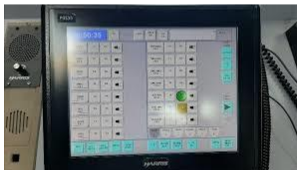
Gambar 3.1 Voice Switching & Control System (VSCS)
