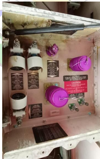
Gambar 4.34 Hydraulic pressurizaation ground service panel
