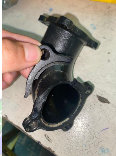
Gambar 4.19 Broken elbow pipe
