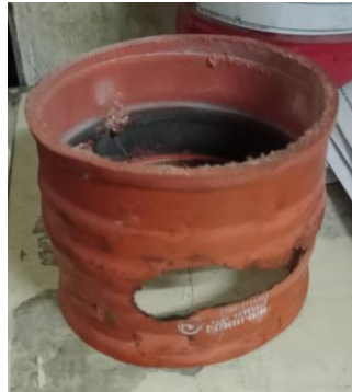
Gambar 4.14 Broken duct air surge
