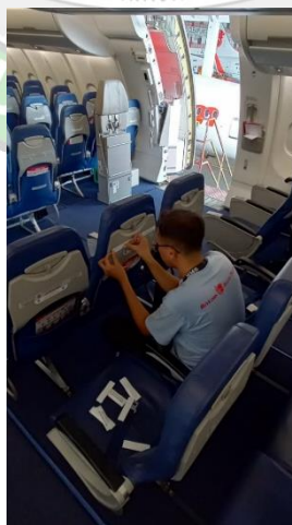
Gambar 4.31 Proses instalasi placards
