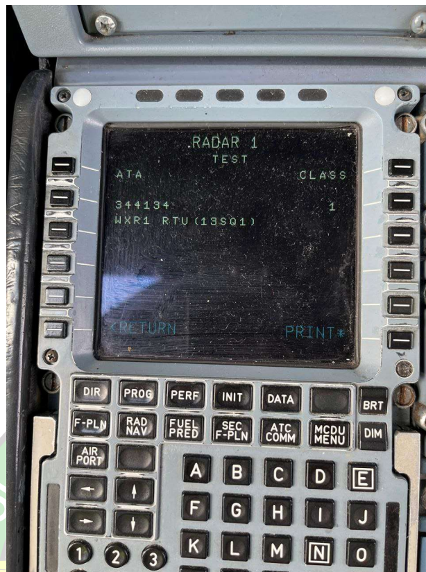
Gambar 4. 4 Weather Radar Transceiver found message (13SQ1)
