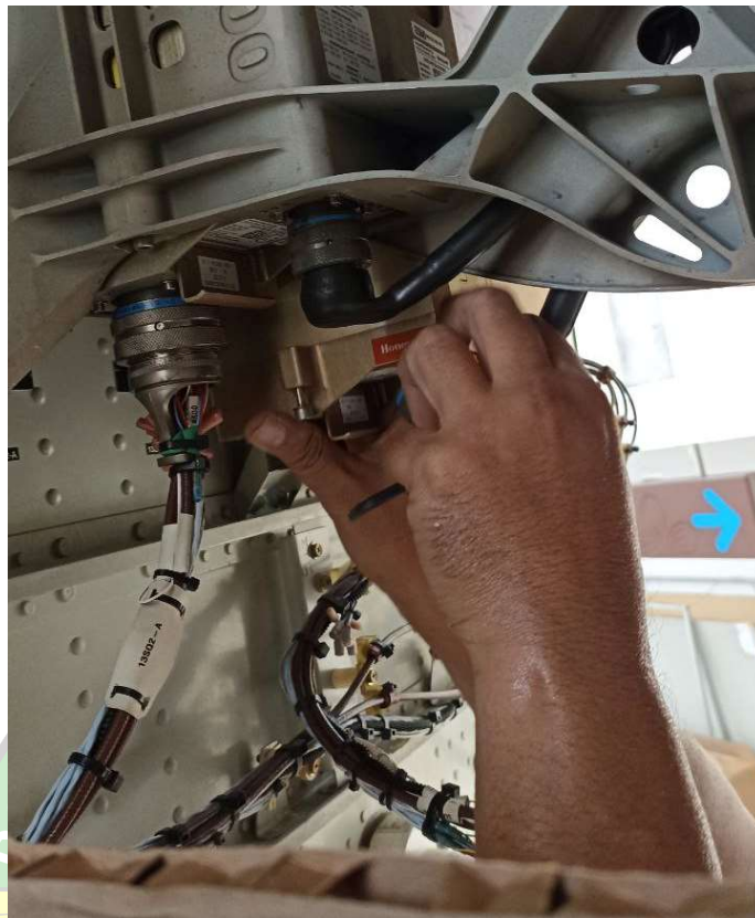
Gambar 4. 6 Pergantian Weather Radar Transceiver 1
