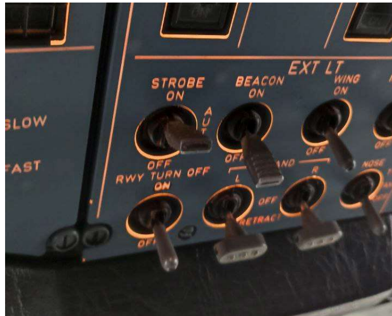
Gambar 4. 22 Operational Test Strobe Light
