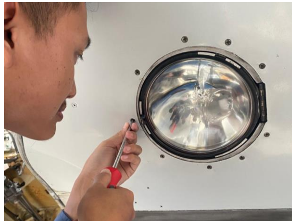
Gambar 4.24 Removal Connector Landing Light
