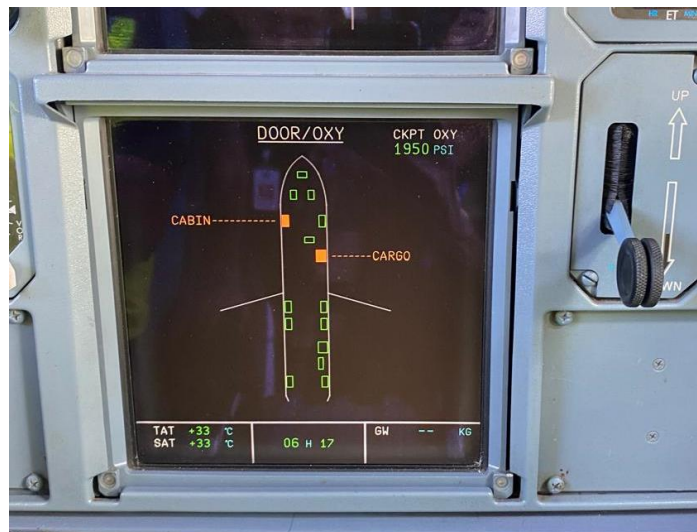
Gambar 4.33 Operational Test FWD cargo door proximity sensor
