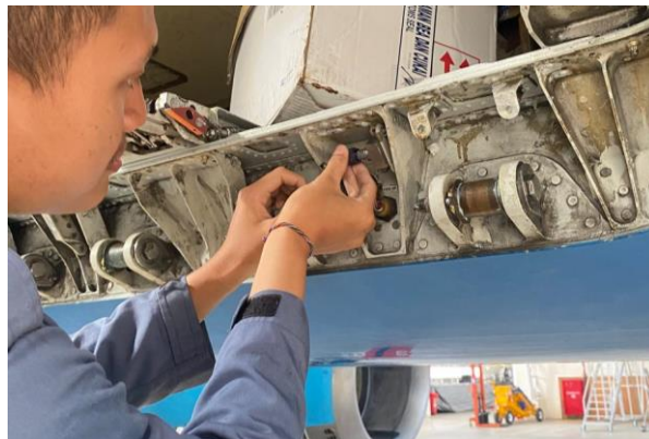
Gambar 4.38 Connector proximity sensor check
