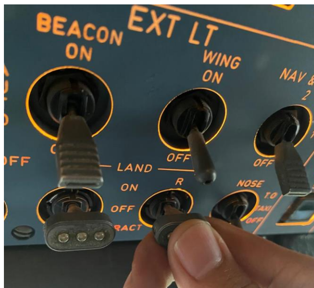
Gambar 4.17 Operational Test Landing Light
