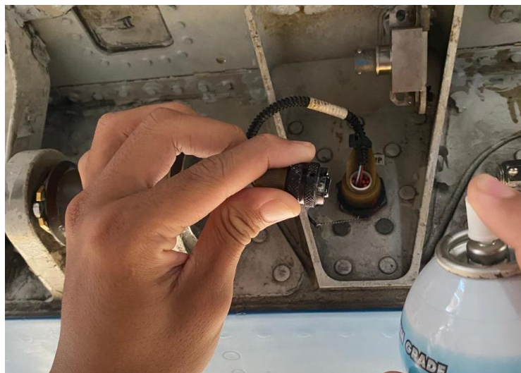
Gambar 4.39 Pembersihan connector proximity sensor
