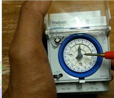
Gambar 4. 13 Setting Timer Theben SUL 181 d
