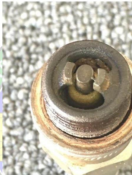
Gambar 4.3 Founded Ignitor Damaged and chapping
