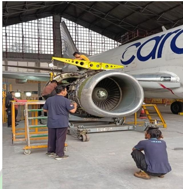
Gambar 4.1 Remove Engine with boot strap and hand crane
