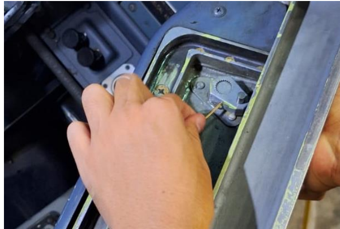
Gambar 4. 10 Emergency Exit Release Adjustment (sumber: dokumentasi pribadi)
