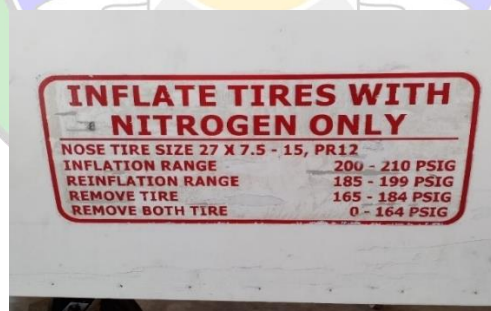
Gambar 3. 12 Nose Wheel Pound per square inch gauge. (sumber: dokumentasi pribadi)
