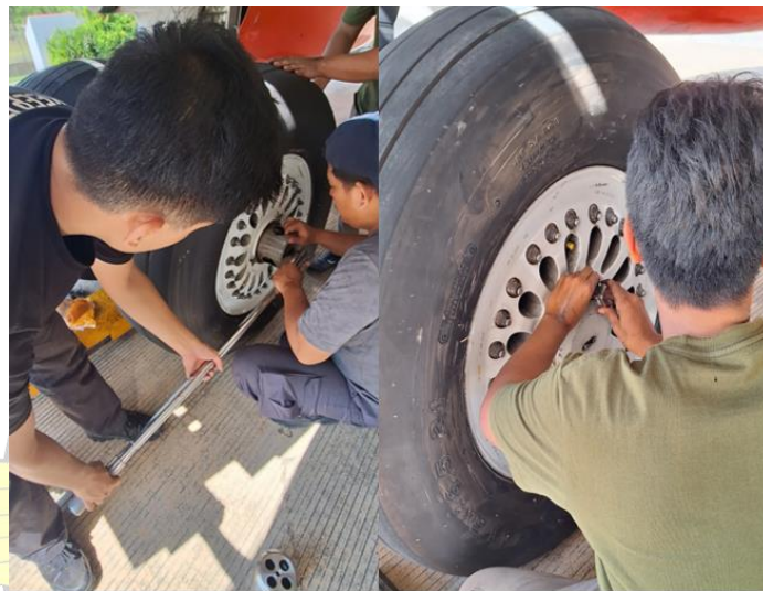
Gambar 4. 15 Servicing replacement wheel (sumber: dokumentasi pribadi)
