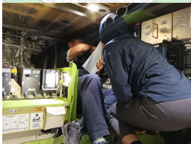
Gambar 4. 22 Proses Replacement Remote Electronics Units
