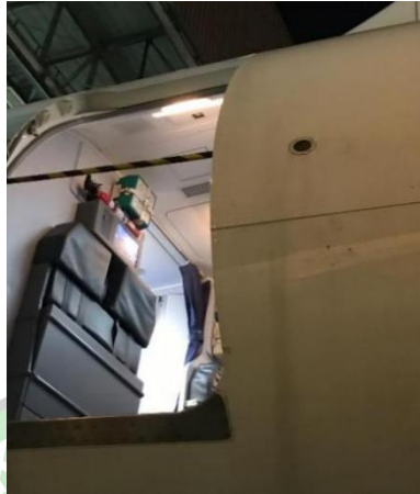
Gambar 4. 3 Aft Emergency Service Light Not Illuminate (Sumber: dokumen pribadi)
