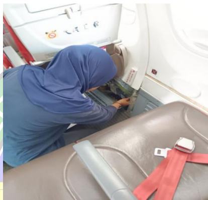
Gambar 4. 4 Open Access Panel Battery Pack (Sumber: Dokumen Pribadi)
