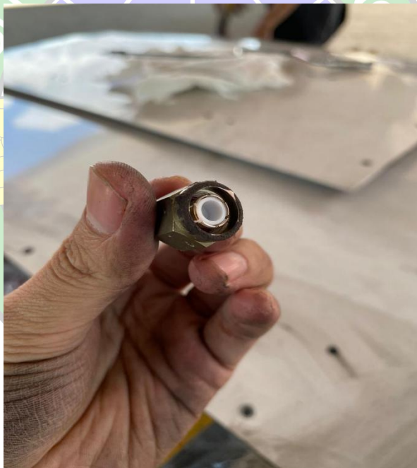
Gambar 4. 16 Connector Marker Beacon broken
