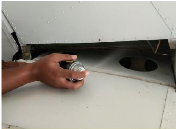
Gambar 4. 8 Servicing Flight Control Cable
