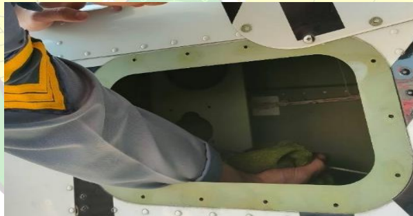
Gambar 4. 7 Inspection Flight Control Cable
