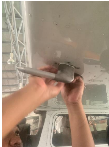
Gambar 4. 2 Disassembly pitot tube
