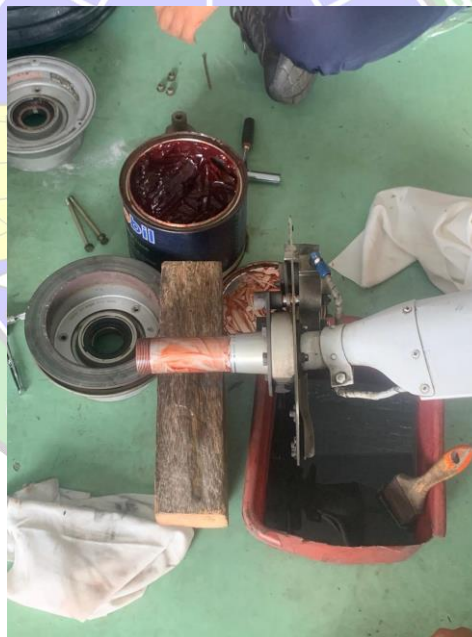
Gambar 4. 11 Reassembly wheel cesna 172S
