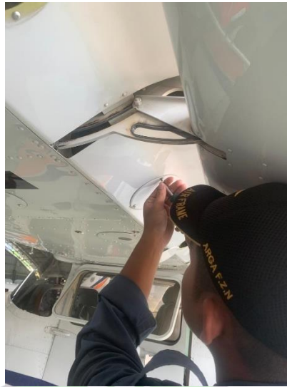
Gambar 4. 6 Fungsional Test Air Speed Indicator
