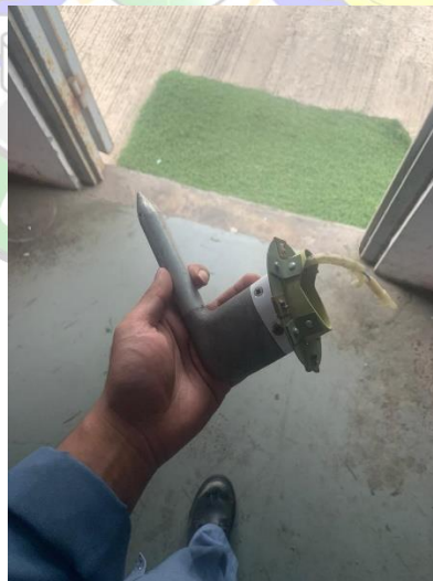
Gambar 4. 3 inspection pitot tube
