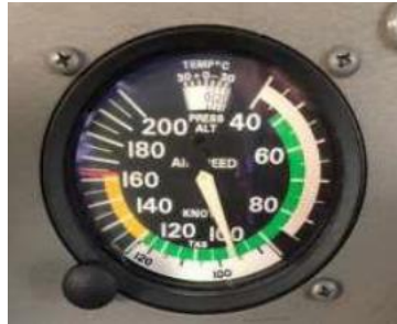
Gambar 4. 5 Fungsional Test Air Speed Indicator
