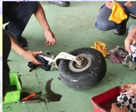
Gambar 4.4 servicing shock strut
