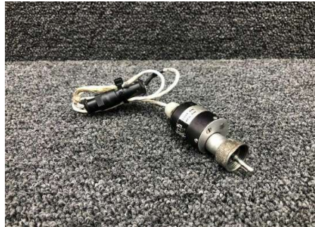
Gambar 4.9 Synchronize Magnetic Tachometer Sensor
