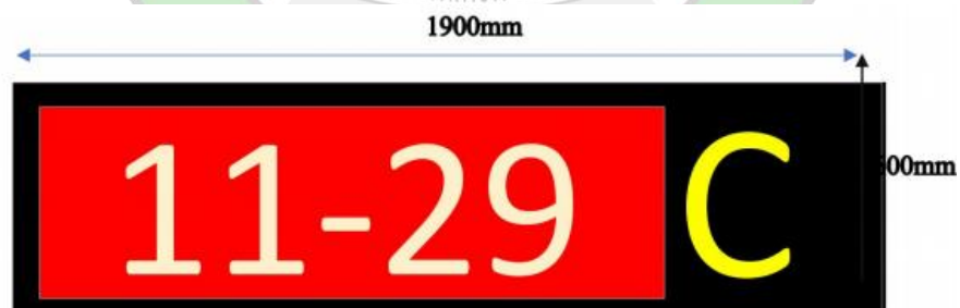
Gambar 4. 5 Fisik Runway Designation Sign C
