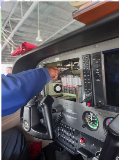
Gambar 4. 5 Install Standby Battery
