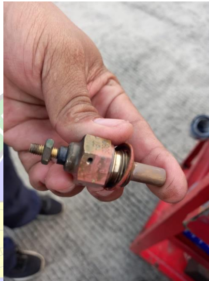
Gambar 4. 14 Inspection Oil Temperature
