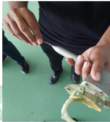
Gambar 4. 9 Inspection pitot tube
