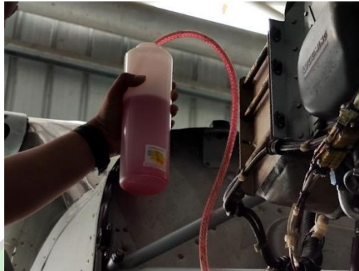
Gambar 4. 21 Proses shock strut servicing setelah proses re-assembly selesai
