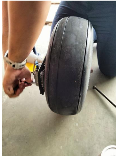
Gambar 4. 19 Disassembly left main wheel PK-BYS
