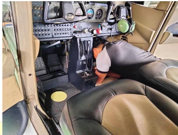
Gambar 4. 16 Installation fuel shutoff valve control cable sesuai AMMCessna 172S Skyhawk.
