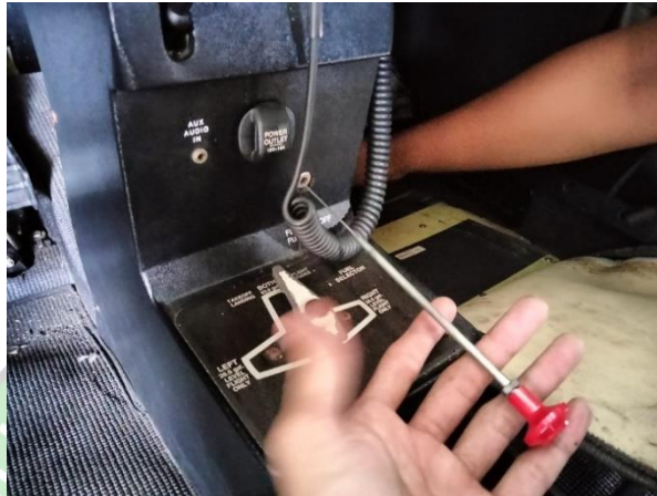
Gambar 4. 3 Shutoff Valve Cable putus
