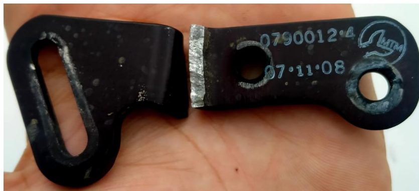
Gambar 4. 17 Clevis Bracket broken
