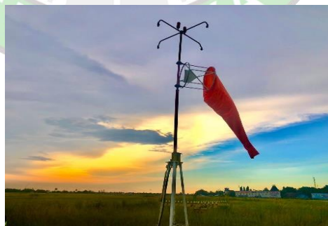
Gambar 2. 19 Wind Direction Indicator
