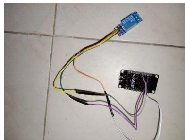
Gambar 4. 23 NodeMCU ESP8266~Modul Relay
