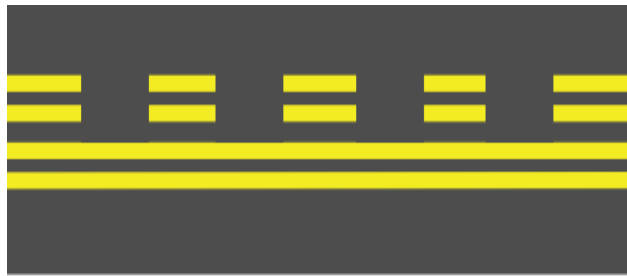
Gambar 3. 6 Runway Holding Position Signs
