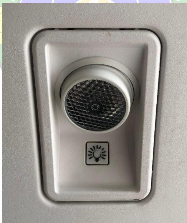
Gambar 3.7 pushbutton switch light reading door 1 R/H
