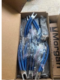
Gambar 4. 7 Perggantian Carbo Brush baru
