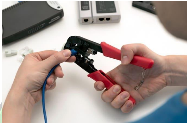
Gambar 3.9 1 Teknik Crimping Sumber : https://it.telkomuniversity.ac.id/
