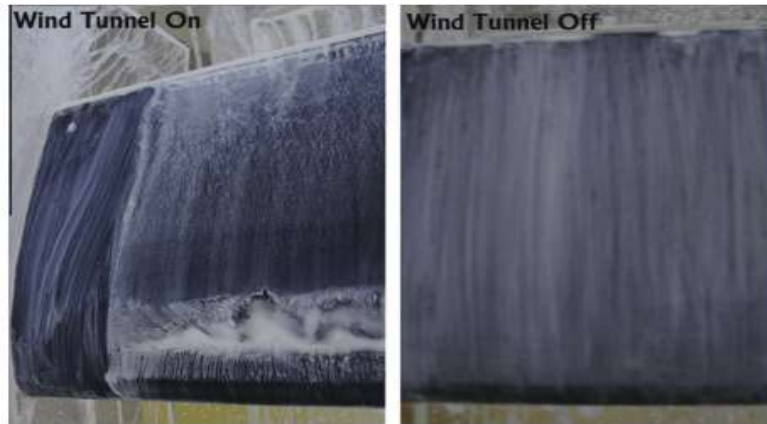
Gambar 2.18 Contoh Ekperimen Oil Flow Visualization over NACA 2415 (Genç,2011)
