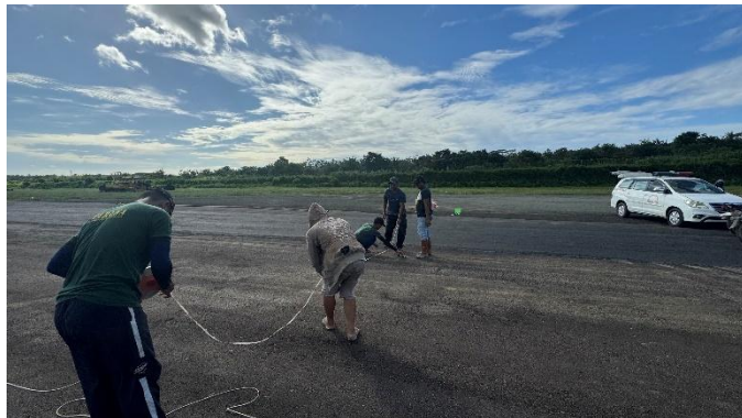
Gambar 4.60 Pengukuran Dimensi Marka Runway Designator
