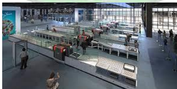
Gambar 3. 2 ATRS (Automatic Tray Return System)
