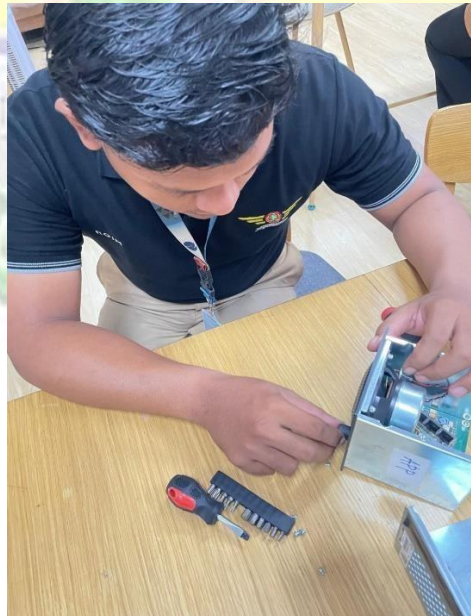
Gambar 4. 4 Perbaikan knop Potensiometer Speaker
