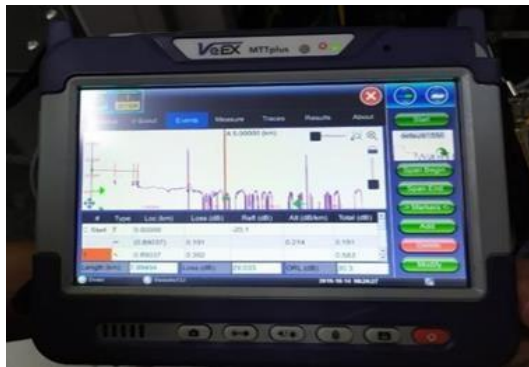
Gambar 3.12 Optical Time Domain Reflector Sumber : Unit Sistem Recording, Switching & Jaringan
