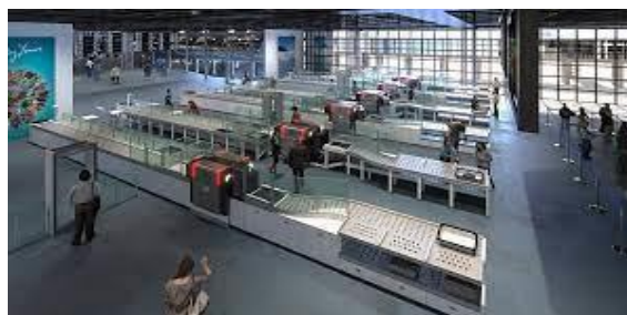
Gambar 3. 2 ATRS (Automatic Tray Return System)
