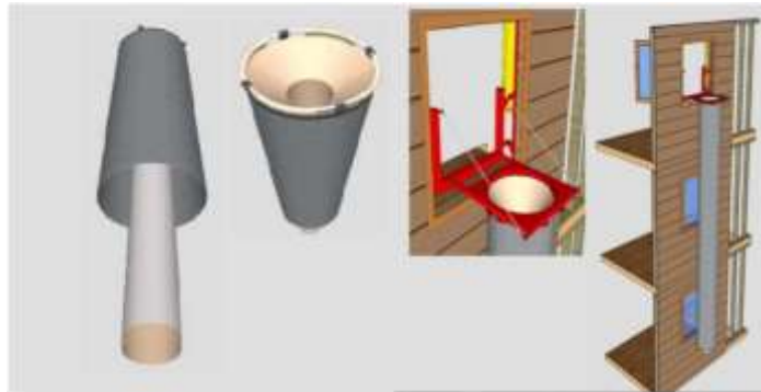
Gambar 4.4.2. Escape Chute System
